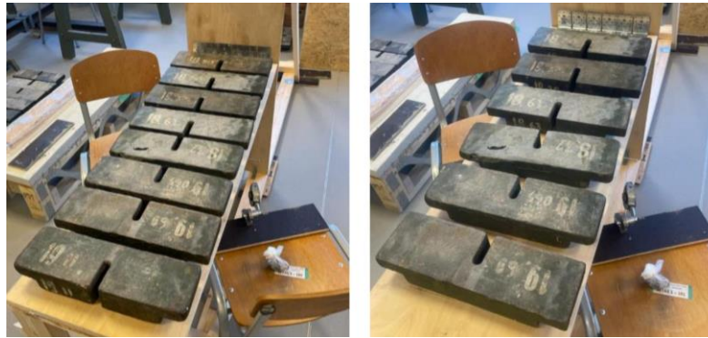
Figure 4. The placement of the steel pieces during loading with 8 pieces (left) corresponding to 151.8 kg, and with 6 pieces (right) corresponding to 113.9 kg.
