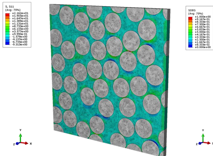
Figure 1: Normal stress distribution in the micro model.
