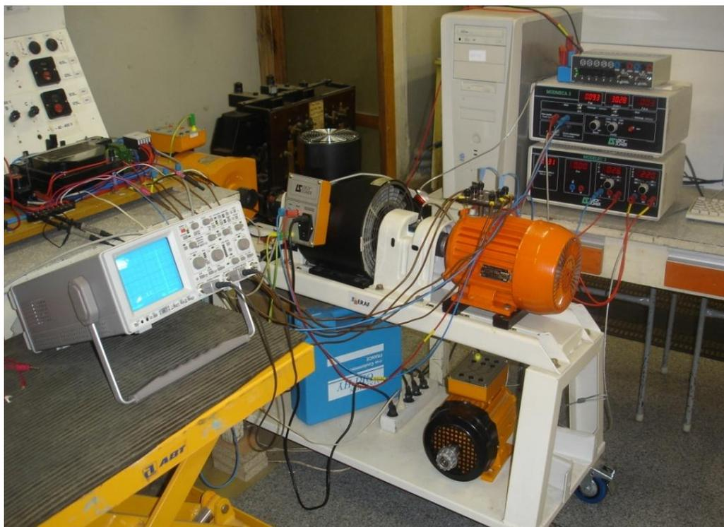
*Fig.4.2. Facilities for induction motor parameters definition*
