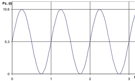
Fig.6 Pulsing side force loading( $P_z = 0 \dots 10,6$  tons).
