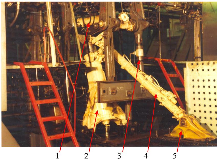
Fig.5 General view of loading gear test bench. 1 - truck; 2 - shock-absorber; 3 – loading system hydraulic cylinder; 4 - stay-hoist; 5 – bracket
