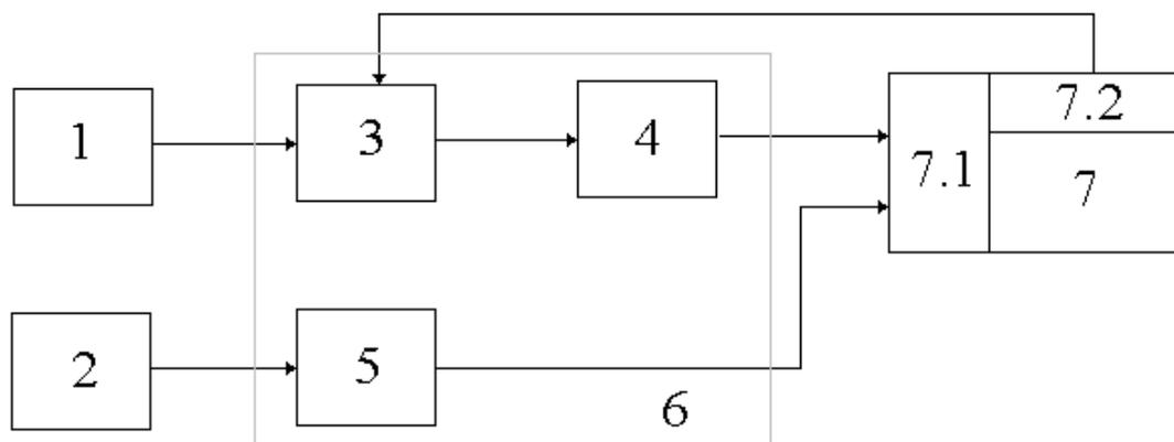
Fig 1. Functional diagram of modernized AE signal measuring complex on the basis of AΦ-15 instrument. 1 - AΦ-15, 2 - load sensor, 3 – controlled pulse counter-divider, 4 – buffer stage, 5 – matching amplifier, 6 - matching device, 7 - personal computer, 7.1. ADC Lcard L-783, 7.2 - DAC Lcard L-783.
