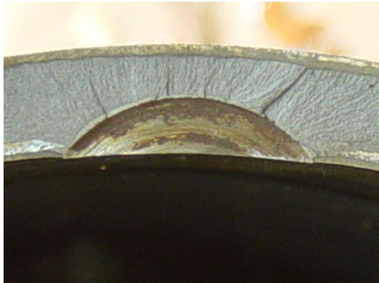
Fig.13 Saw cut concentrator (obtained after the destruction)
