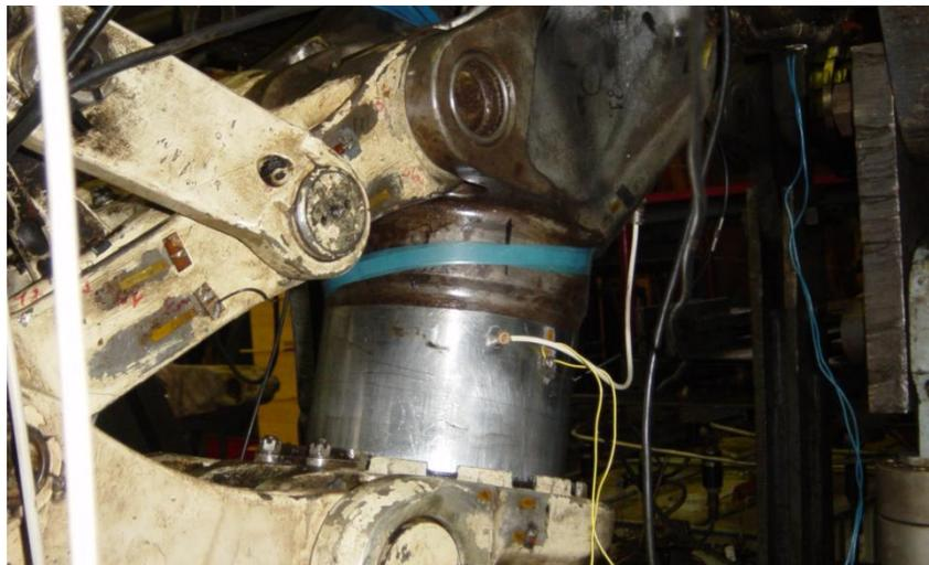
Fig 14. Placing piezoelectric transducer and strain gauge on shock-absorber rod mirror.
