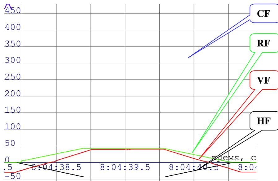
Fig.8 Cyclogram of load application to propeller pitch control arm of EH-101 helicopter.
