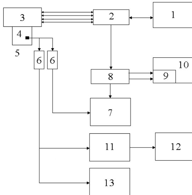
Fig.2. Diagram of AE measuring equipment connection. 1 - Control system computer, 2- Control system, 3- Hydraulic cylinder for setting loads, 4 – Test object, 5- AE sensor, 6 – Preamplifier (PA), 7 - AΦ-15 instrument, 8 – Matching device, 9 - AIQI Lcard L-783, 10 – AE registering computer, 11 - P-DAQ/T-DAQ measuring system, 12 -notebook, 13 - PAC 3000/3004 measuring system.
