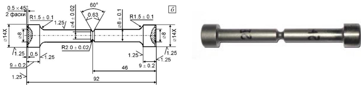
Fig.9 Geometry and appearance of specimens tested
