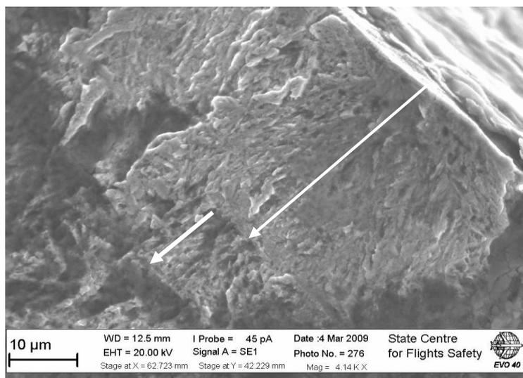
Fig.15. Fragments of fracture at the initial stage of landing gear support destruction
