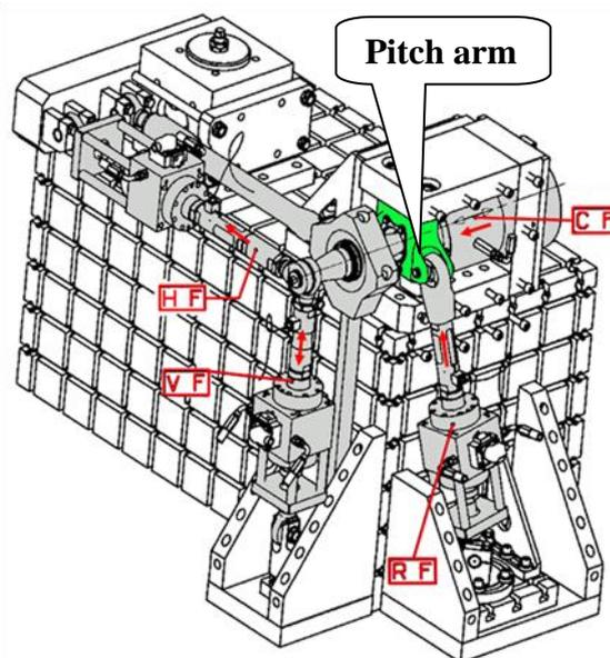
Fig.7 Diagram of a bench for conducting fatigue tests of propeller pitch control arm of EH-101 helicopter.
