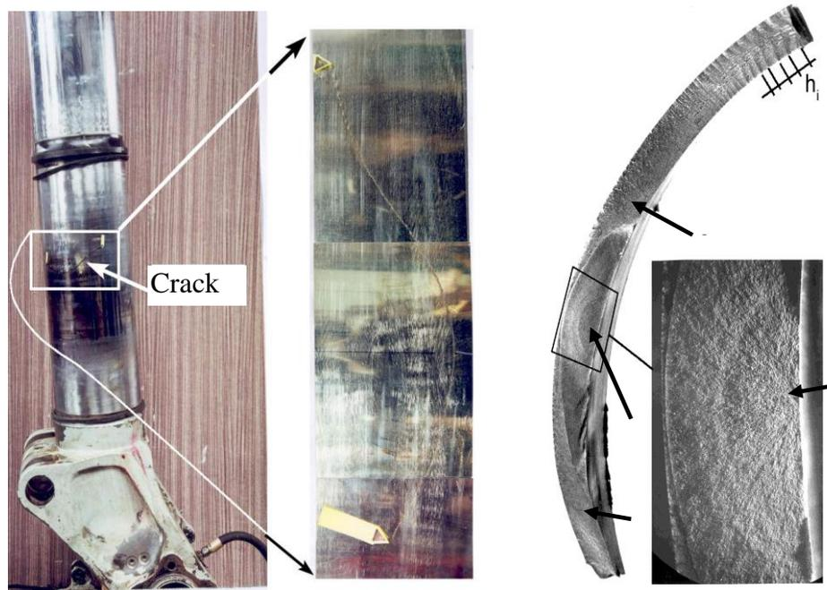
Fig.12 Shock-absorber rod crack
