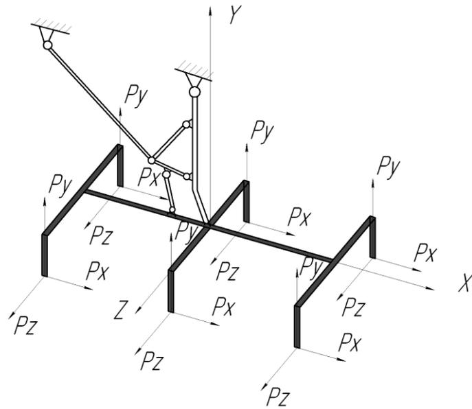
Fig.4. Diagram of load action upon landing gear principal support
