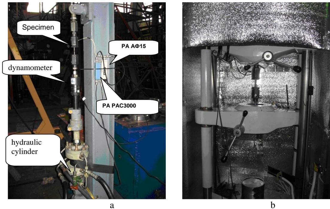
Fig.3. Titanium specimens testing unit (a), WPM testing machine (b)
