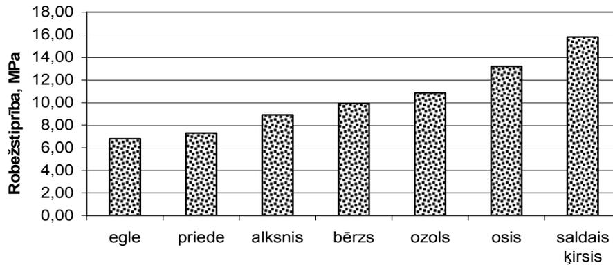
Fig. 9. Parameters of ultimate detrusion strength of wild cherry wood and other species [8] in tangential direction
