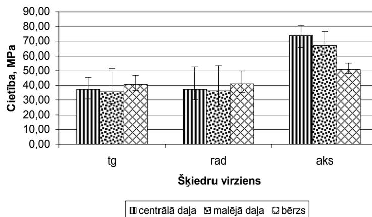
Fig. 10. Parameters of wild cherry and birch wood hardness in the main transverse anisotropy directions in wood
