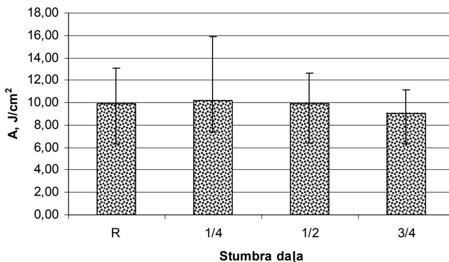
Fig. 11. Parameters of wild cherry wood resistance to shock at different stem heights
