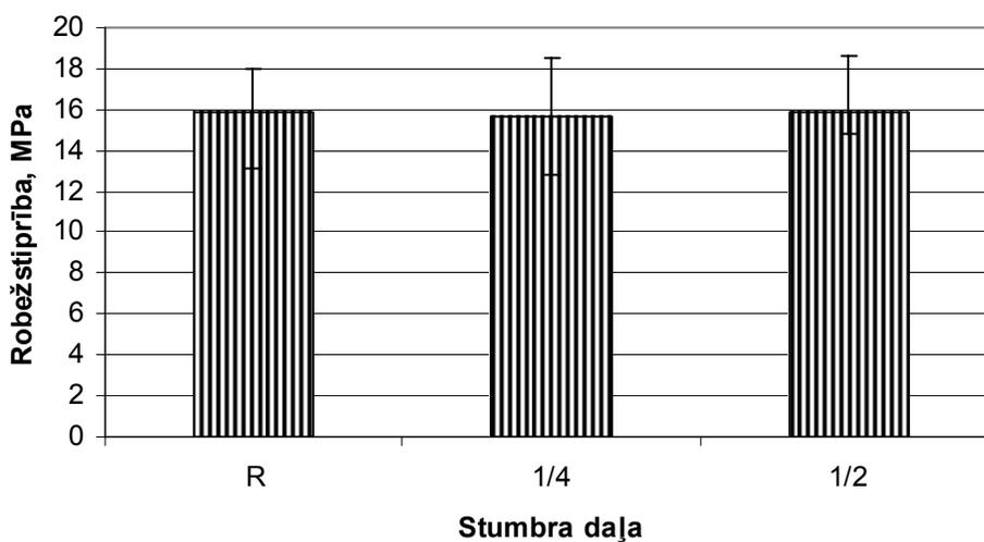
Fig. 8. Ultimate detrusion strength of wild cherry wood in tangential direction
