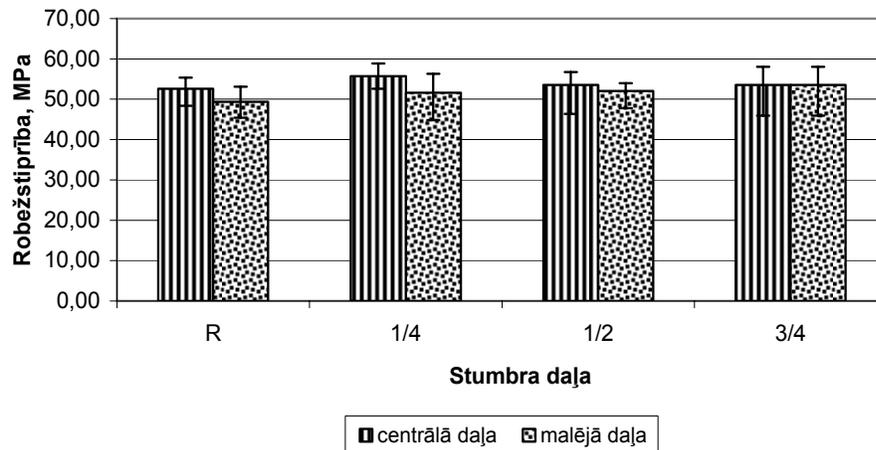
Fig 4. Ultimate compression strength of wild cherry wood in direction of fibres along the stem
