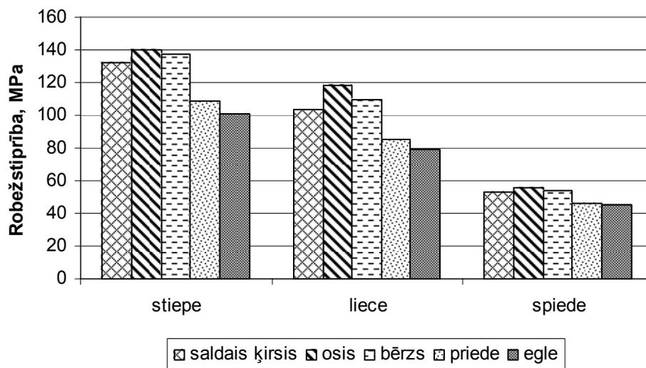
Fig. 6. Comparison of ultimate tensile, bending and compression strength of different tree species
