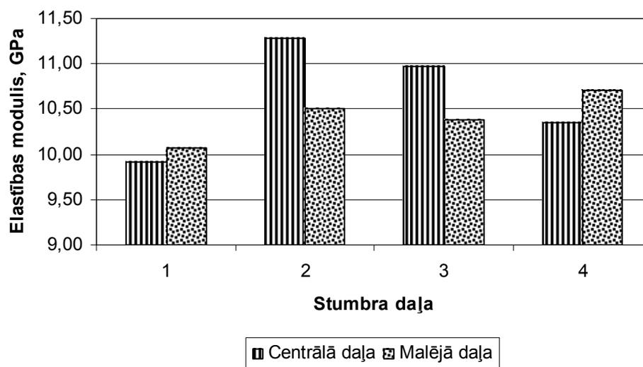
Fig. 7. Modulus of elasticity in bending of wild cherry wood at different stem heights
