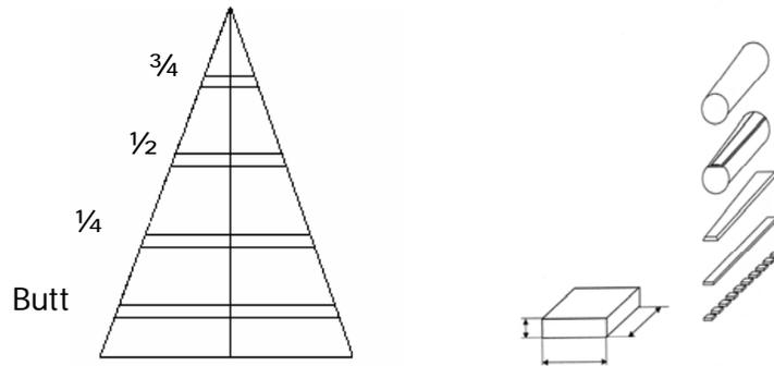
Fig. 1. Schematic location of samples in the stem
