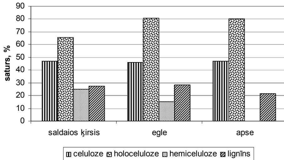
Fig. 14. Content of main wood components (cellulose, hemicellulose, holocellulose and lignin) for different tree species (%)
