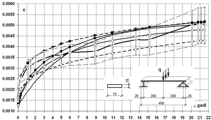
Fig 4.2. Loading scheme, cross-section and creep curves of particleboard plate, if load  $q=2.562$  kN-m. Patterns applied in graphic:
