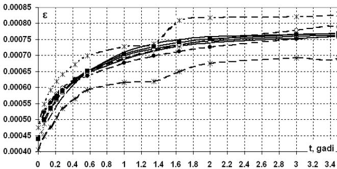
Fig 4.5. Creep curves of composite wood I-beam-2. Decoding of patterns see in fig 4.2. Loading scheme, cross-section and value of applied load are analogous to those show in the fig 4.4.
