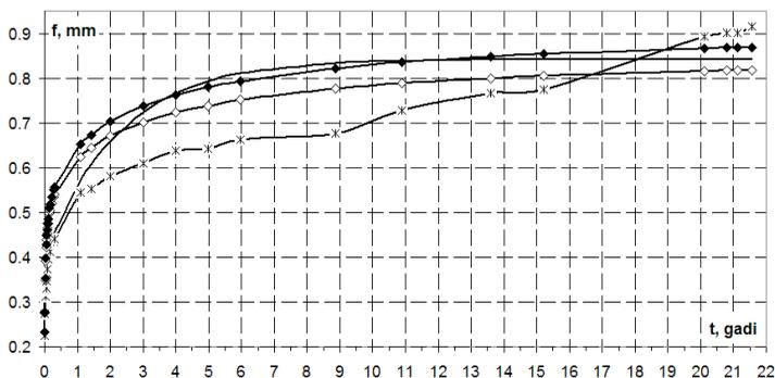
Fig 4.6. Creep curves of particleboard plate subjected to bending calculated as for composite material using the rheological properties of components. Patterns applied in graphic:
