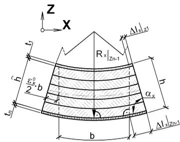
$$R_x|_{z_{n-1}} = \frac{\bar{h} \cdot \left( \frac{b}{2} + \Delta l_x|_{z_{n-1}} \right)}{\Delta l_x|_{z_{n-1}} - \Delta l_x|_{z_1}}, \text{ where} \quad (2.2)$$
