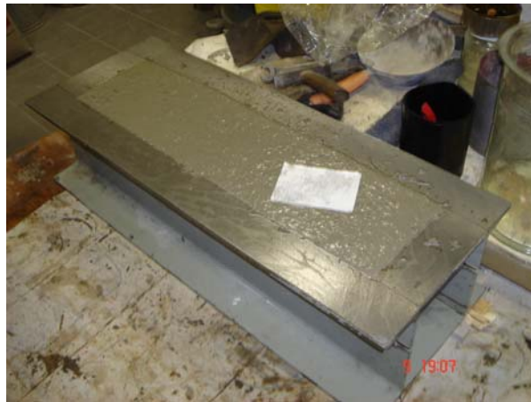
Fig.5.10. FRC beam sample casted in a steel mould
