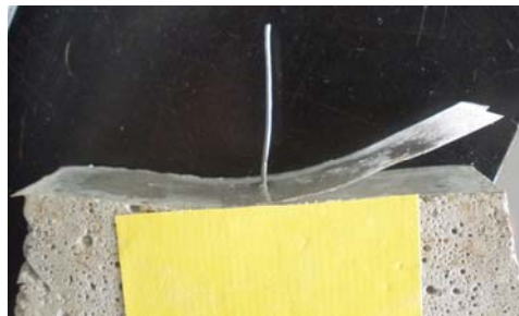
Fig.3.16. Undulated form fiber after complete pull-out
