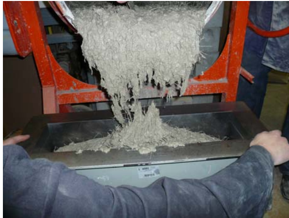
Fig.5.9. Filling of the mould with FRC mix with high fiber weight fraction
