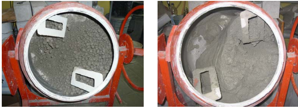
Fig.3.2. Mixing of concrete in a conventional concrete mixer
