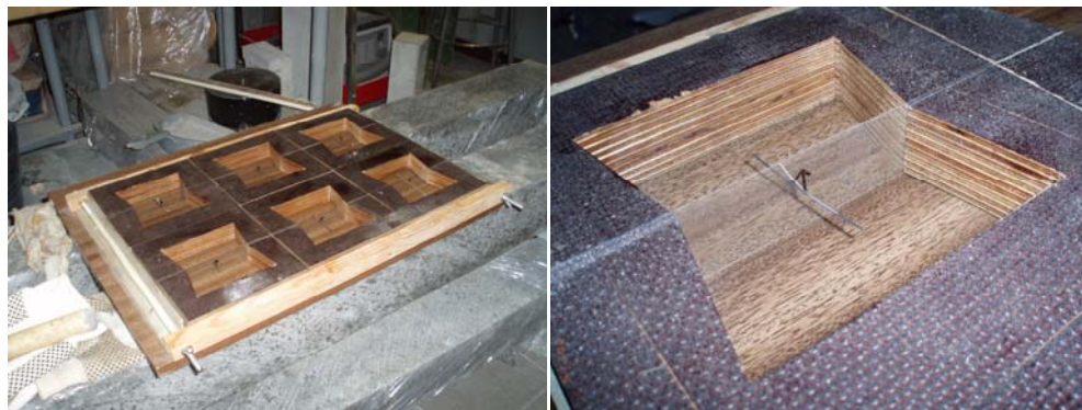
Fig.3.3. Plywood moulds before filling of concrete and a close-up showing plastic insert film with steel fiber
