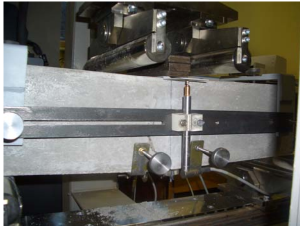
Fig.5.11. Displacement transducers attached on a FRC beam
