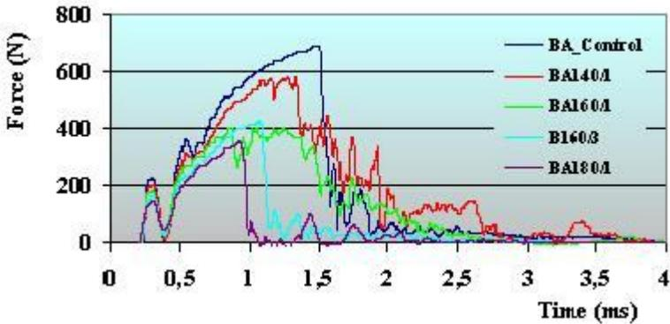
**Figure 6.a** Effect of HTM on the dynamic impact bending rupture-time curves of untreated and HTM **grey alder wood**
