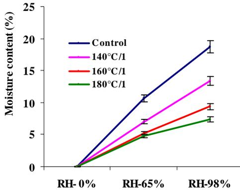
**Figure 4.c** Equilibrium moisture content of untreated and HTM aspen wood under variable RH
