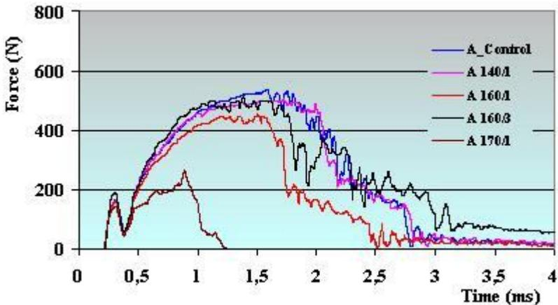
**Figure 6.b** Effect of HTM on dynamic impact bending rupture-time curves of untreated and HTM **aspen wood**
