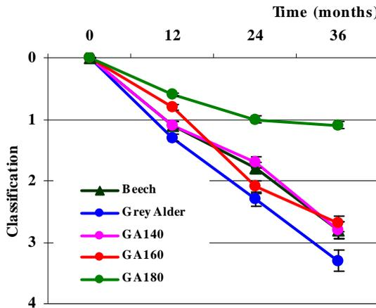
**Figure 9.** Average „pick-test” results of the untreated and HTM grey alder wood according to the EN 252 classification
