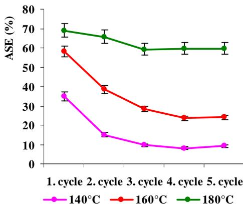
**Figure 5.c** Change of the total anti-swelling efficiency (ASE) of HTM **grey alder** wood during 5 cycles of water saturation and oven drying
