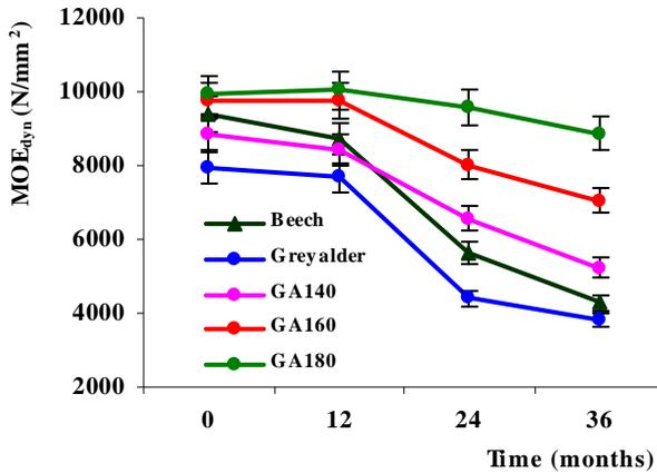
**Figure 8.** Average decrease in the dynamic modulus of elasticity for HTM grey alder wood until 3 years
