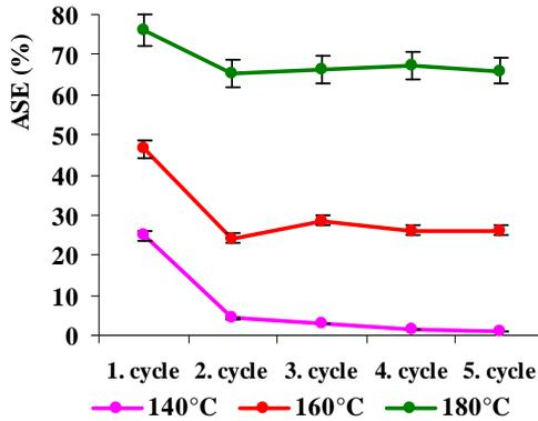
**Figure 5.a** Change of total anti-swelling efficiency (ASE) of HTM birch wood during 5 cycles of water saturation and oven drying
