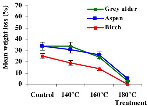
Figure 7.b Mean weight loss of untreated and HTM deciduous wood after 12 weeks inoculation to the **brown rot fungus *Poria placenta***
