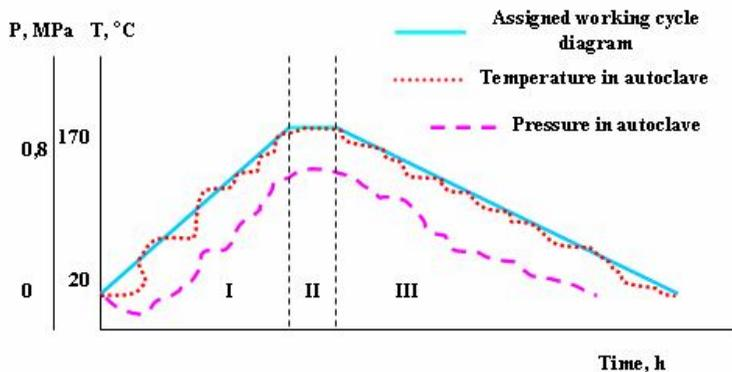
Figure 2. Diagram of the working cycle of thermal modification at 170 °C
