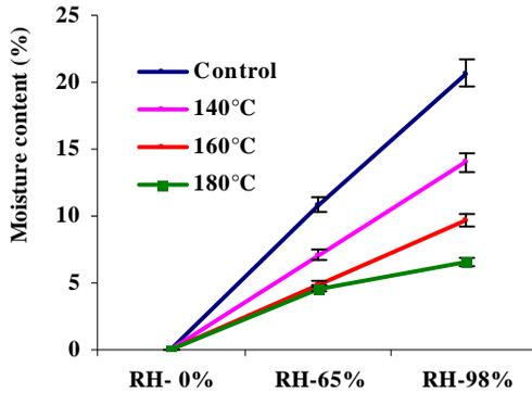
**Figure 4.b** Equilibrium moisture content of untreated and HTM birch wood under variable RH
