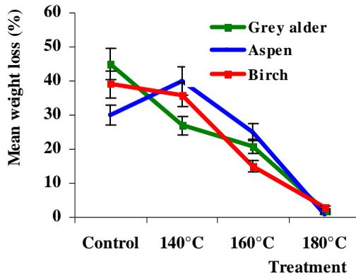
**Figure 7.c** Mean weight loss of untreated and HTM deciduous wood after 12 weeks inoculation to the **brown rot fungus** *Coniophora puteana*
