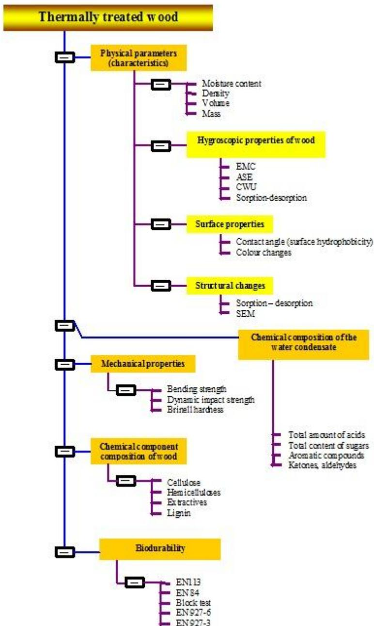
Figure 3. Course of the experiment and analysis methods applied
