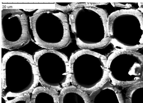
**Figure 12.** Libriform fibres after the 180°C treatment
