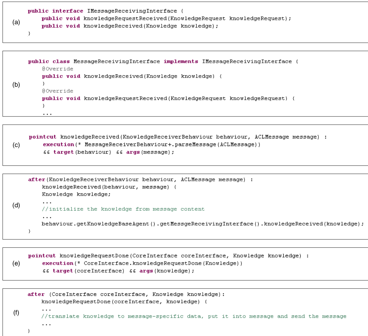
Fig. 7. Code samples for aspect interface ((a), (b), (c) and (d)) and aspect listener ((e) and (f)) of the messaging component
