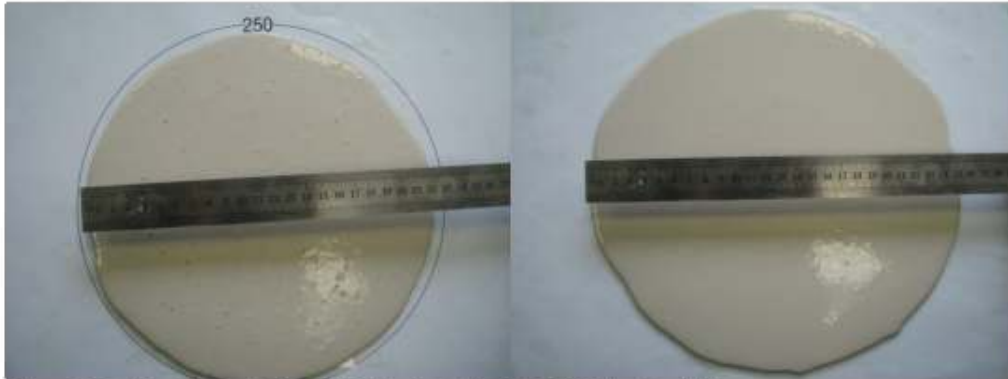
Figure 5: Cylinder flow test. Mix REF-1 (on the left), Mix CAV-1 (on the right).
