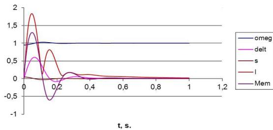
Fig. 2.8. Results of synchronization with frequency  $\omega = 0,95$ , moment, current, rotation frequency, shift angle in time
