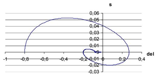
Fig. 2.5. Results of synchronization with mismatch angle  $\delta = -0,8 \text{ el.rad}$ , phase's trajectory.
