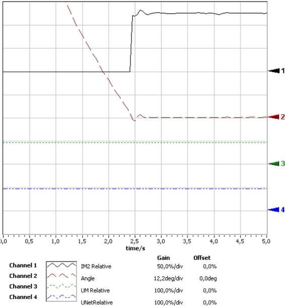
Fig.3.5. The results obtained at the moment of synchronization under condition– generator-double load.
