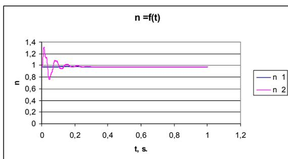
Fig. 2.13. Synchronization results of two generators – frequency by time:
