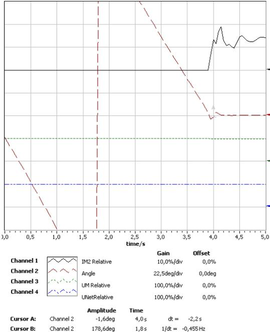
Fig.3.3. The results obtained at the moment of synchronization under condition– generator-network.
