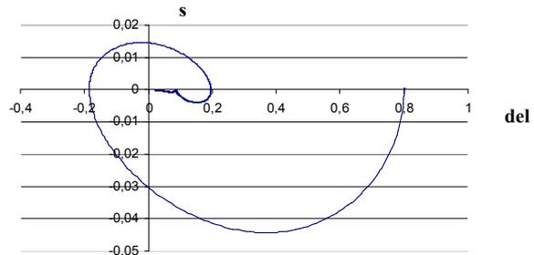
Fig. 2.3. Results of synchronization with mismatch angle  $\delta = +0,8 \text{ el.rad}$ , phase's trajectory.
