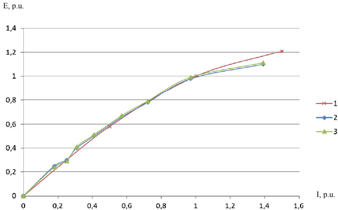
Fig.3.7. Regular(1) obtained by practical approach (3)and estimated (2) characteristics of idle run of the generator.
