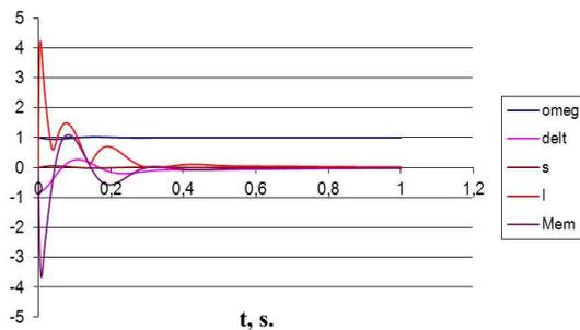
Fig. 2.4. Results of synchronization with mismatch angle  $\delta = -0,8 \text{ el.rad}$ , moment, current, rotation frequency, shiftangle in time.
