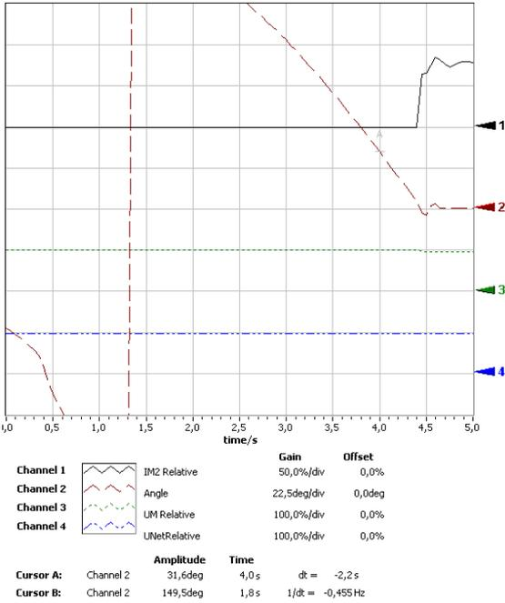
Fig.3.4. The results obtained at the moment of synchronization under condition– generator-load.
