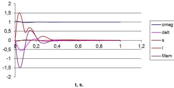
Fig. 2.6. Results of synchronization with frequency  $\omega = 1,05$ , moment, current, rotation frequency, shift angle in time.
