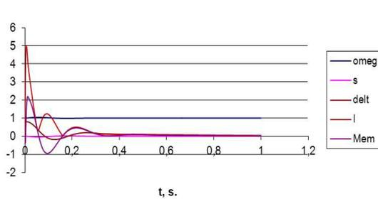
Fig. 2.2. Results of synchronization with mismatch angle  $\delta = +0,8 \text{ el.rad}$ , moment, current, rotation frequency, shift angle in time.
