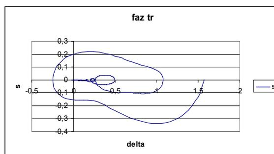
Fig. 2.14. Synchronization results of two generators – phase trajectory.
