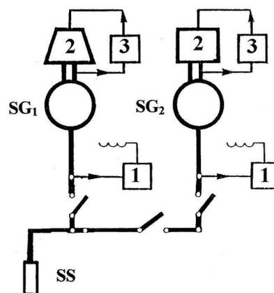
Fig. 2.10. Scheme of mathematical model. (1.- excitation; 2.- the engine; 3.- the engine control; SS - load).
