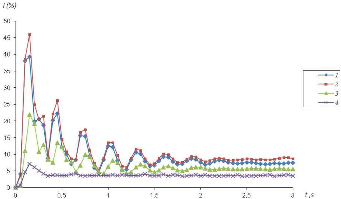
Fig.3.6. Results for cases of coming into a synchronous work are resulted at a deviation from synchronization conditions generator-network (no load)  $I=f(t)$ , ( $U_{net}=U_g$ ,  $\delta=0$ );
