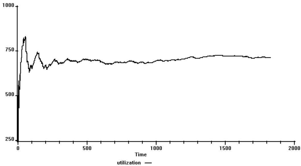
Figure 4.1:  $M/M/1$  system utilization,  $\lambda = 0.7, \mu = 1$
