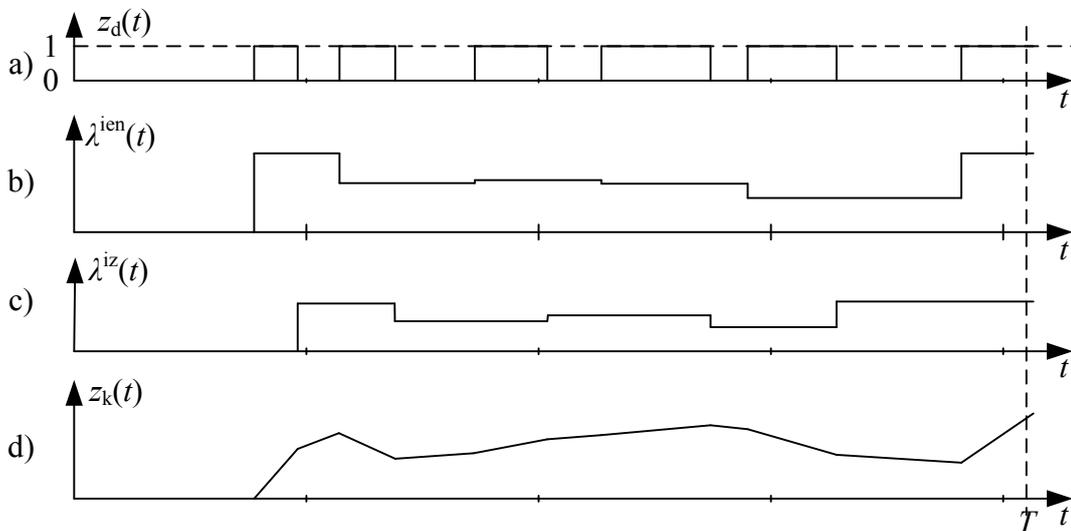
**Figure 5. a) the state trajectory of a discrete device, b) the incoming and c) the outgoing flow intensities and d) the state trajectory of a bunker**
