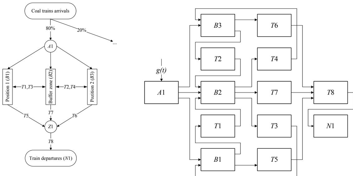
a) The process diagram of the first zone of the coal terminal
