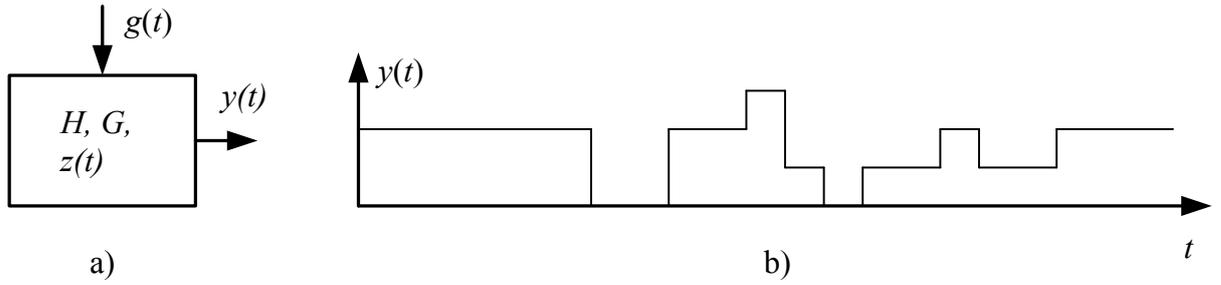
**Figure 4. The single-channel source: a) simple image, b) an example of an outgoing signal**
