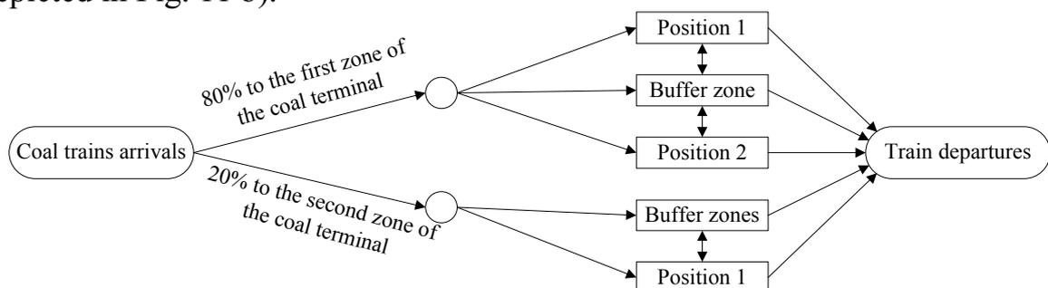
**Figure 10. The simplified structure of the coal terminal**
