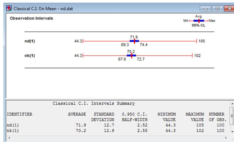
**Figure 13. The test of loading/unloading positions utilisation estimates obtained from discrete event and combined model with 95% confidence level**
