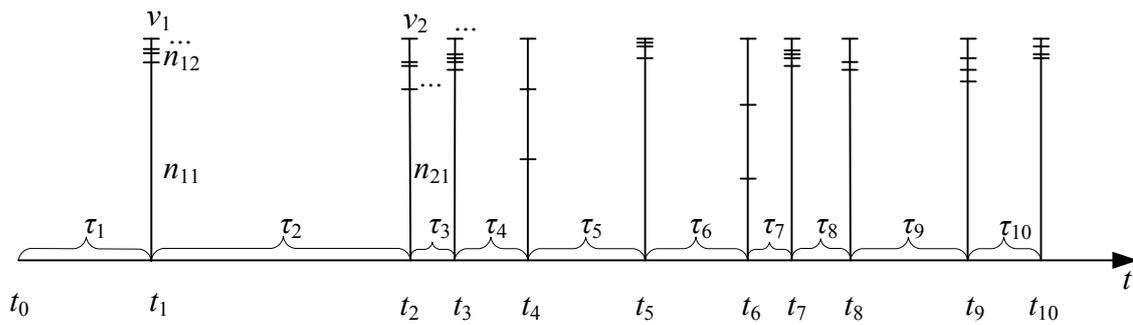
**Figure 2. An example of wagon flow time diagram**
