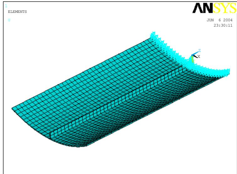
Figure 2. Finite-element model of the plate
