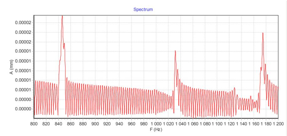
Figure 18. Frequency spectrum 800-1200 Hz of calculated process, 2000 steps
