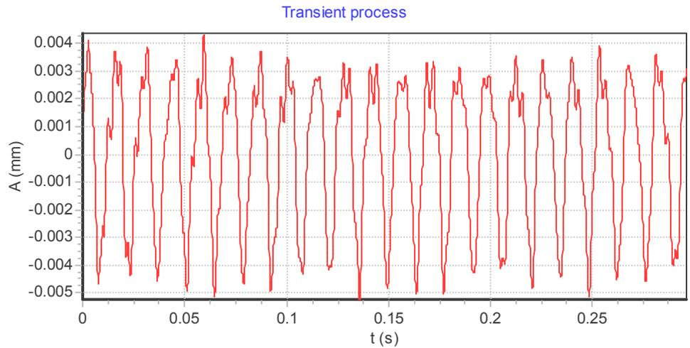
Figure 4. Calculation by ANSYS – displacement of the point №1978 at time along Y-axis (Fig.1.)
