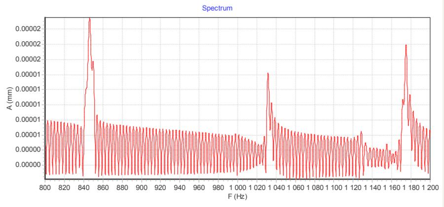
Figure 19. Frequency spectrum 800-1200 Hz of calculated process, 3000 steps
