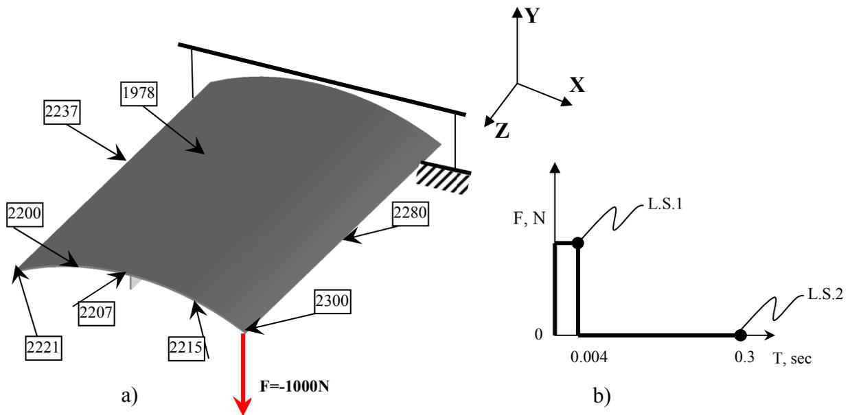
Figure 1. a) covering element – plate with checkpoints, (0.4x0.25x0.002 s-0.015),
