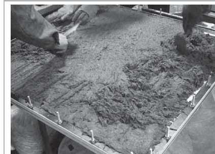
Figure 1. Short glass fiber concrete is evenly placed on the surface of rubber membrane (pneumatic mould).
