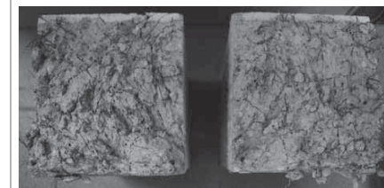
Figure 5. Both fracture surfaces for one prism. It is possible to see many fibers oriented close to parallel to crack surface. SFRHPC with Tabix 50 (50 mm long undulator round crosssection steel fibers), Dramix 30 (30 mm long ends hooked round crosssection steel fibers), Dramix 13 (13 mm long straight round crosssection steel fibers) and Dramix 6 (6 mm long straight round crosssection steel fibers) fibers cocktail.
