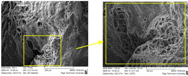
Fig. 5 PVA hydrogel SEM microphoto ( $C_{15}$ , PVS III,  $n_C = 3$ )
