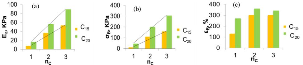
Fig. 22 Conditional tensile modulus  $E_a$  (a), tensile strength at break  $\sigma_B$  (b) and relative deformation at break  $\varepsilon_B$  (c) for PVA gels depending on  $n_c$
