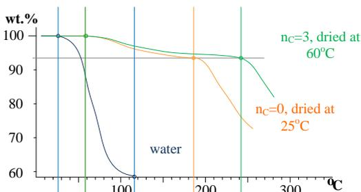
Fig. 11 TG thermogram  $C_{15}$ : unfrozen dried sample 25°C ( $n_c = 0$ ), 60°C dried PVA gel ( $n_c = 3$ ) and pure water
