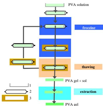
Fig. 1 Cryosynthesis process of PVA gel: 1 – aluminium mould, 2 – sealable plastic bag, 3 – foam capsule
