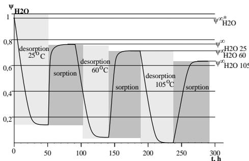
Fig. 14 Scheme of change of water content  $\psi_{H_2O}$  in desorption - sorption cycles
