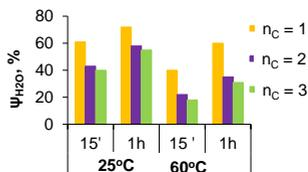
Fig. 17 Water content in gels after a sorption period (15' and 1h), depending on the drying temperature (25 and 60°C) and the number of f-t cycles
