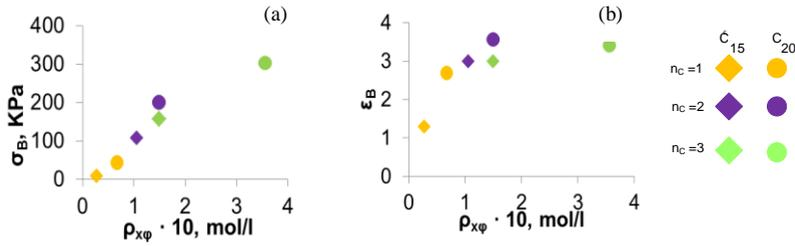
Fig. 24 Values of  $\sigma_B$  (a) and  $\varepsilon_B$  (b) depending on the crosslinking density  $\rho_{x\varphi}$
