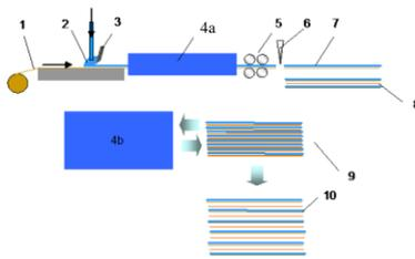
Fig. 27 Technological scheme of industrial-scale production of PVA cryo-hydrogel dressing: 1 - support layer 2 - dosing of PVA solution, 3 – equipment of squeegee-type PVA layer application and calibration, 4a, b - cryo-thermostat, 5 - pulling equipment, 6 - cutting machine, 7 - PVA solution sheet with support layer, 8 - dividing polymer film, 9 - sheet pack, 10 - PVA cryo-hydrogel dressing sheet
