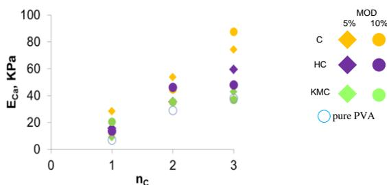
Fig. 25 Values of elastic modulus  $E_{ca}$  of PVA hydrogel - a polysaccharide composites depending on the number of f-t cycles
