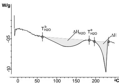
Fig. 10 DSC thermogram of  $C_{15}$  PVA unfrozen sample dried of 25°C ( $n_c = 0$ )
