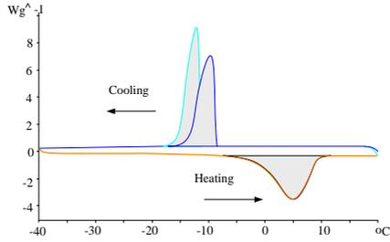
Fig. 3 DSC thermogram of freeze-thaw process of PVA aqueous solution ( $C_{15}$ )
