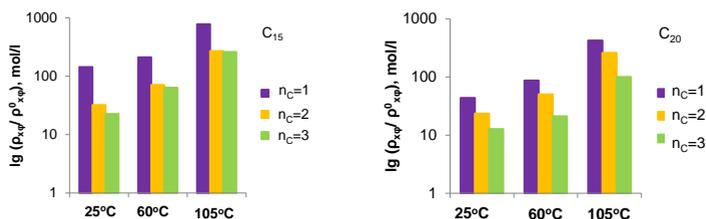
Fig. 18 The dependence of relative values crosslinking density  $\rho_{x\phi} / \rho_{x\phi}^0$  of gels on drying temperature and number of f-t cycles ( $\rho_{x\phi}^0$  – the initial value of the gel crosslinking density)
