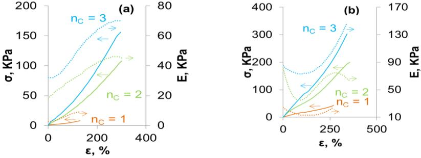
Fig. 21  $\sigma(\varepsilon)$  and  $E(\varepsilon)$  relationships in tensile mode of PVA hydrogel: C<sub>15</sub> (a) and C<sub>20</sub> (b)
