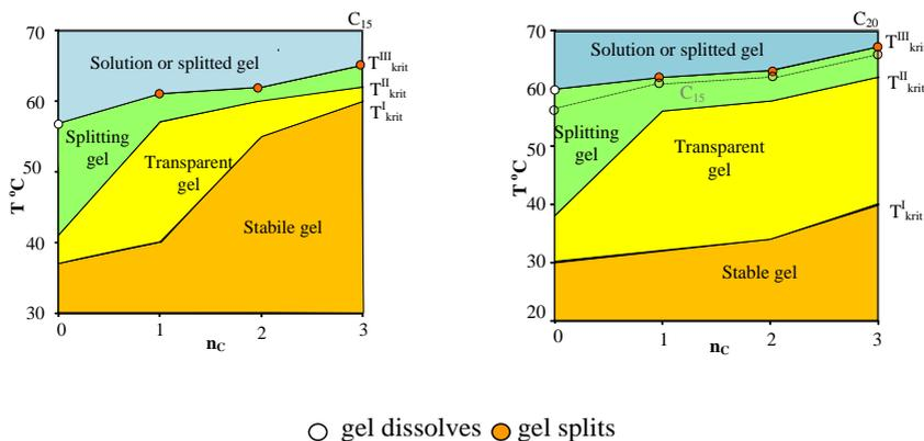
Fig. 7 The dependence of critical temperature from the number of f-t cycle
