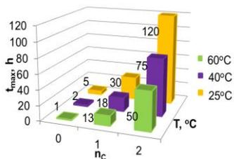
Fig. 8 dependence of  $t_{krit}$  on exposing temperature and number of f-t cycles ( $C_{15}$ )
