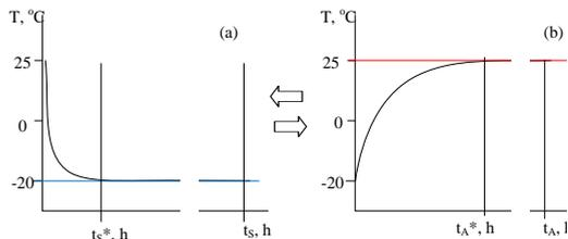
Fig. 2 Time-temperature regime scheme of freezing (a) - thawing (b) process.
