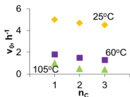
Fig. 16 The initial water sorption rate  $v_0$  of PVA gels dried at different temperatures and obtained with different number of f-t cycles
