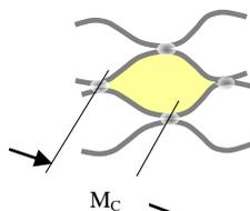
Fig. 19 Schematic representation of the "canal" in macromolecular structure of gel
