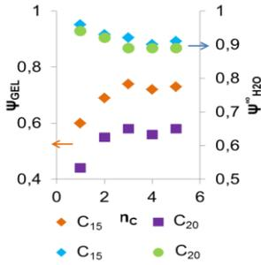
Fig.4. The dependence of hydrogel characteristics  $\psi_{GEL}$  and  $\psi_{H_2O}^\infty$  on the number of f-t cycles  $n_C$
