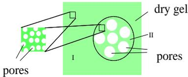
Fig. 6 Schematic structure of porous of dried gel
