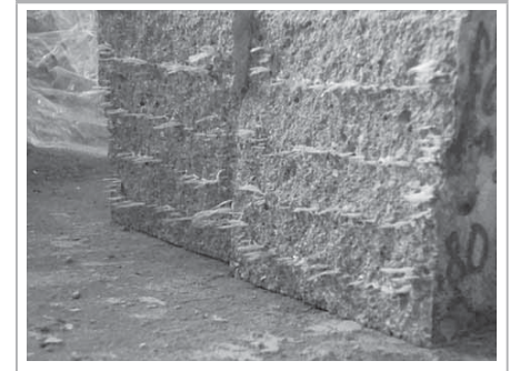
Figure 7. Concrete prisms tested by bending.
