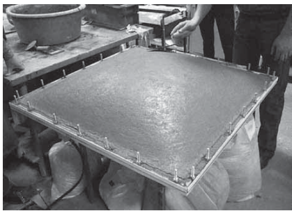
Figure 2. Rubber mould is inflated by air till its final shell shape size was reached.
