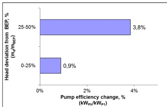
Fig. 2.5 Centrifugal pump efficiency reduction at different changes of head value from the nominal head
