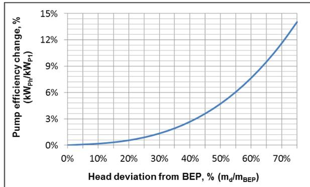
Fig. 2.4 Centrifugal pump efficiency reduction at different changes of head value from the nominal head
