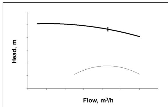
Fig. 1.3 Best efficiency point (BEP) of centrifugal pump
