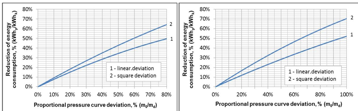
Fig. 2.2 Reduction of electrical energy consumption by pumps
