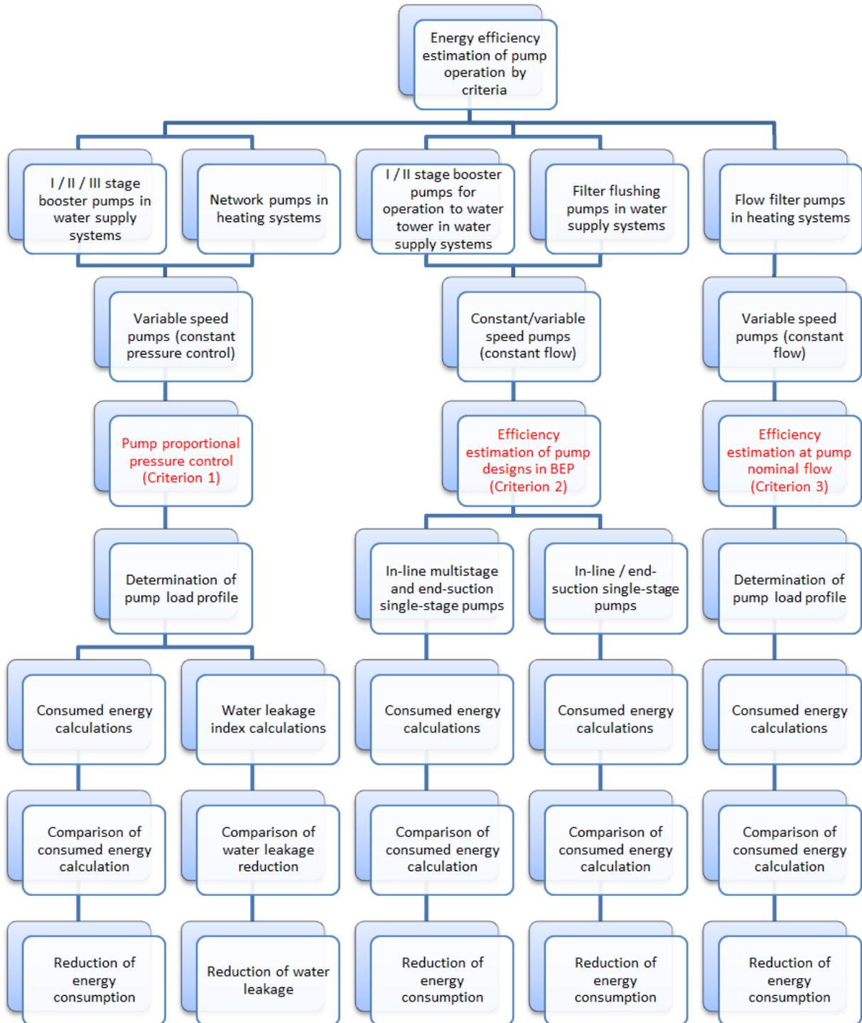
Fig. 2.1 Algorithm of energy efficiency evaluation of centrifugal pumps operation (by criteria)
