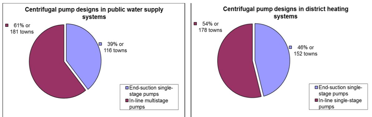
Fig. 1.4 Usage of pump designs in public water supply and district heating systems in Latvian towns (up to 10,000 inhabitants)
