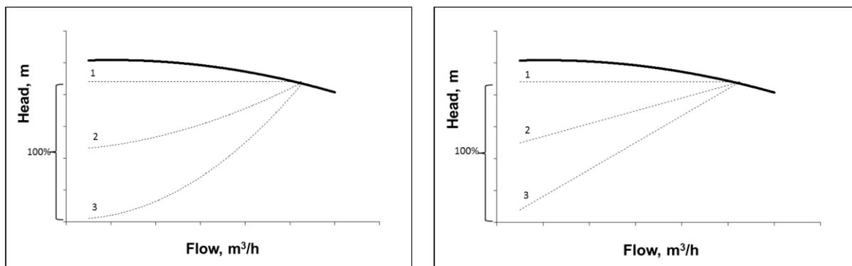
Fig. 1.1 Variable speed pump control modes
