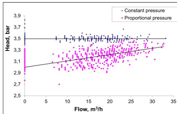
Fig. 3.1 Pump head and flow values of second stage booster system
