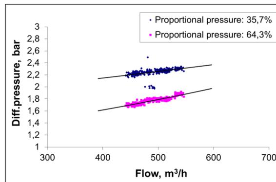
Fig. 3.2 Pump differential pressure and flow values of main network pumps Proportional pressure control modes with different control curve deviations (35.7% to 64.3%)
