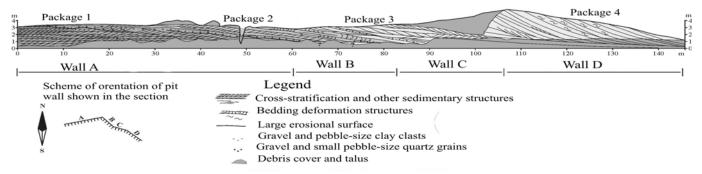
Fig. 6. Composition and structure of quartz sands in Bale sand pit sector 2 [6].
