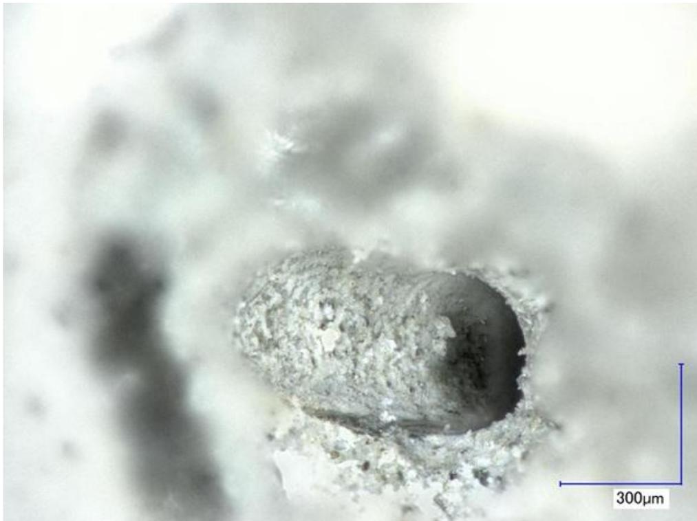
Fig.1.9. Canal surface left by the orientated fiber at an angle of 80°
