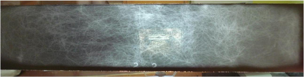
Fig.1.12. X-ray image of fiberconcrete K2 (screened from the top)
