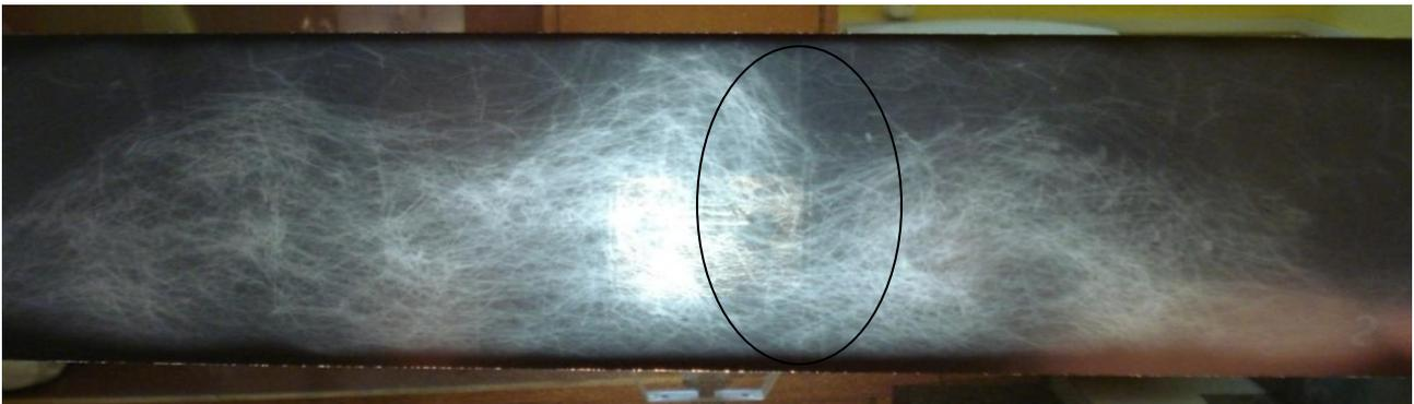
Fig.1.13. X-ray image of fiberconcrete K2 (screened at the side)
