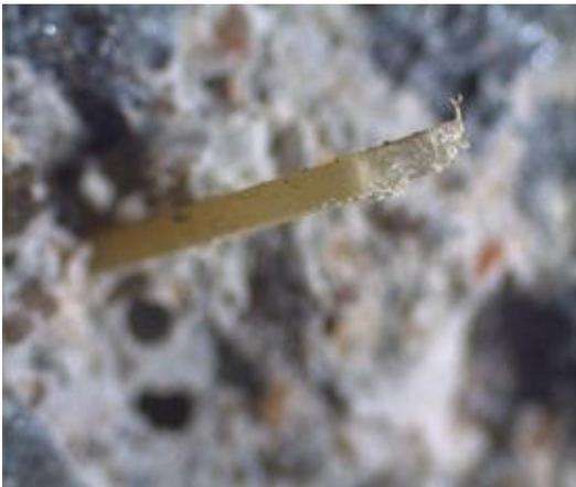
Fig.1.1. Polymeric synthetic fiber at an angle of  $90^\circ$  pull-out of the concrete (under microscope)
