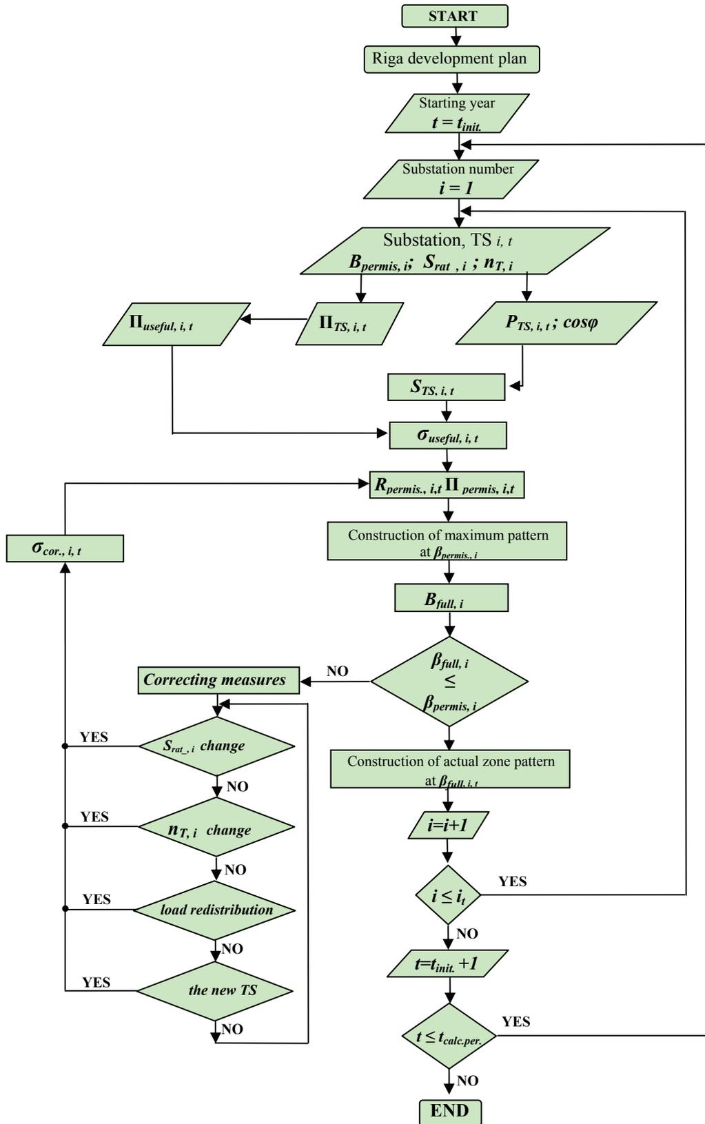
Fig. 3.1. The load density correction algorithm in development projects
