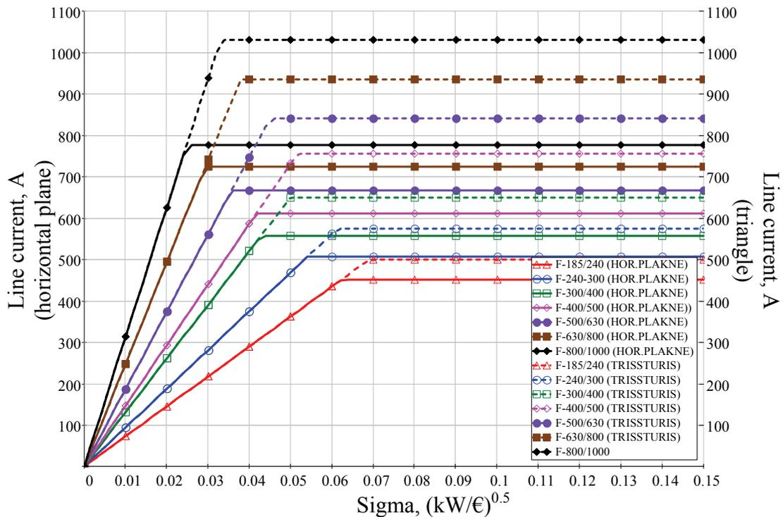
Fig. 4.5. Current nomograms for single-core 110 kV cable lines with copper conductors depending on cable laying method
