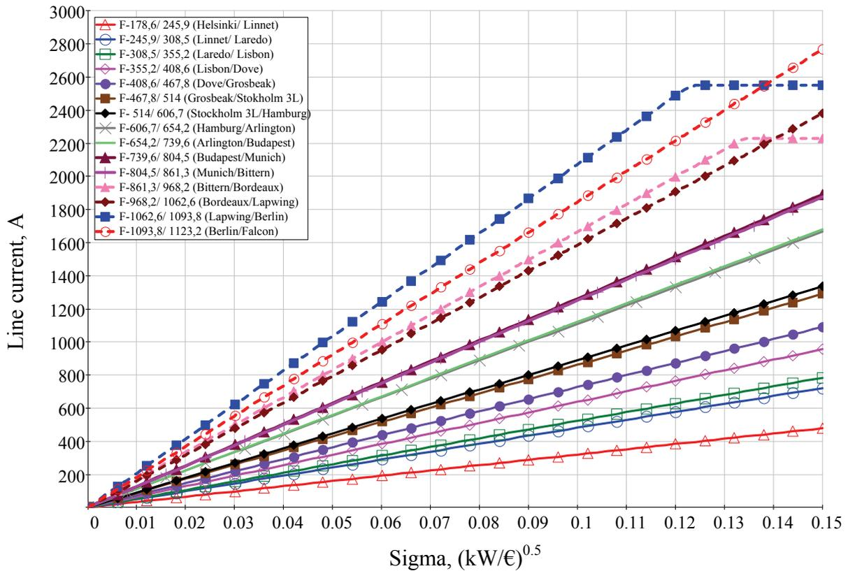
Fig. 4.3. 110 kV ACCC (Aluminium Conductor Composite Core) wire current nomograms
