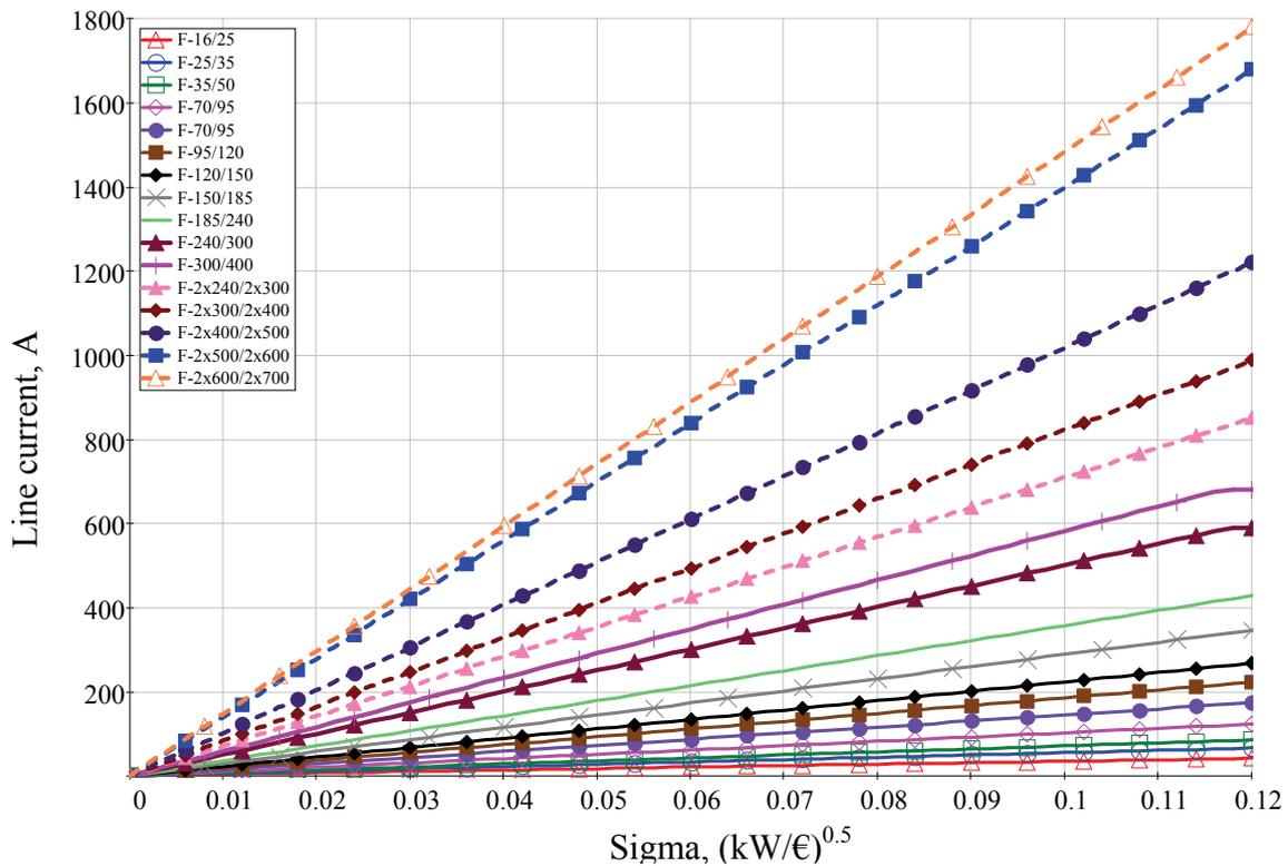
Fig. 4.1. Universal current nomograms for 0.4-10-20-110-330 kV overhead lines with aluminium conductor
