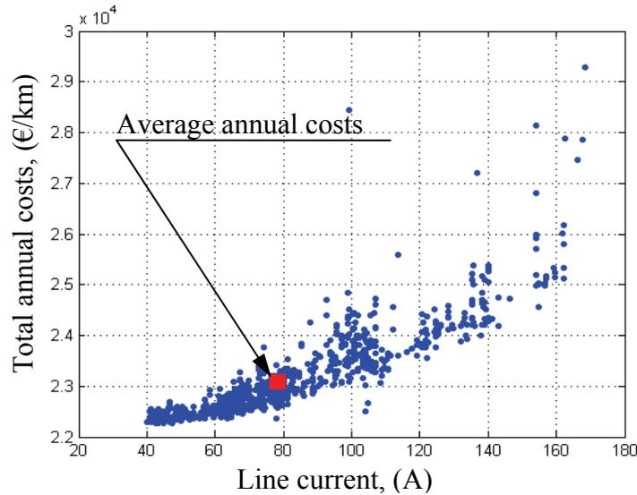
Fig. 5.4. The calculated annual exploitation and construction costs for 1xAS-240 OHL depending on the line current (the PAMC method, 110 kV).
