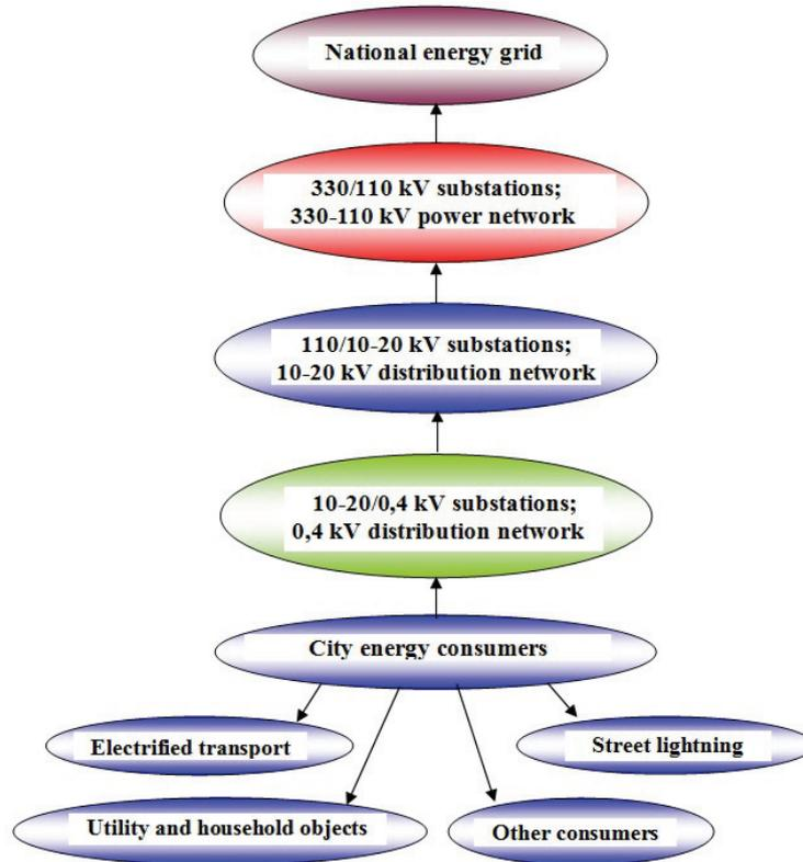
Fig. 2.2. Urban load determination algorithm after sequential generalization of the loads of network elements
