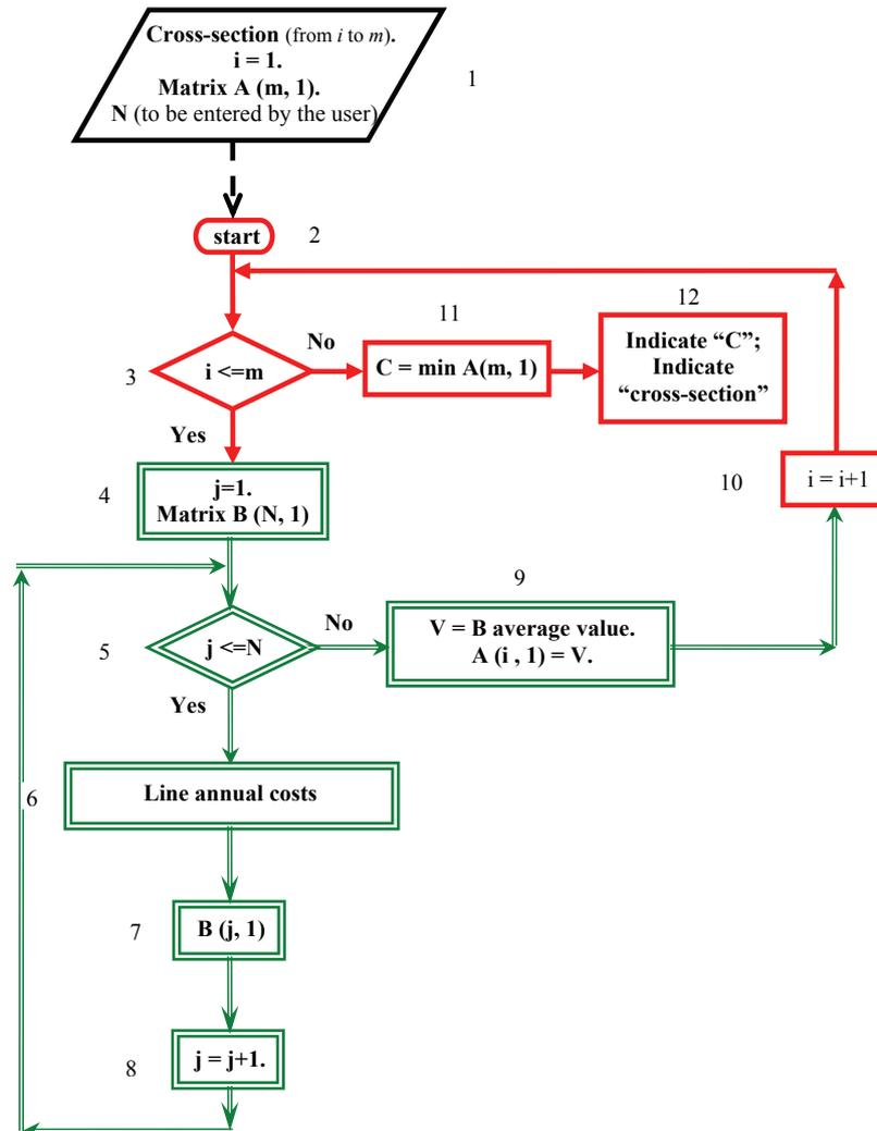
Fig. 5.3. The structure of the optimum cross-section calculation algorithm
