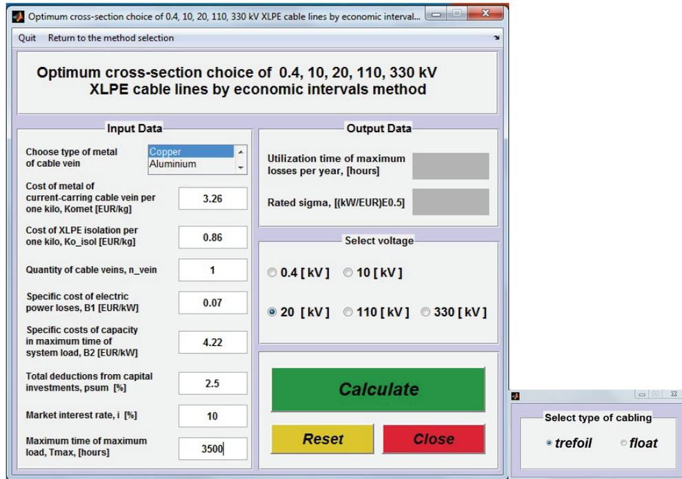
Fig. 4.7. Graphical user interface for cable lines
