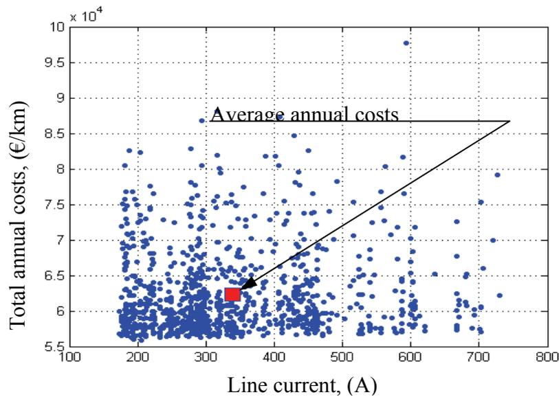
Fig. 5.5. The calculated annual exploitation and construction costs for 1xAS-600 OHL depending on the line current (PAMC method, 330 kV)
