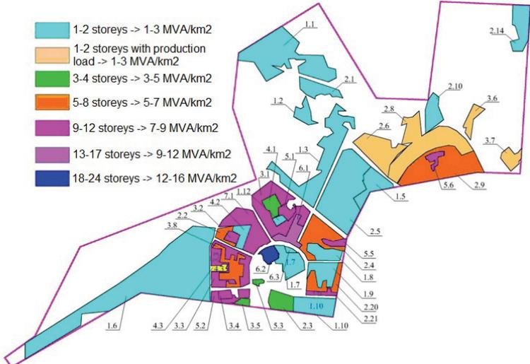
Fig. 3.2. Correction of the division of the real area of substation “Imanta” into zones according to the number of storeys
