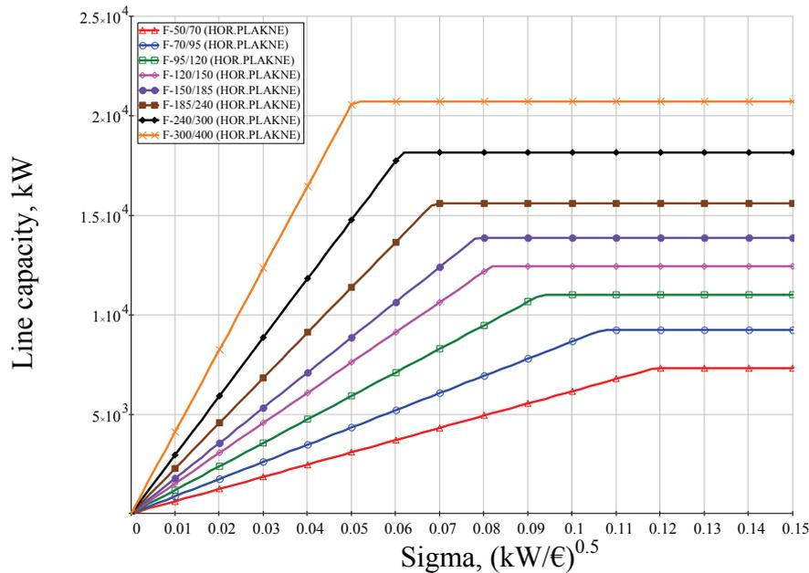
Fig. 4.4. Capacity nomograms for single-core 20 kV cable lines with copper conductors
