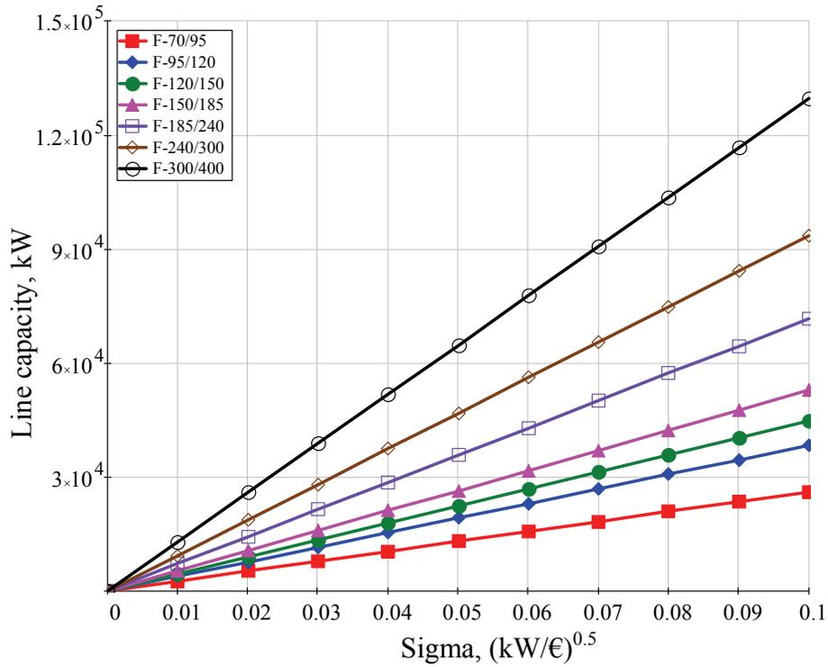
Fig. 4.2. Capacity nomograms for 110 kV overhead lines with steel-aluminium conductor
