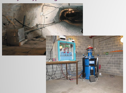
Long base watertube tiltmeter (top) and superconducting gravimeter (bottom) at the Walferdange Underground Laboratory for Geodynamics, Luxembourg
