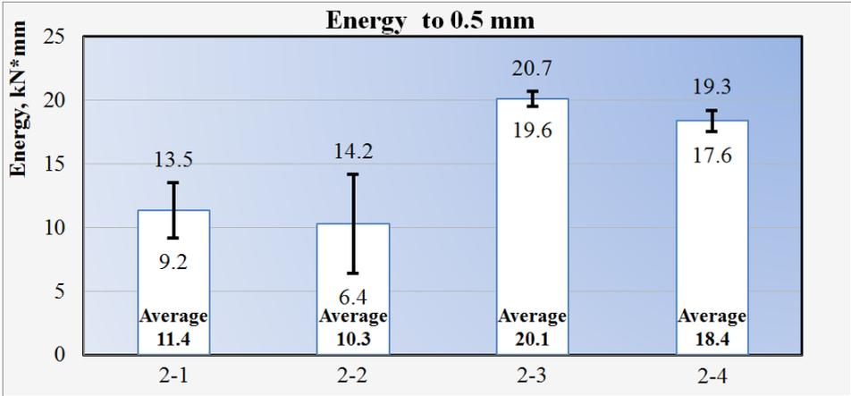
Fig. 5 Deformation energy and confidence limit to 0.5 mm
