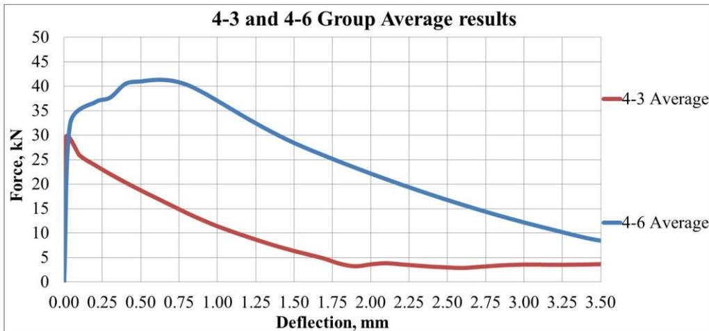
Fig. 16 Load — vertical deflection experimental graphs for specimens Group 4-3 and 4-6
