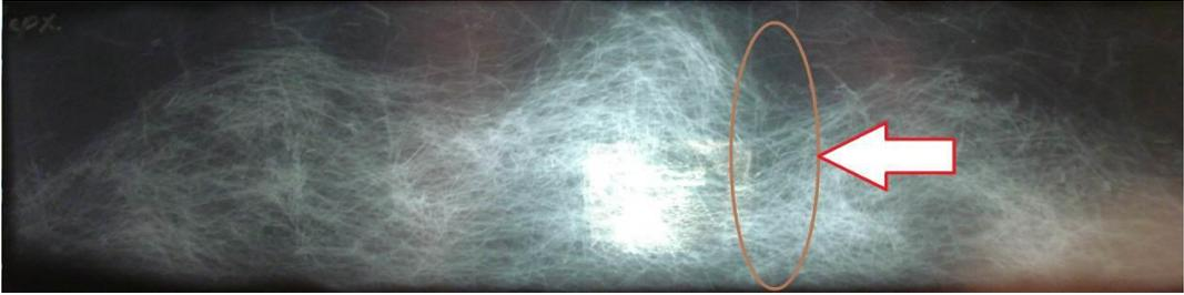
Fig. 20 SFRC specimens 5-2 X-ray image, side view [2,3]
