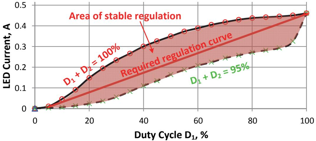
Fig. 4.4 Possible regulation area of tested non-inverting buck-boost converter controlled as combination of current source and current regulator.
