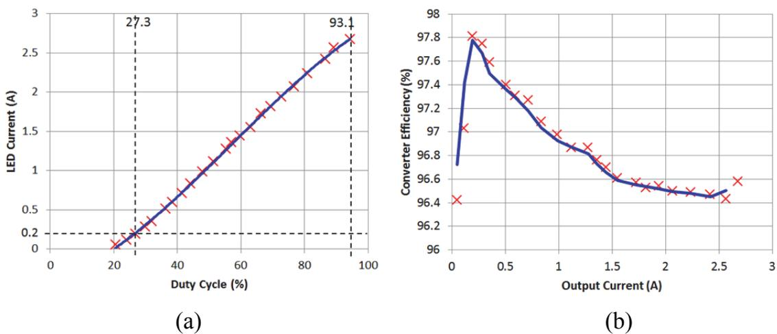
Fig. 3.6 Results of the experiments with the prototype of fitted-buck ( $\lambda = 0.1$ ) tapped-inductor converter: a) measured controllability curve; b) efficiency in the whole regulation range.
