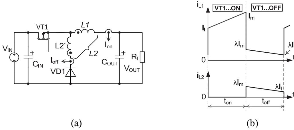
Fig. 3.7 Energy efficient inductor current measurement approach: a) possible placing of current sensor; b) typical current waveforms of tapped-inductor.
