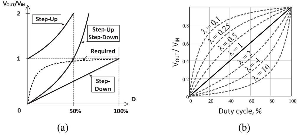
Fig. 3.2 The curve required for compensation of LED V-A curve: a) relationships between the gain of the converter and duty cycle for the conventional topologies; b) input-to-output gain curves of tapped-inductor buck converter at different duty cycles and parameter  $\lambda$  values.
