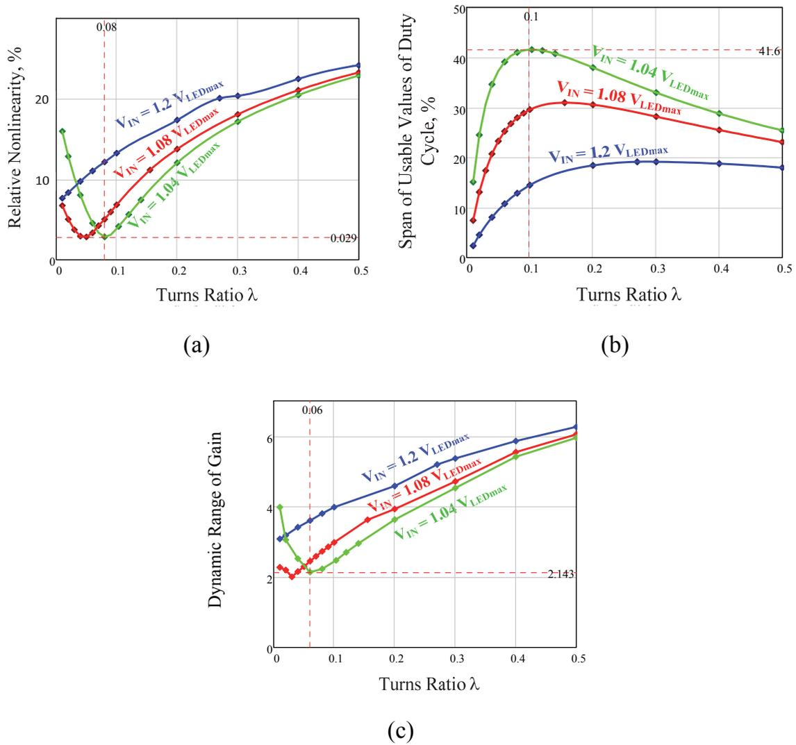
Fig. 3.5 Controllability parameters of the tapped-inductor buck converter connected to the LED load at different input voltages and tapped-inductor turns ratio  $\lambda$  values: a) nonlinearity; b) usable duty cycle span; c) dynamic range of gain.
