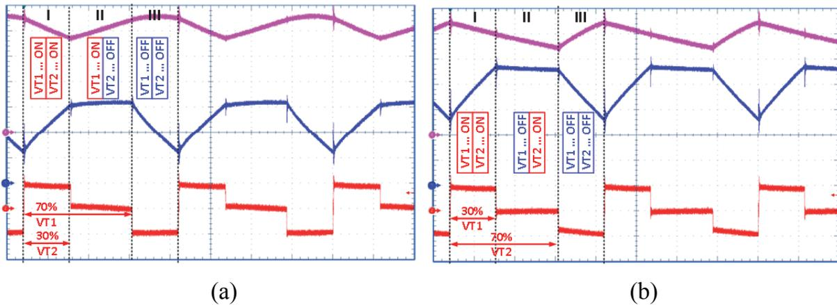
Fig. 4.3 Inductor L1 current (blue), voltage (red) and CR capacitor voltage (magenta): a) at duty cycle  $D_1 = 30\%$  of transistor VT1; b) duty cycle  $D_1 = 70\%$  of transistor VT1 (time scale is  $5 \mu\text{s}/\text{div}$ , voltage scale for inductor (red) is  $50 \text{ V}/\text{div}$ , voltage scale for capacitor is  $10 \text{ V}/\text{div}$ , but current scale is  $0.2 \text{ A}/\text{div}$ ).
