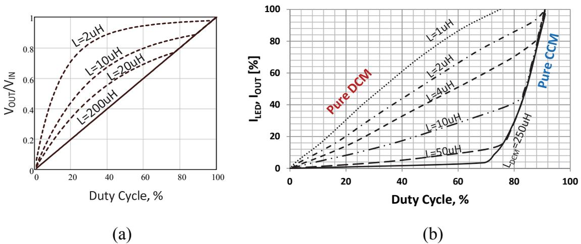
Fig. 3.9 Discontinuous conduction mode operation of the buck converter: a) with resistive load (analytical calculations); b) with LED load (obtained from experiments).
