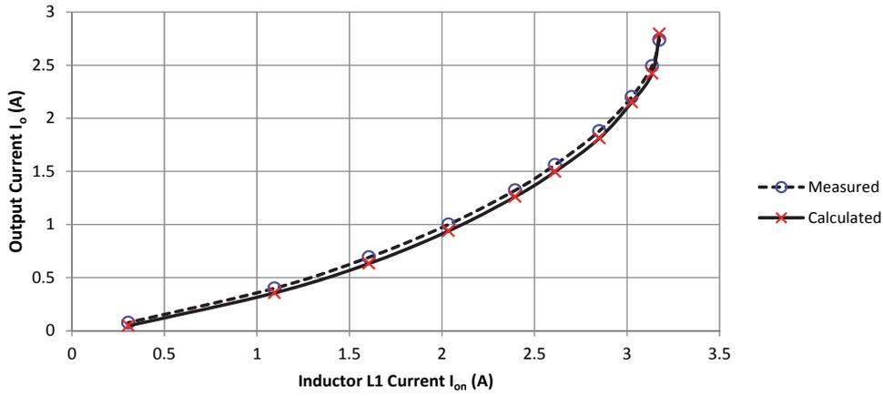
Fig. 3.8 Relationship between the output current and average current  $I_{on}$  in the primary winding of tapped-inductor: comparison of measured and calculated values of output current of the converter.
