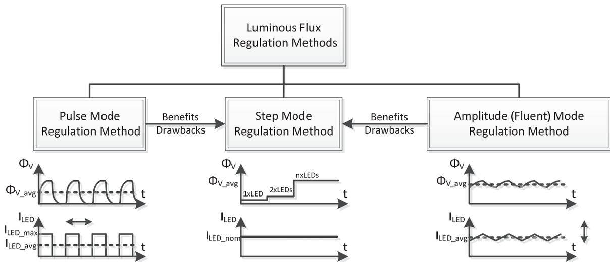
Fig. 2.3 Luminous flux regulation methods for LED lamps as well as typical waveforms of LED forward current and luminous flux.
