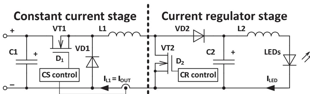
Fig. 4.2 Principal circuit of non-inverting buck-boost converter, considered to be the combination of constant current (CS) source and current regulator (CR).
