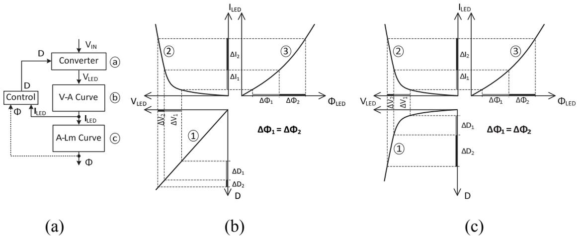
Fig. 3.1 Compensation of nonlinearity: a) simplified control chain structure; b) relationship between the duty cycle (control parameter) and luminous flux (parameter under control) in case of linear relationship of the converter; c) relationship between the duty cycle and luminous flux in case of nonlinear relationship of the converter.
