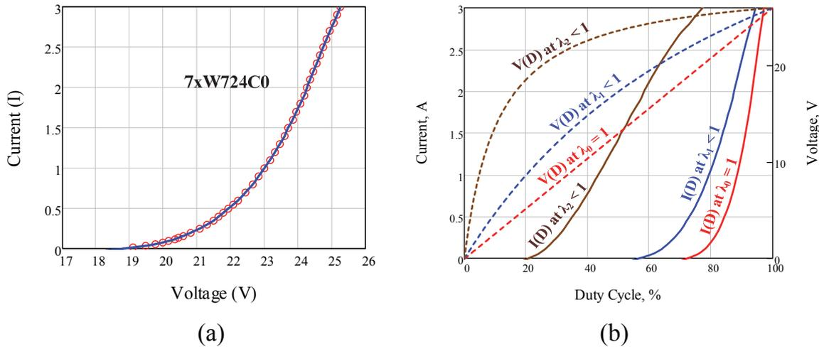
Fig. 3.4 The analysis of the loaded converter: a) V-A curve of the LED load used in experiments and for numerical calculations; b) examples of analytical relationships between the duty cycle and output voltage/current of loaded converter.
