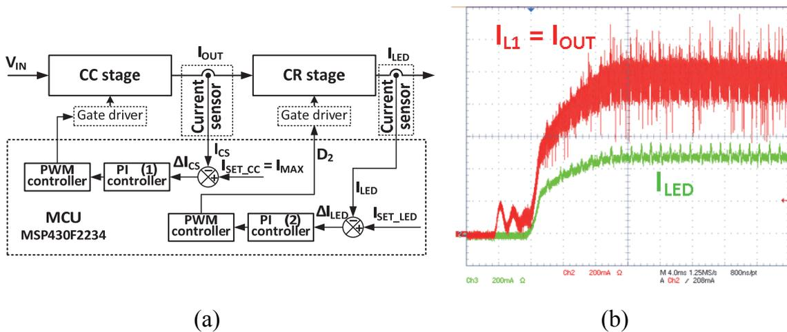
Fig. 4.5 Microcontroller based synchronous operation of transistors VT1 and VT2 of non-inverting buck-boost converter: a) block diagram of the control system; b) results of the tests — start-up process and further operation at half load.
