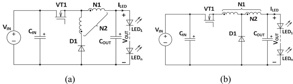
Fig. 3.3 The principal electrical circuits of tapped-inductor buck converter: a) fitter-buck converter ( $0 < \lambda < 1$ ); b) reducer-buck converter ( $\lambda > 1$ ).
