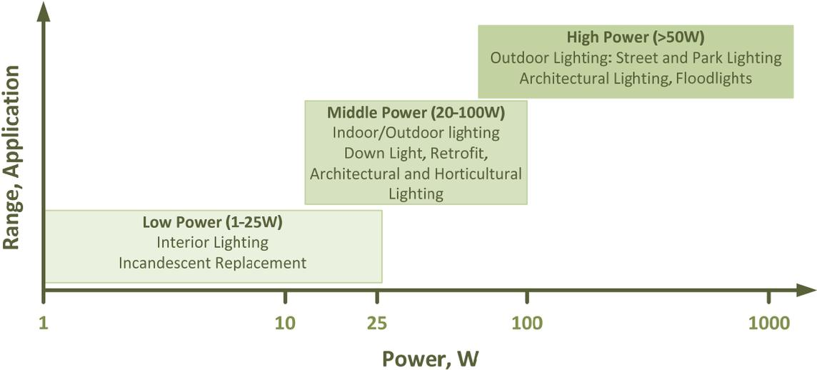
Fig. 2.2 Typical power ranges and applications of LED lamps [28].
