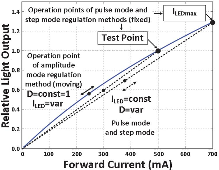
Fig. 2.4 Ampere-lumen curve of a common high power LED and operation points for different luminous flux regulation methods.
