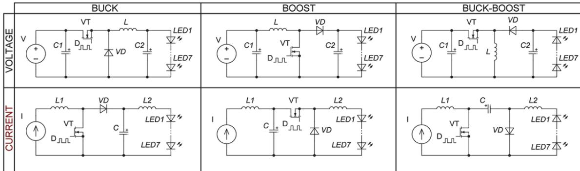
Fig. 4.1 The most widely spread VF converters and their CF versions.
