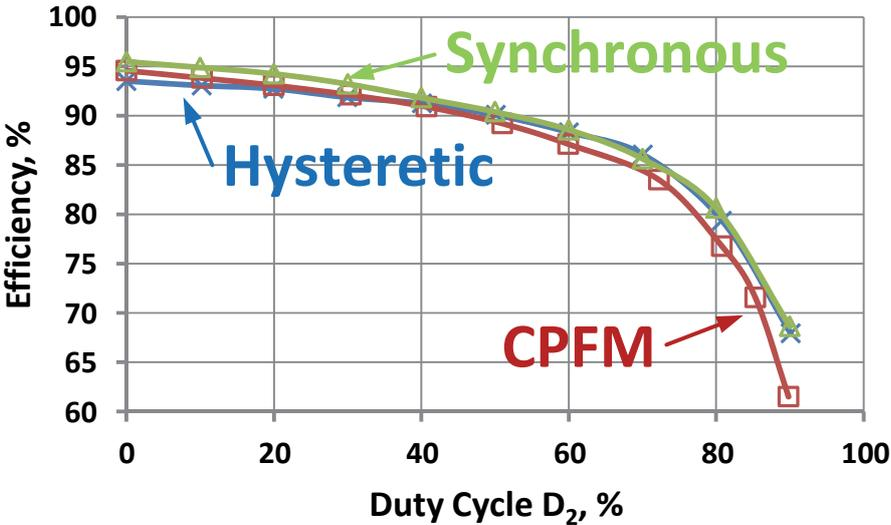
Fig. 4.6 Efficiency of non-inverting buck-boost considered to be combination of CS and CR stages using synchronous control approach and two asynchronous approaches (with hysteretic and constant pause frequency modulation controllers of CS).
