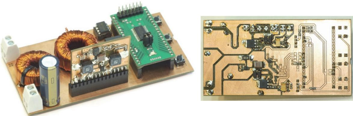
Fig. 4.7 One of the built prototypes: a) top view — the control board with a microcontroller is seen, auxiliary power supply board for control circuit and transistor driver circuits, as well as main inductor L1 and filtering inductor L2; b) bottom view — surface mount transistors VT1, VT2 and diodes VD1 and VD2, as well as CR stage capacitor.
