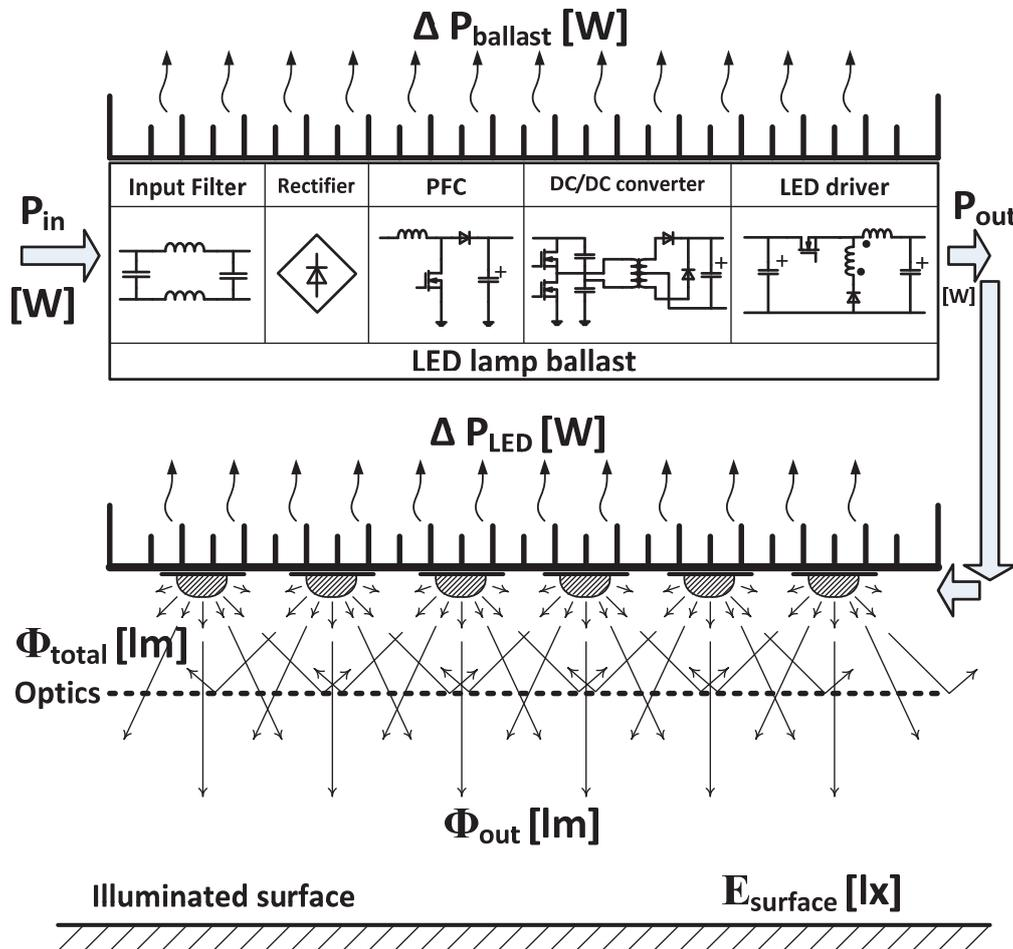
Fig. 2.1 Standard configuration of the LED lamp and the ballast for high power applications, including several conversion stages and power losses.
