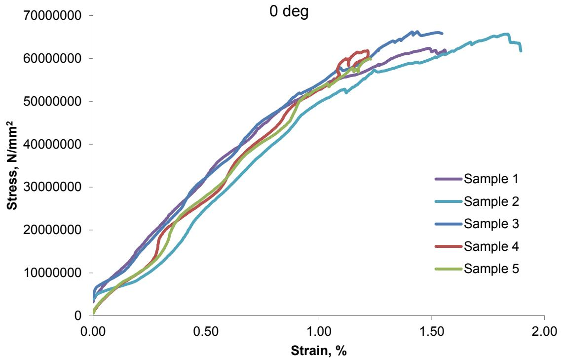
Fig. 4. Experimental results for 4-ply  $0^\circ$  samples.
