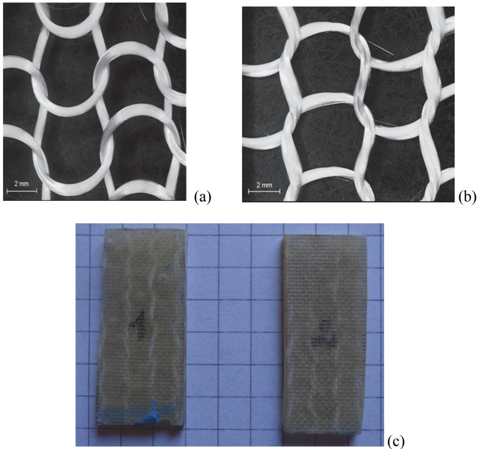
Fig. 1. Samples for microtomography analysis: fabric G2 (a), G3 (b) and 4-ply composite (c).
