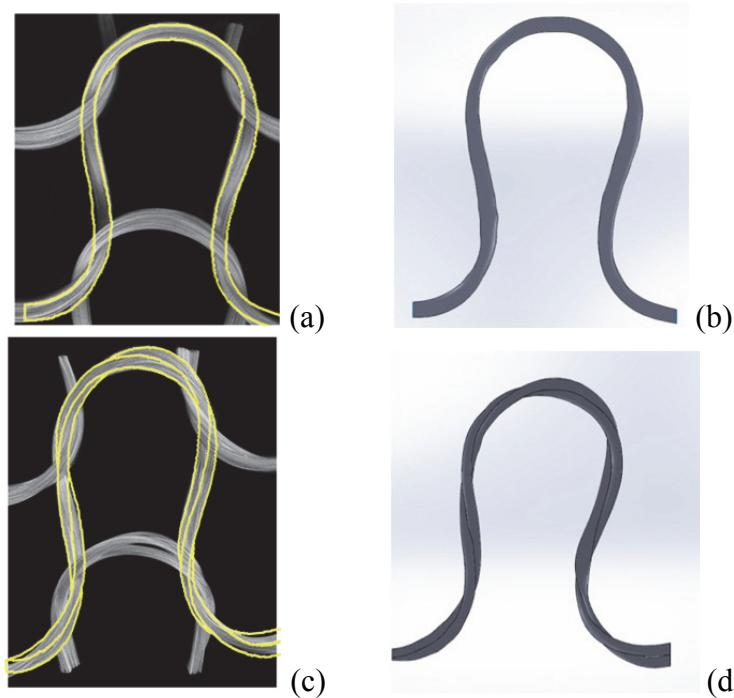
Fig. 2. Visual results of microtomography analysis for fabric G2 (a, b) and fabric G3 (c, d):
