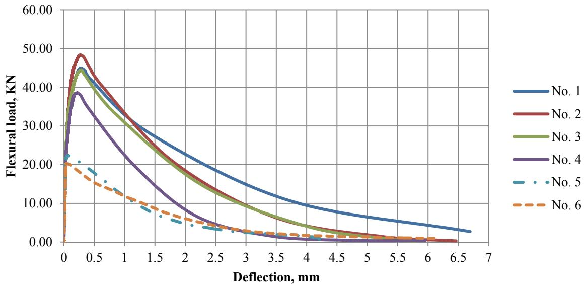
Fig. 13. Flexural load/deflection curves: samples No. 5 and No. 6 are without knitted reinforcement.
