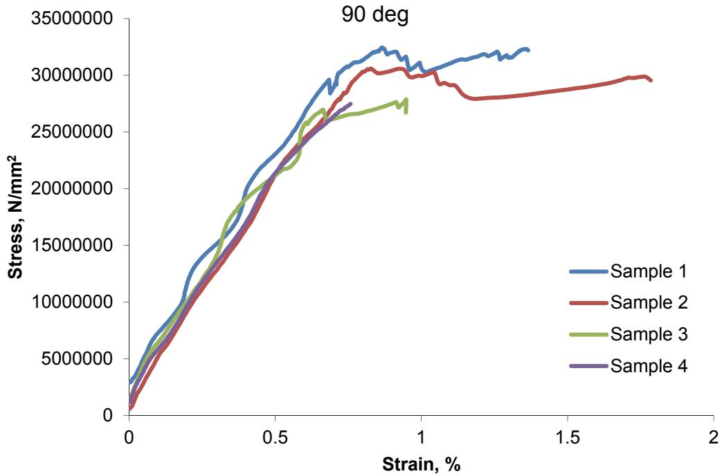
Fig. 5. Experimental results for 4-ply 90° samples.
