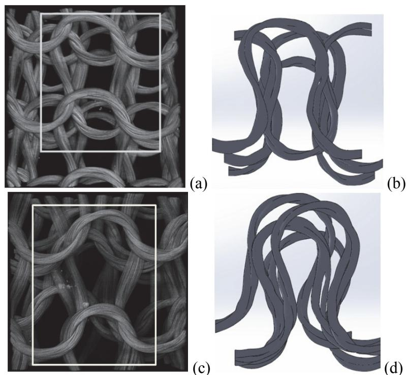
Fig. 3. Knitted fabric reinforced composite material: — Sample 1 (a–b) and Sample 2 (c–d):
