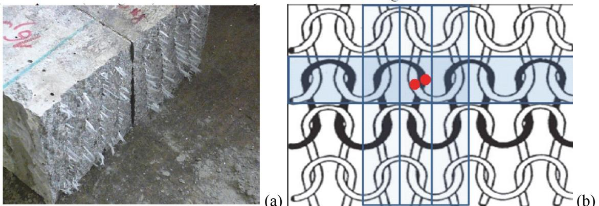
Fig. 14. (a) Concrete samples with 4-ply knitted reinforcement after fracture;
