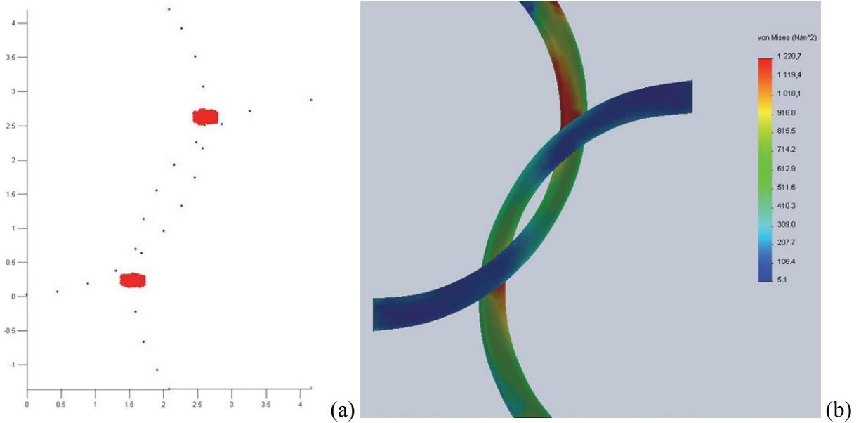
Fig. 9. Location of maximum stresses for model No. 7 — isotropic model with partly elliptical (axis ratio is 0.4) cross-section (a) and stress distribution in the respective FE model.
