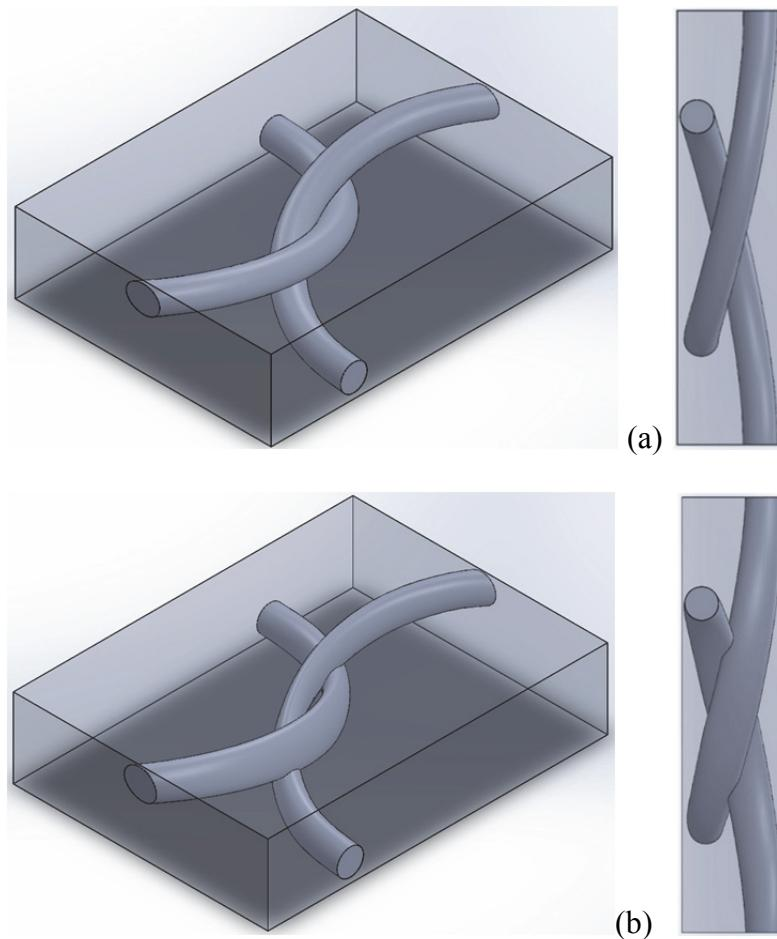
Fig. 7. Some models in an isometric view and a view from the left side: a — isotropic model with circular cross-section, b — isotropic model with partly elliptical (ellipse axis ratio is 0.4) cross-section.
