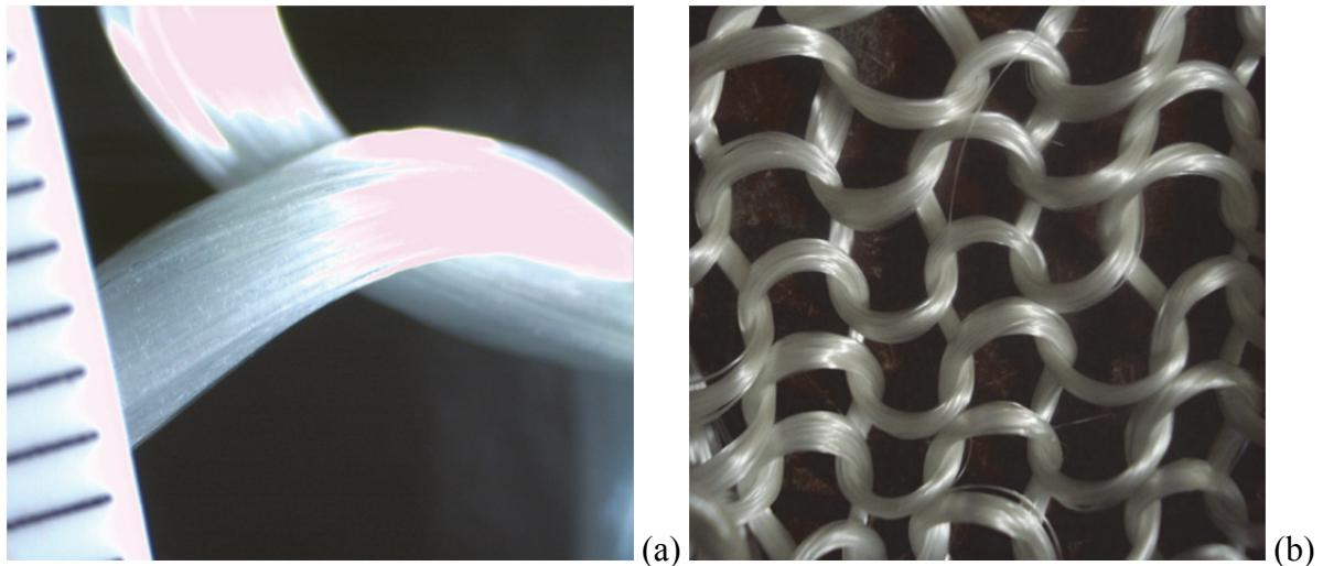
Fig. 11. Knitted fabric reinforcement: (a) yarn intersection and fragment of fabric (b).
