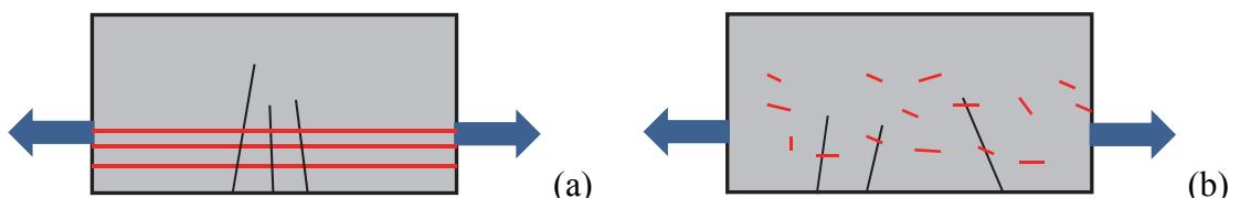
Fig. 10. Fabric (a) and short fibre (b) reinforcement under tensile load in concrete (two different load bearing mechanisms) [11].
