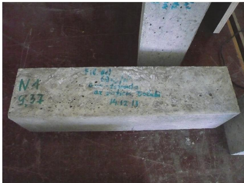
Fig. 12. Fibre concrete sample ( $100 \times 100 \times 400$  mm).
