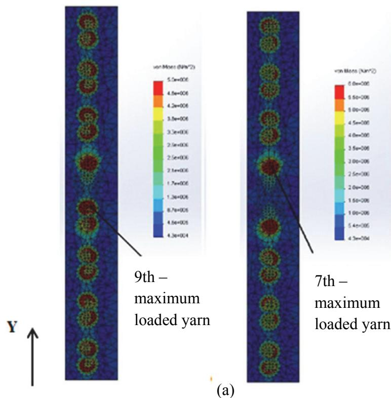
Fig. 16. Von Mises stress distribution example: (a) one yarn is broken ( $8^{\text{th}}$  from the top), (b) two yarns are broken ( $8^{\text{th}}$  and  $9^{\text{th}}$ ).
