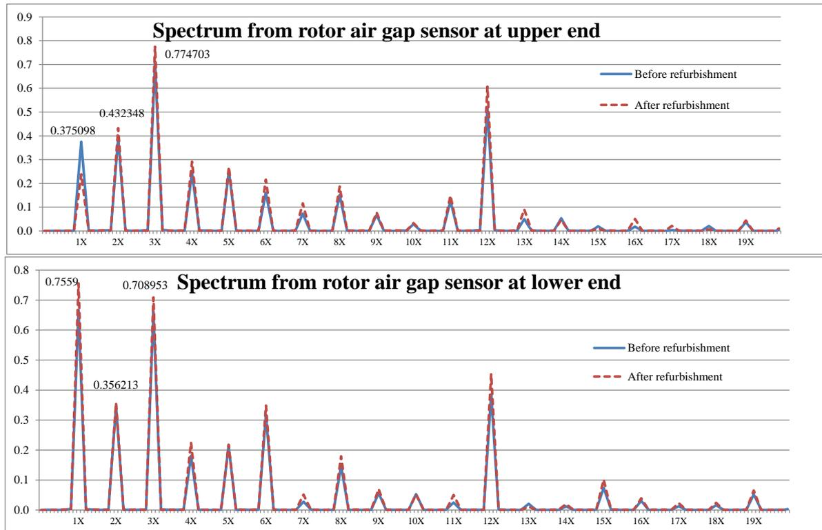
Fig. 7.2. The spectrum of the air gap for the second unit.
