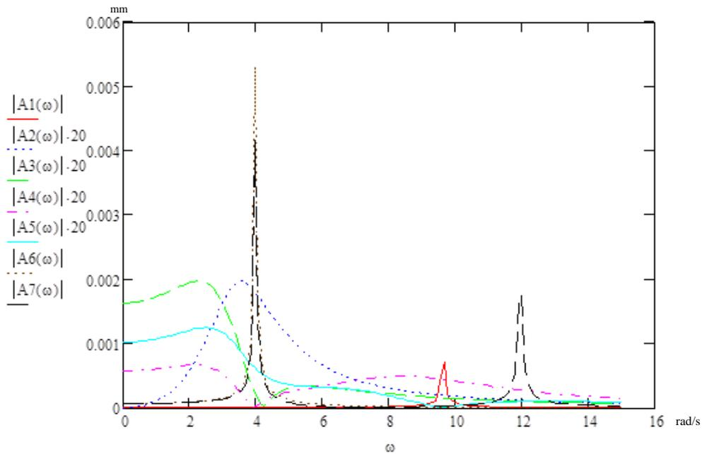
Fig. 3.1. Example for calculation of excited oscillation amplitudes and system critical rotational frequency zones from bending and torsion in MathCAD.
