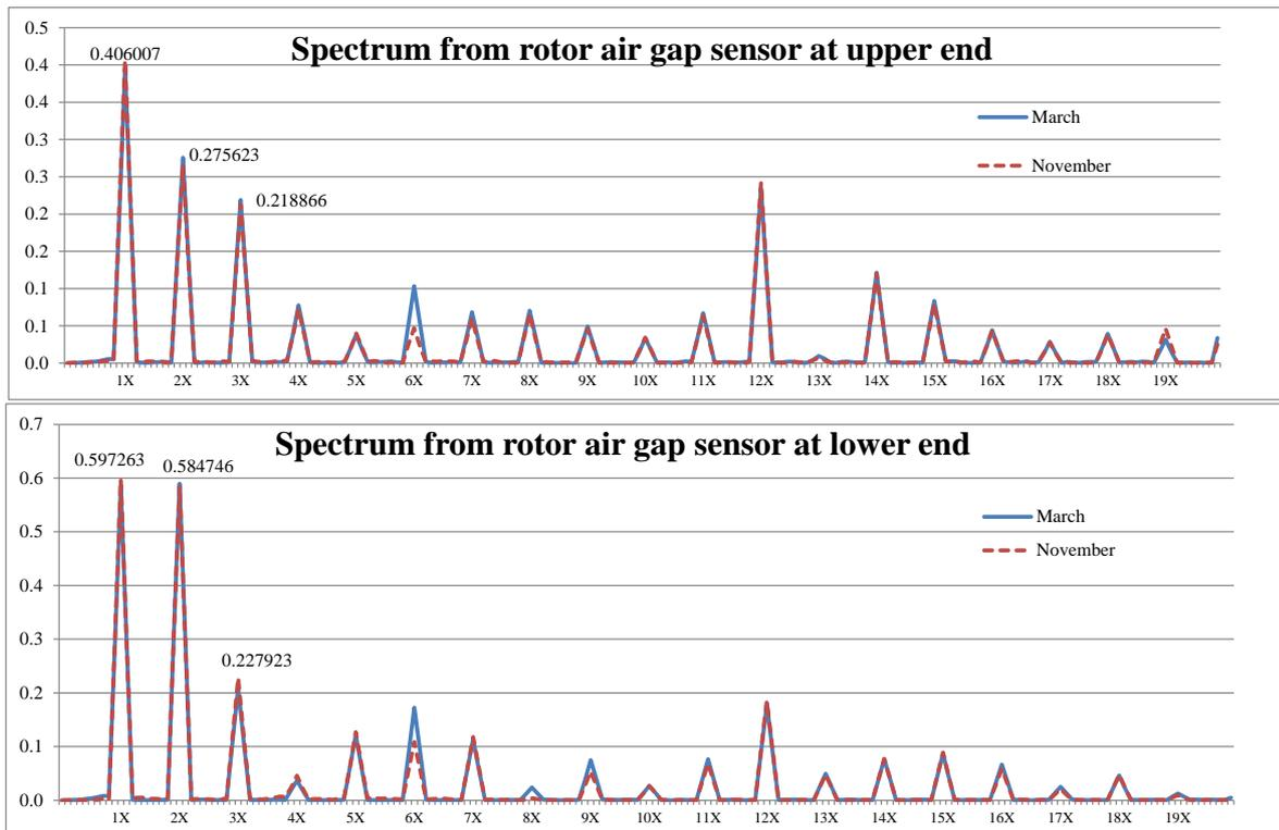
Fig. 7.1. The spectrum of the air gap for the first unit.
