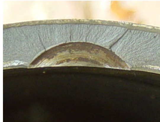
Fig. 17. Concentrator — cut (obtained after collapse)
