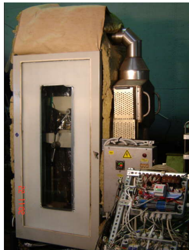
Fig. 6. Test stand thermostatic chamber
