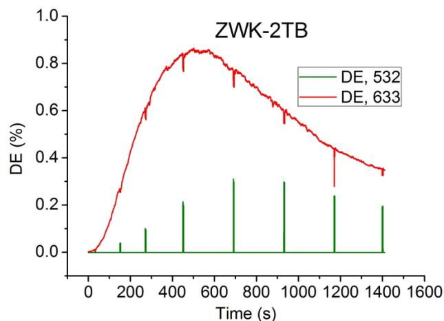
**Figure 1.** Diffraction efficiency exposure time dependences of the reflection grating recorded in ZWK-2TB film by 532 nm light and read out at 532 and 633 nm.  $A=182\text{ nm}$ , readout angles  $\theta_{inc}(532)=20^\circ$ ,  $\theta_{inc}(633)=25^\circ$ .
