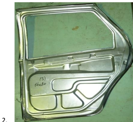
Fig.14. Back door of a car of series 2118 which was obtained with the proposed technology
