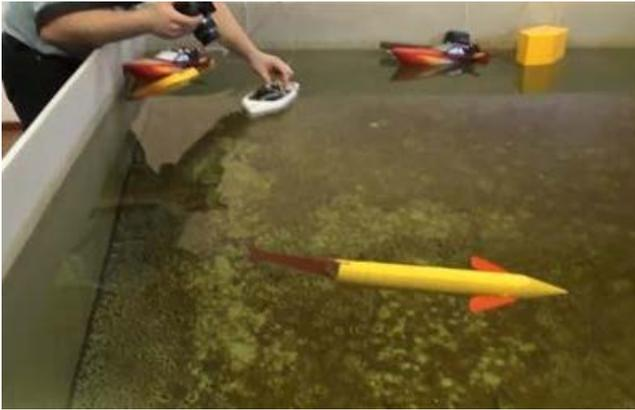
Fig. 11. Straight corners water tank with some floating devices. In the forefront is robot *RR-9* in neutral floating (before motion starts). Robot is controlled using three actuators: a tail frequency actuator for propulsion force generation, a steering angle exchange actuator and an up or down motion control actuator (by side fin rotation angle exchange).
