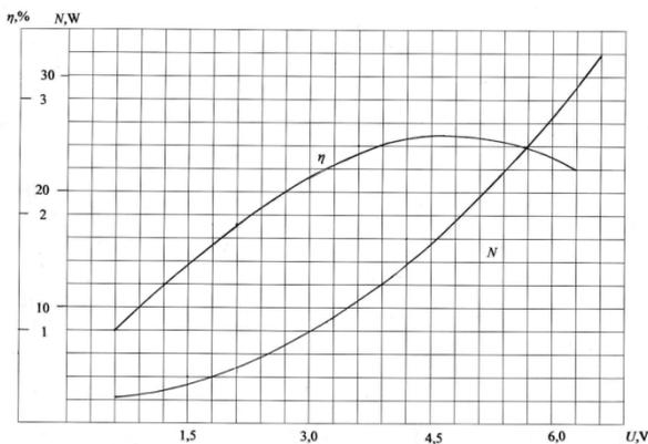
Fig. 8. Power consumption  $N$  and efficiency  $\eta$  dependence as function of voltage  $U$  of the electric motor. Extreme is in the region  $U = 4.8$  V.
