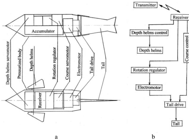
Fig. 5. Fish robot *RR-9*: a – a design; b – the management scheme.
