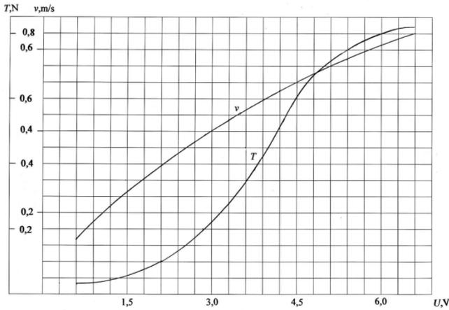
Fig. 7. Swimming speed  $v$  and draught  $T$  dependence as function of voltage  $U$  of the electric motor.
