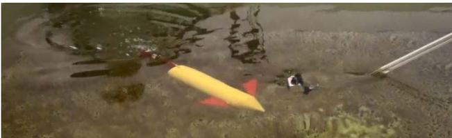
Fig. 12. Start of the diving motion of robot *RR-9* in water tank. On the right side under water video camera can be seen.
