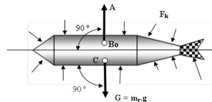
Fig. 1. Oversight scheme of robot at horizontal rest position.  $C$  – center of mass;  $Bo$  – center of buoyancy;  $G$  – gravity force;  $A$  – Archimedes force.
