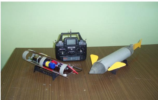
Fig. 6. The general view of fish robot *RR-9* (with the radio management panel).
