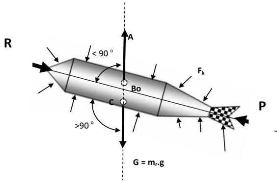
Fig. 2. Oversight scheme of robot on oblique position.  $C$  – center of mass,  $Bo$  – center of buoyancy,  $G$  – force of gravity,  $A$  – Archimedes' force,  $R$  – force of water resistance,  $P$  – propulsion force.
