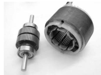
Fig. 9. Rotor and stator from a stepper motor.
