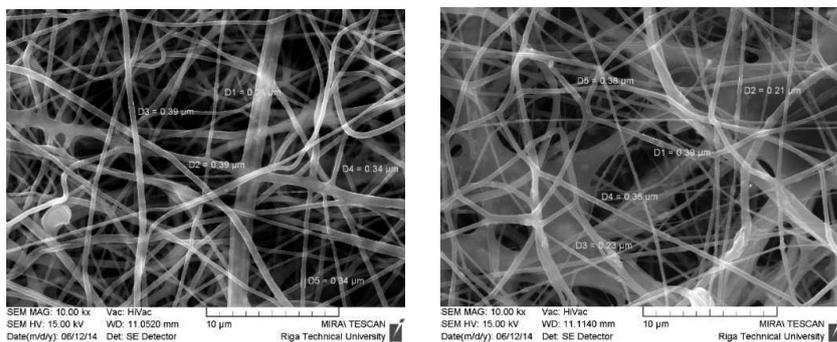
Figure 1. SEM micrographs of PVA/TiO<sub>2</sub> (a) and PVA/NF/TiO<sub>2</sub> (b) nanofiber composites morphology
