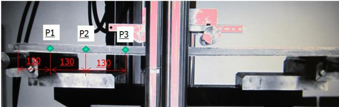
Figure 4.7 Location of intermediate markers for displacement track.
