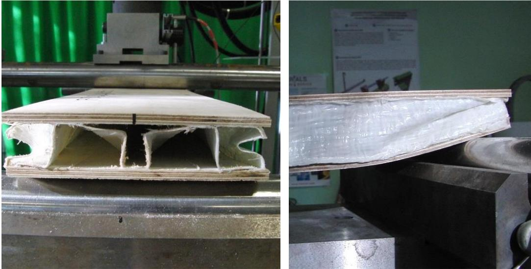
Figure 4.28. Failure mode of the double section sandwich panel.
