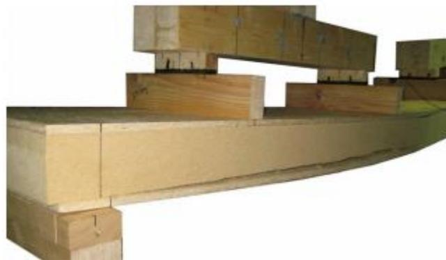
Figure 1.15. Facade sandwich panel in 6-point bending [90].
