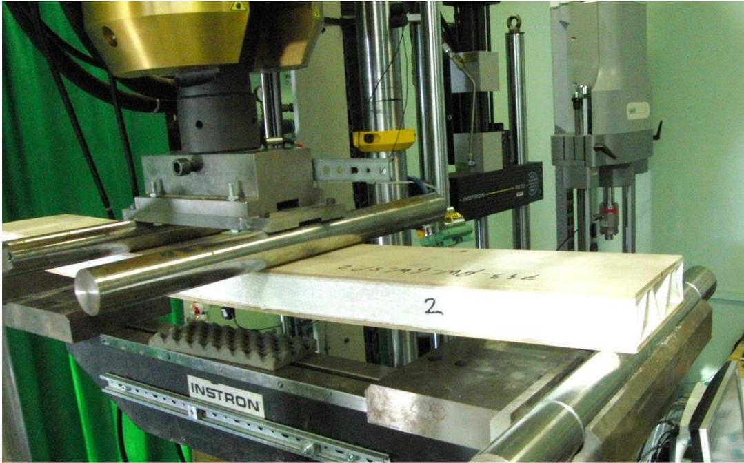
Figure 4.24. 4-point bending test of the double-section sandwich panel on INSTRON 8802.
