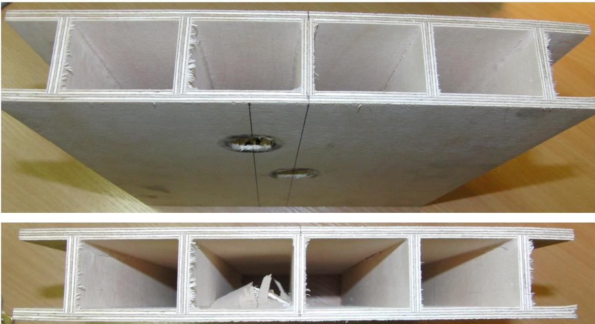
Figure 8.13. Inside view of the sandwich panel.
