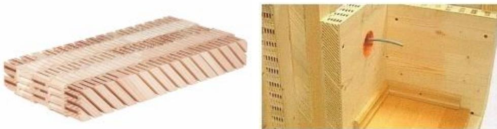
Figure.1.10 Cellular wood material — application in building walls [78].
