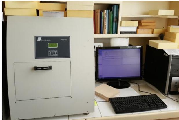
Figure 2.11. Linseis HFM 300 test set-up.
