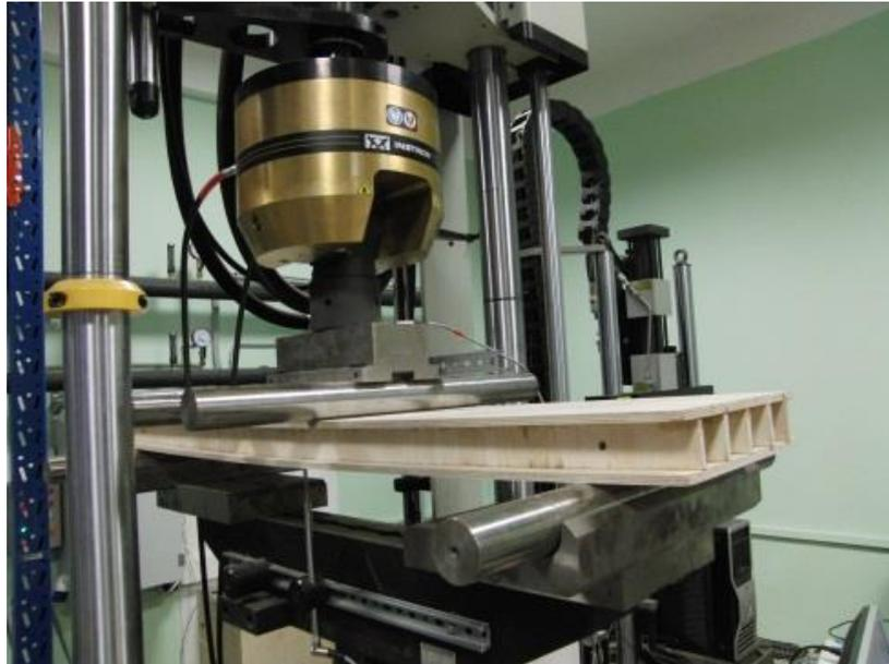
Figure 3.3. Testing of plywood sandwich panels in 4-point bending set up on INSTRON 8802.
