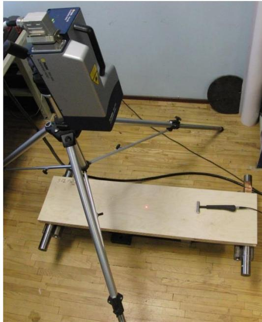
Figure 7.10. Test set-up for hammer impact test.
