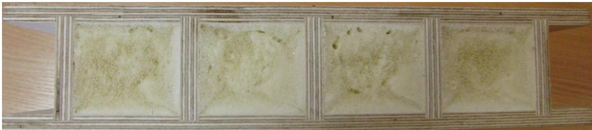
Figure 6.4 Cross-section of rib-stiffened sandwich panel with foam core.
