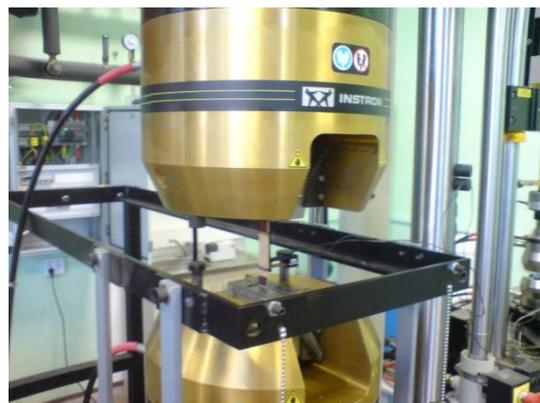
Figure 2.3. Specimen tension test on INSTRON 8802.
