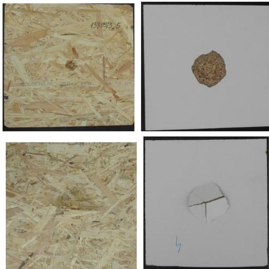
Figure 8.5 Damaged areas for OSB and particle board.
