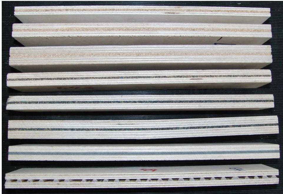
Figure 8.7. Side view of plywood specimens with thin middle layer.
