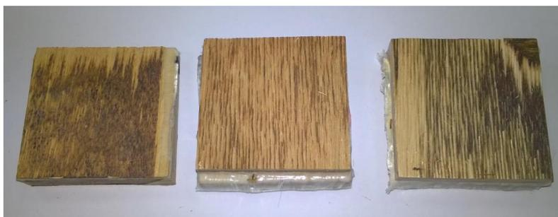
Figure 2.15. Samples after the EN 319 tests.
