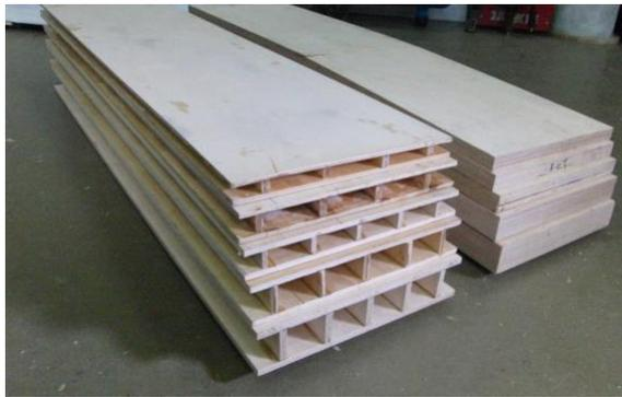
Figure 3.7 Prototyped sandwich panels in comparison with conventional plywood boards.
