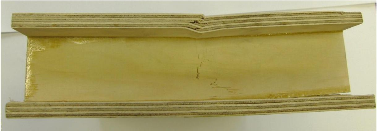
Figure 3.12 Failure of the faces and core (Cutted middle section)
