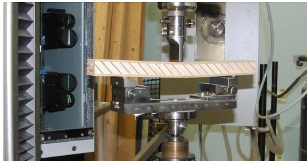
Figure 5.6. 3- point bending test set-up on ZWICK Z100.
