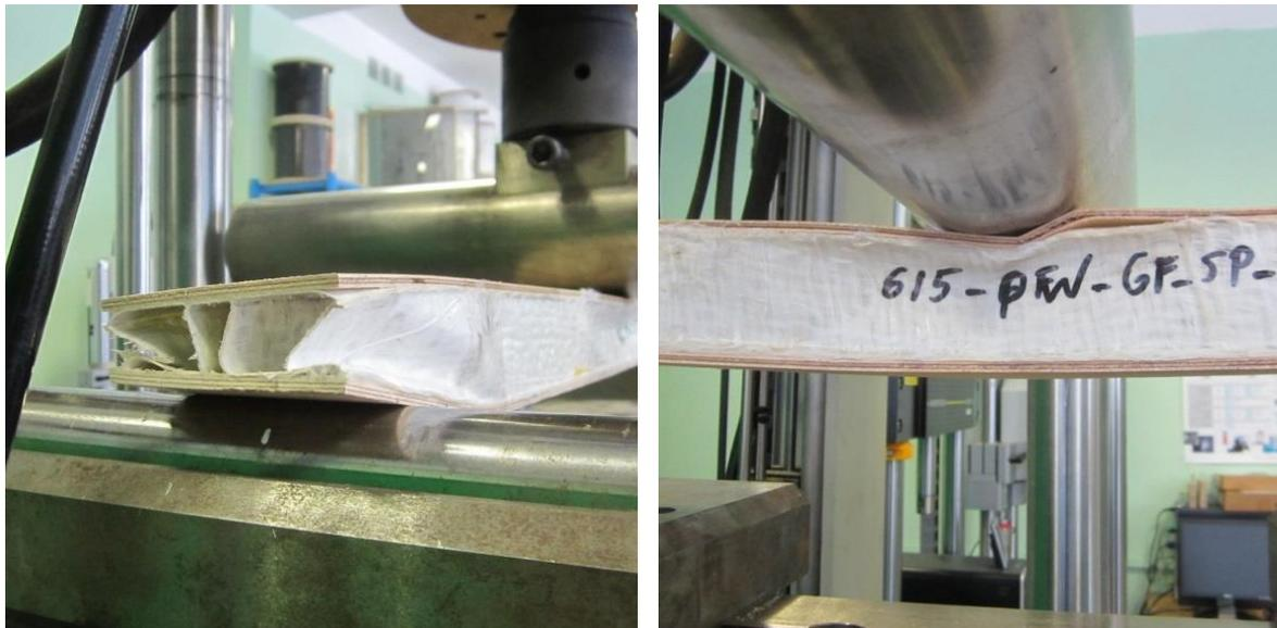
Figure 4.29. Failure of the support for the single-section sandwich panel.
