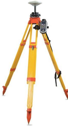
**Fig. 3.2.** Equipment for accurate GNSS receiver setting.
