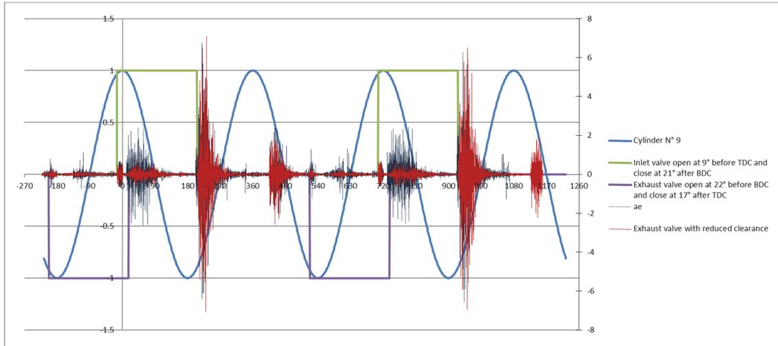
Fig. 4.5. Exhaust valve with reduced clearance
