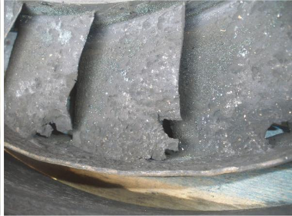
Fig. 1.4. Damaged turbocharger
