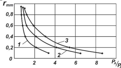
Fig. 4.12. Range limits for compressed air leakage in subsonic turbulent flow mode
