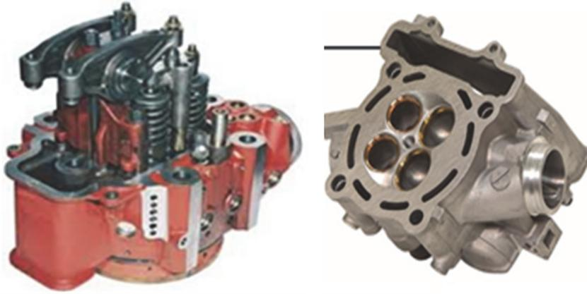
Fig. 2.1. Medium and high-speed diesel engine heads
