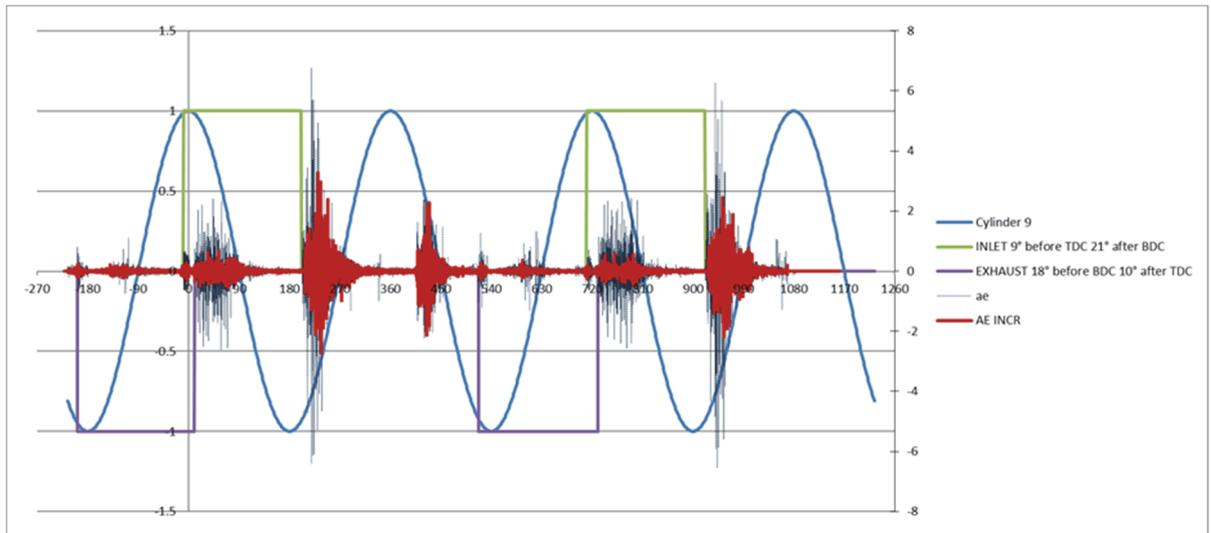
Fig. 4.7. Inlet valve with crack
