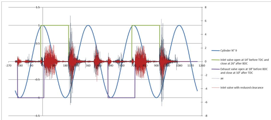
Fig. 4.4. Inlet valve with reduced clearance
