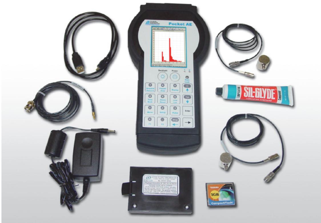
Fig. 2.2. Measuring Pocket AE-2 equipment
