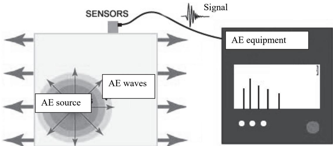
Fig. 1.6. Working principle of the AE method
