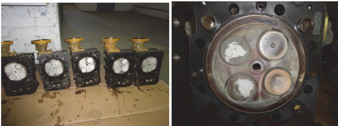
Fig. 4.8. Cylinder heads and valves checked with a capillary / liquid penetration method
