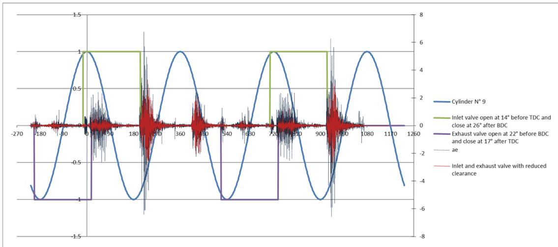
Fig. 4.6. Inlet and exhaust valve with reduced clearance
