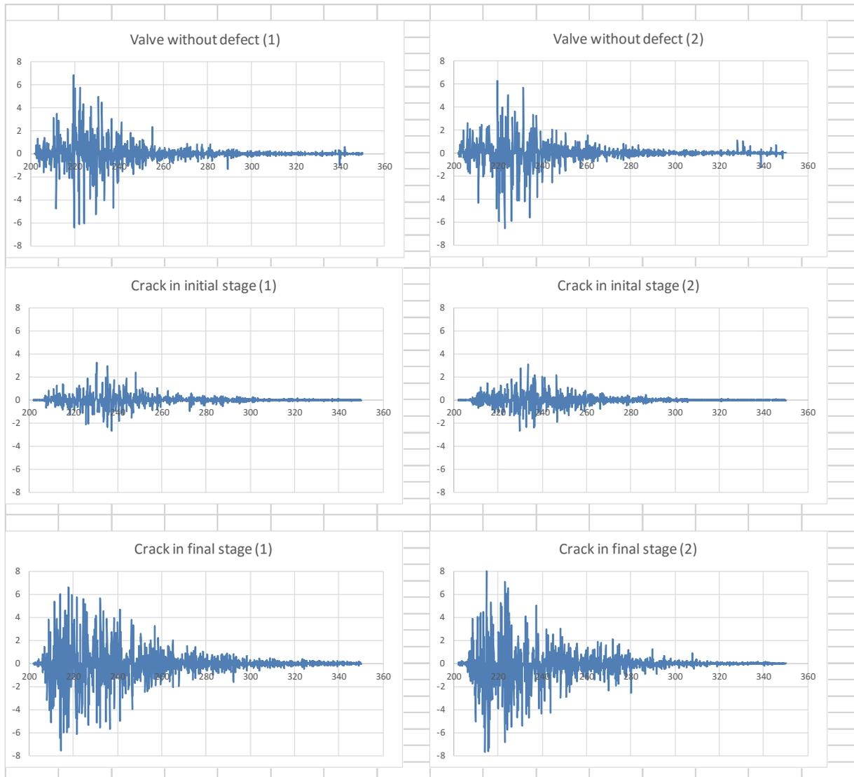
Fig. 4.11. Graphical representation of measurement for valve with the crack (X-axis: crankshaft turning angle; Y-axis: signal amplitude (V))
