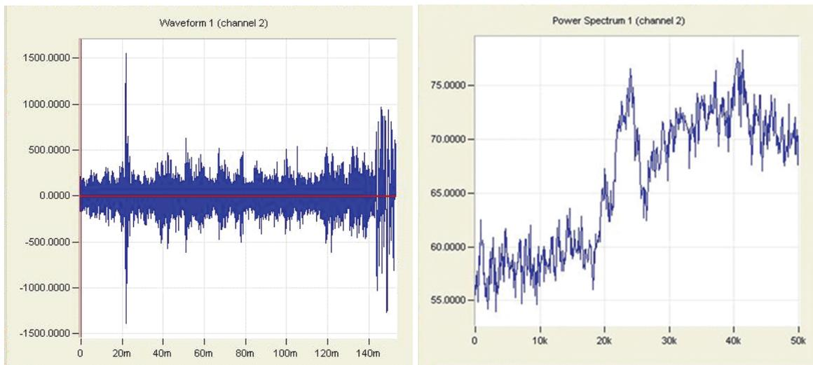
Fig. 4.1. AE waveform and spectrum at the engine flywheel
