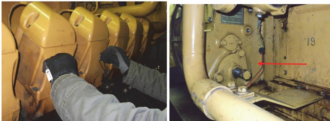
Fig. 2.7. AE sensor strengthening at the cylinder head and connection to the hall transducer
