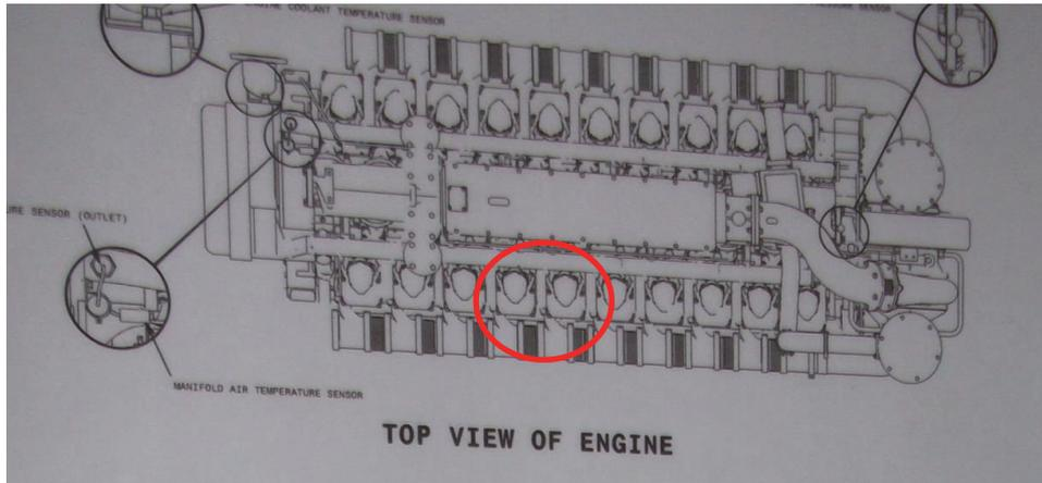
Fig. 2.5. AE sensor mounting location (cylinder head 7 and 9)
