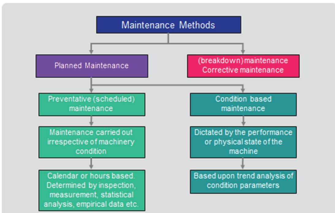
Fig. 1.5. Current maintenance methods
