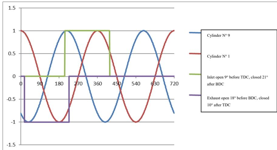
Fig. 4.3. Operation of piston n° 1 and n° 9 motion curves and inlet, exhaust valves (X-axis: crankshaft turning angle; Y-axis: relative value)
