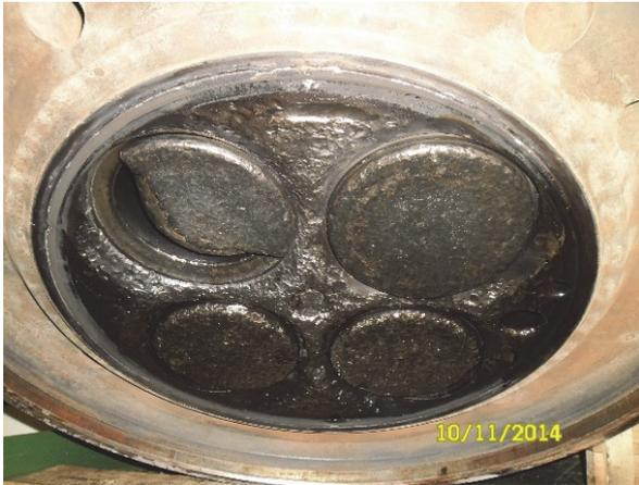
Fig. 1.1. Damaged exhaust valve
