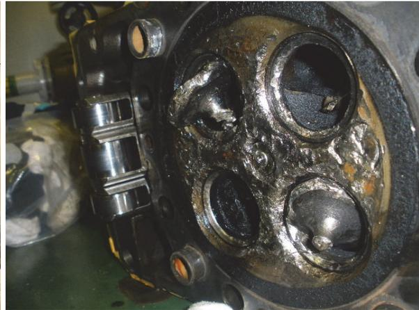
Fig. 1.2. Damaged exhaust valves and cyl.head
