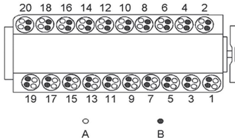
Fig. 2.4. Engine cylinder and valve location scheme
