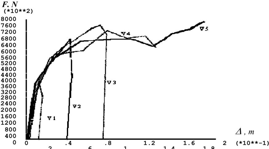
Figure 5. Expansion effort vs. working stroke of mandrel velocity:  $V_1 - 1\text{m/s}$ ,  $V_2 - 2\text{m/s}$ , ...,  $V_5 - 5\text{m/s}$
