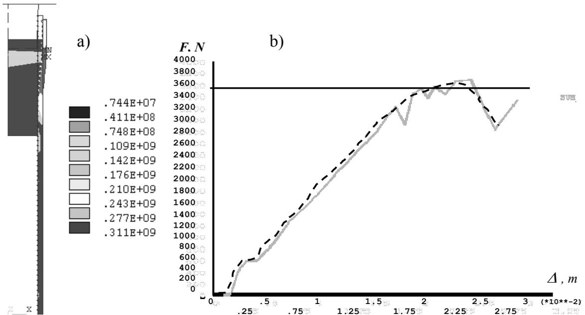
Figure 4. The equivalent stress (a) and expansion effort vs. working stroke of mandrel (b)
