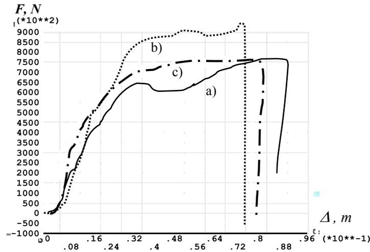
Figure 7. Calculation of expansion effort vs. working stroke of mandrel for different forms of cone generating line: a) – straight line, ——— –  $RAD = \infty$ ; b) – concave line,  $\cdots$  –  $RAD = 0,04m$ ; c) – convex line,  $-\cdot-\cdot-$  –  $RAD = 0,04m$ ,  $\dot{x} = 3,05 \text{ m/s}$
