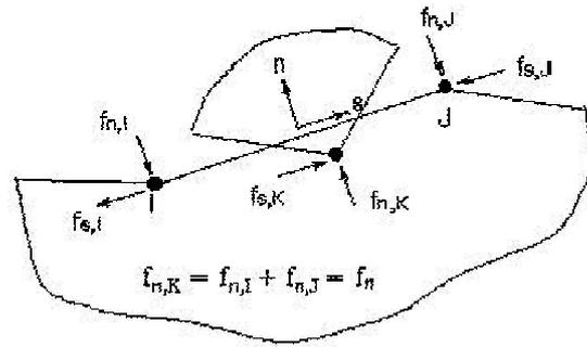
Figure 3. Scheme of contact forces with Coulomb friction
