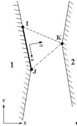
Figure 2. Scheme of contact element
