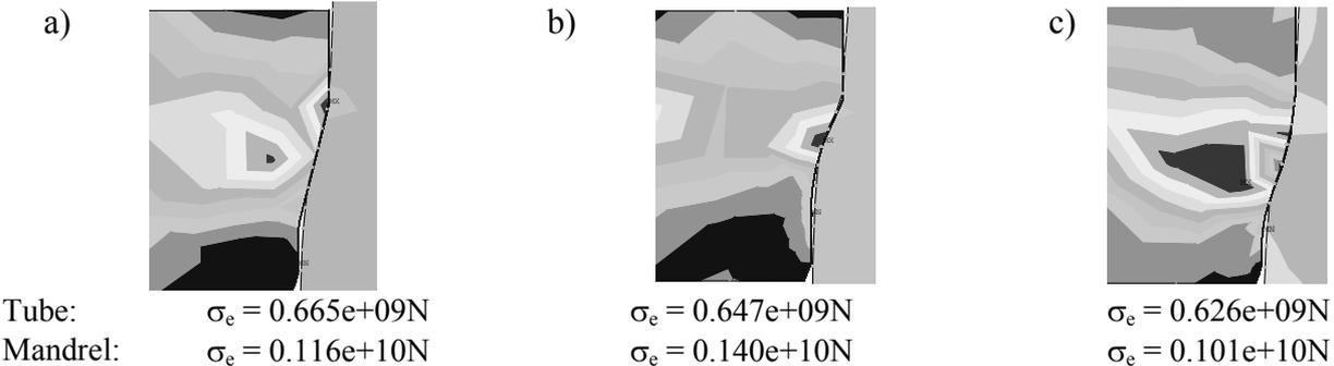
Figure 6. The equivalent stress  $\sigma_e$  of plastic working element for different forms of the cone generating line of mandrel: a) – straight line, b) – concave line, c) – convex line. Speed of loading –  $\dot{x} = 3,05\text{ m/s}$
