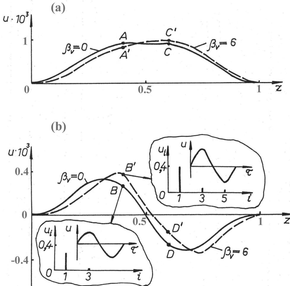
Figure 3. Modes of pipe resonant flexural vibrations: (a) the first resonant mode; (b) the second resonant mode
