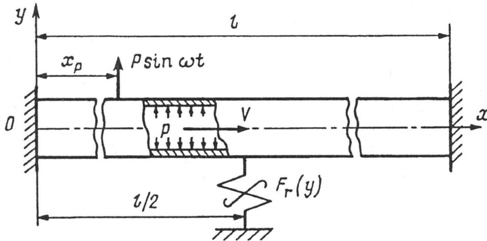
Figure 1. Dynamic model of the flow meter
