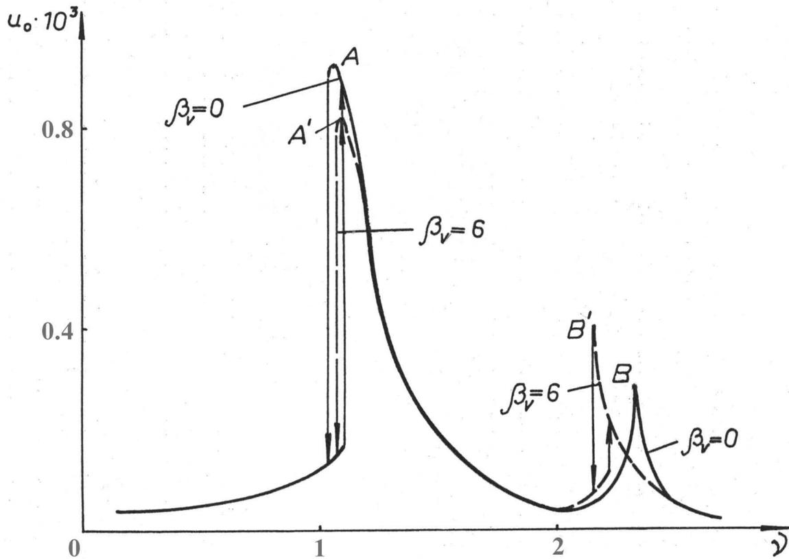
Figure 2. Amplitude-frequency characteristic of the pipe flexural vibrations
