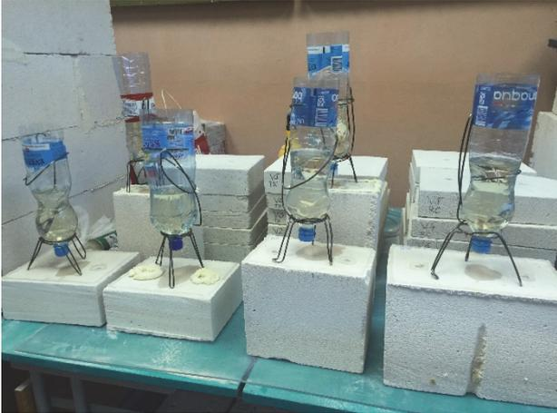
Fig.2.55. Stand of the water application on the AAC masonry blocks in condition of water droplets
