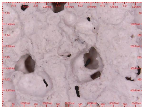
Fig.2.59. Macropore distribution throughout the cross section of the AAC sample (parallel to the manufacturing direction) D type of AAC in table 2.1.
