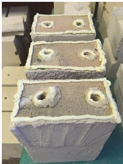
Fig.2.54. Samples with application of water on the top of the samples
