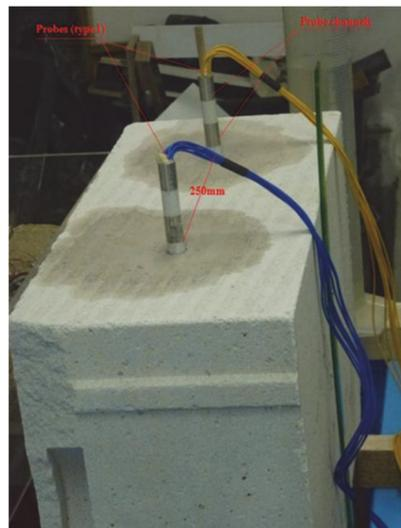
Fig. 1.13. Type 1 probes inserted in autoclaved aerated concrete block
