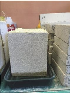
Fig.2.53. Monitoring of capillary suction of water in AAC masonry block
