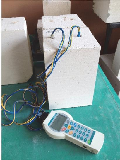
Fig. 1. Z-meter III device with measurement probes.
