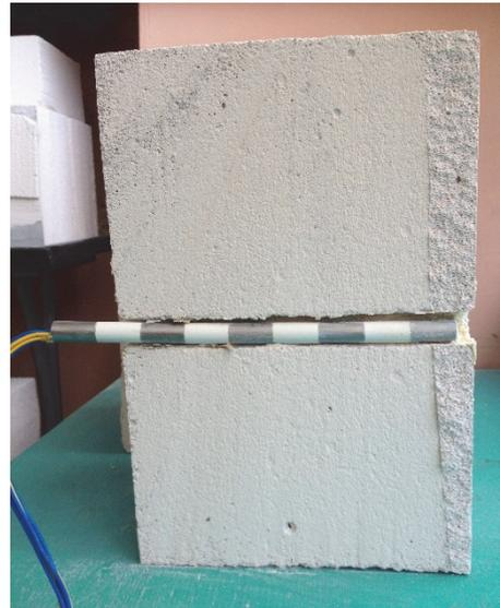
Fig.2.37. Example of measurement probe embedment in fragment of autoclaved aerated concrete block
