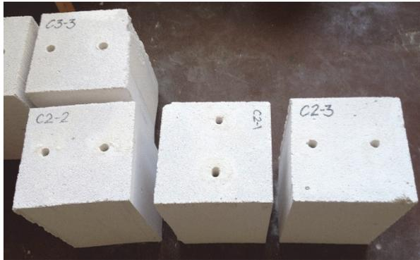
Fig.2.36. Specimen of autoclaved aerated concrete blocks bores for measurement probes
