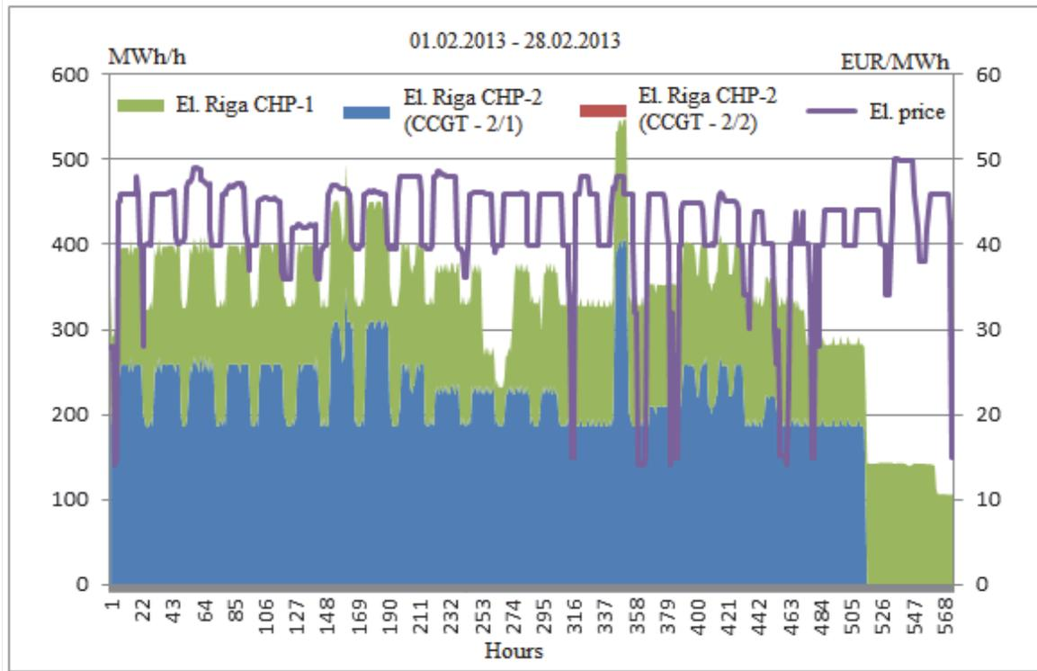
Fig. 12. Riga CHP operation in February 2013: CCGT 2-2 was not launched into operation (prior to joining NPS) (by the author according to production data of Riga CHP plants).
