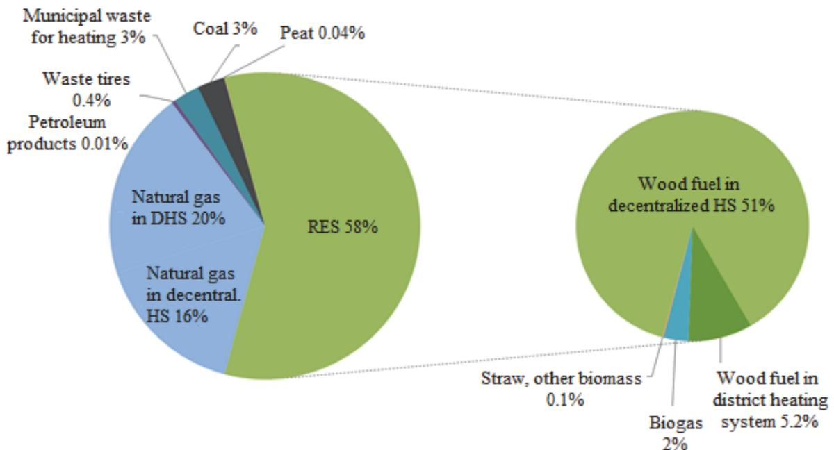
Fig. 2. Breakdown of the consumption of energy sources in 2014 in final consumption of heat energy 86.5 PJ (24.0 TWh) [1].
