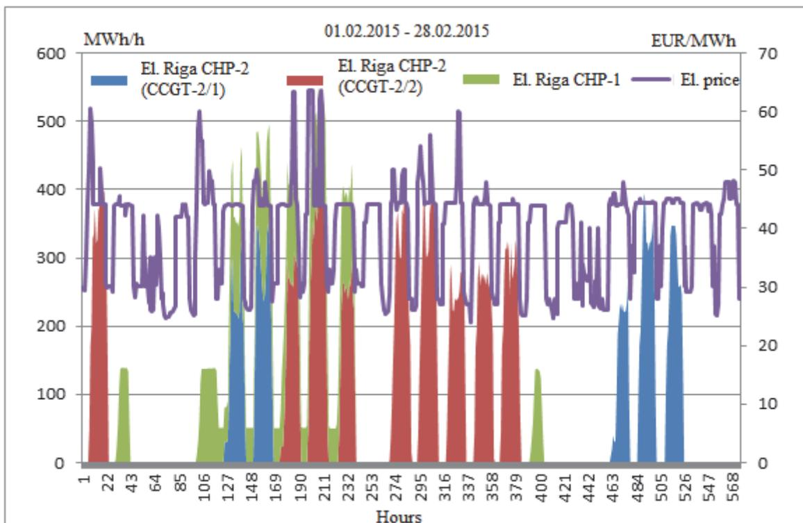
Fig. 13. Riga CHP operation in February 2013 (after joining NPS) (by the author according to production data of Riga CHP plants).
