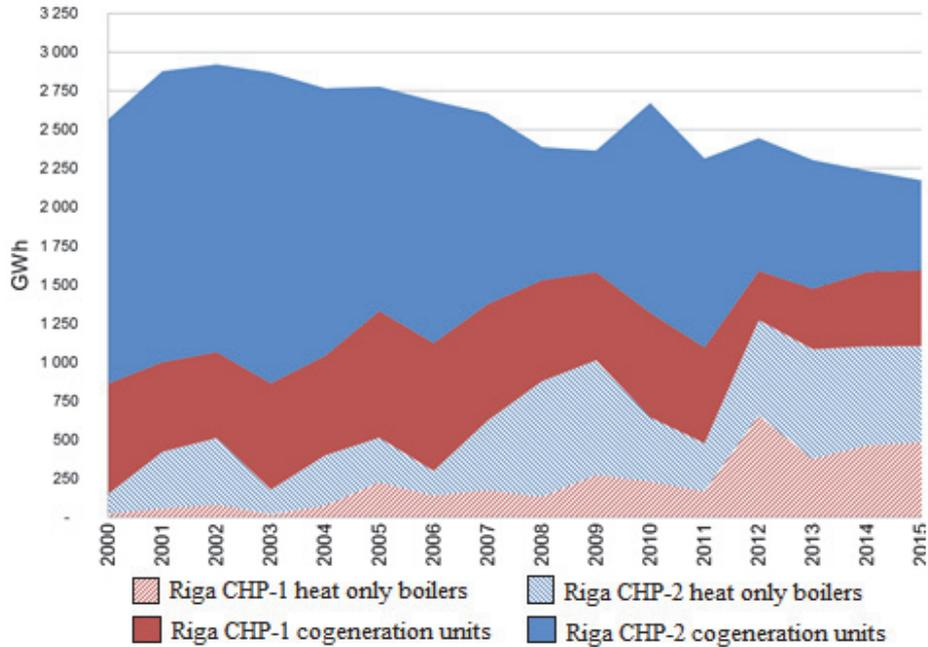
Fig. 3. Heat generation in Riga CHP (by the author; based on [2]).
