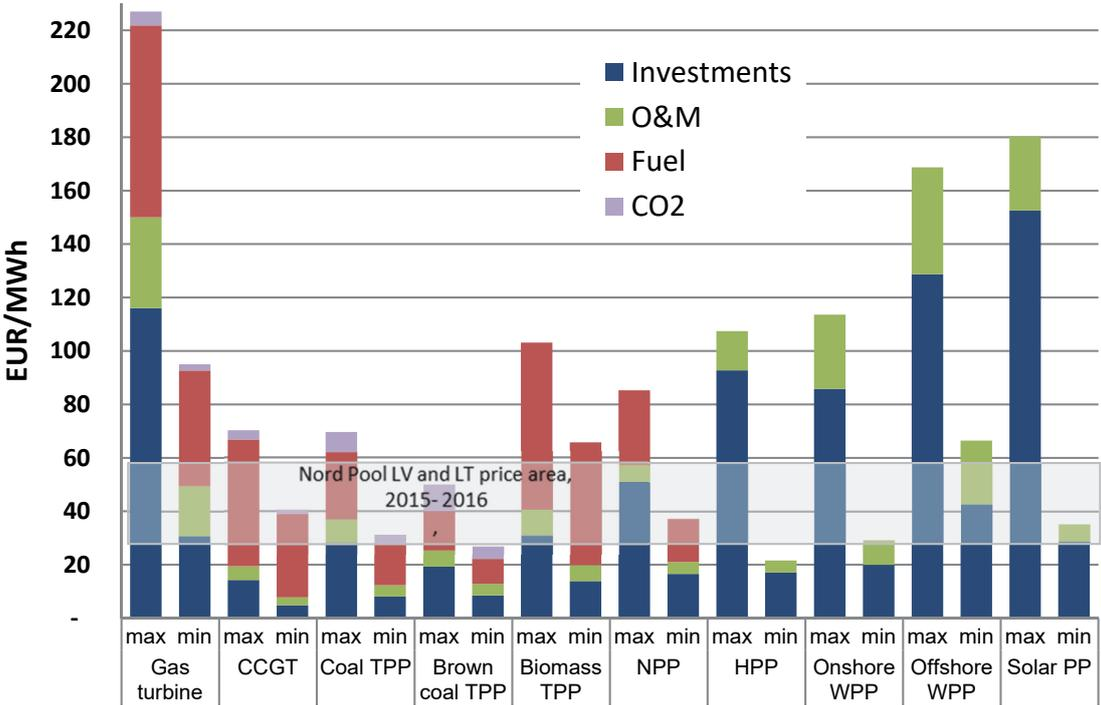
Fig. 6. Production costs for various technologies (optimum load) [4], [5].
