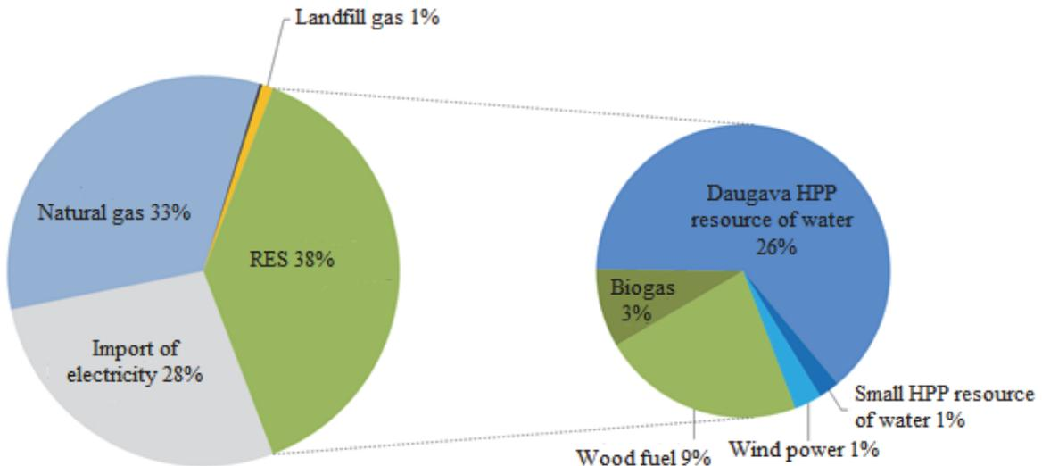
Fig. 4. Breakdown of the consumption of energy sources in 2014 in final consumption of electricity (6.58 TWh) [1].
