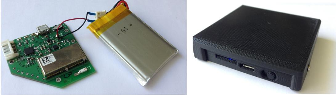
Figure 4.14. Master data acquisition module.
