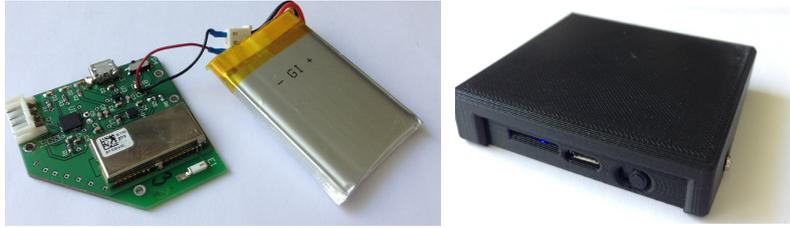
Figure 4.6. Master data acquisition module.
