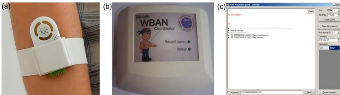
**Fig.5.1. MAS WBAN Experiment kit: (a) wireless perspiration sensor; (b) Coordinator Node (c) Application Layer.**
