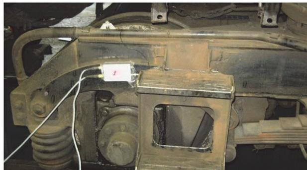
Fig. 2.8. Control sensors attachment on the bogie frame of the locomotive.
