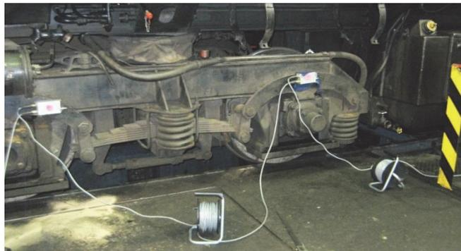
Fig. 2.7. The alignment of AE control system modules on the locomotive bogie frames.
