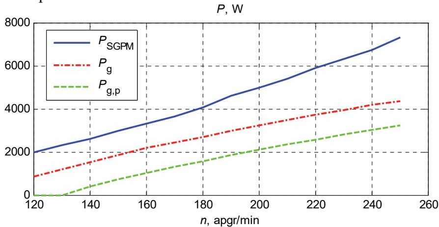
Figure 3.9. The rated power  $P_g$  of discussed self-excited generator and the available power  $P_{g,p}$  comparing with the PMSG rated power  $P_{SGPM}$
