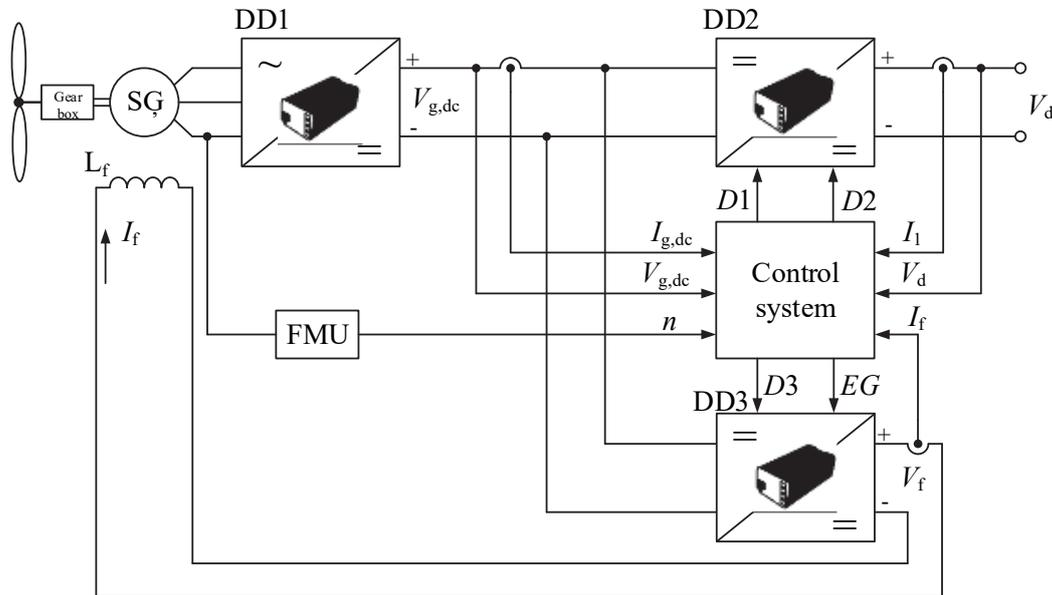
Figure 3.8. Self-excited SG and DC bus interconnection diagram: DD1 – uncontrolled built-in rectifier; DD2 – DC/DC converter; DD3 – SG self-excitation system; FMI – frequency measurement unit;  $D1$ – $D3$  – PWM outputs;  $EG$  – electronic generator control output;  $V_f$  – field (excitation voltage);  $I_f$  – excitation current;  $L_f$  – excitation winding
