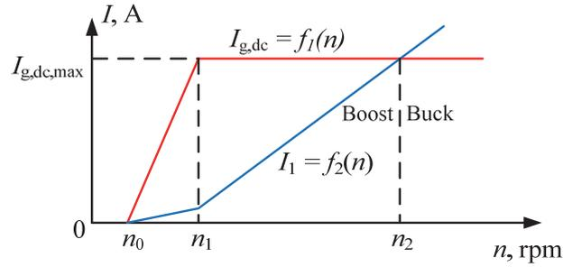
Figure 3.2. Wind turbine circuit current as function of generator speed
