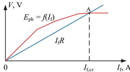
3.5. att. Generator phase EMF  $E_{ph}$  and voltage drop across the generator resistance:
