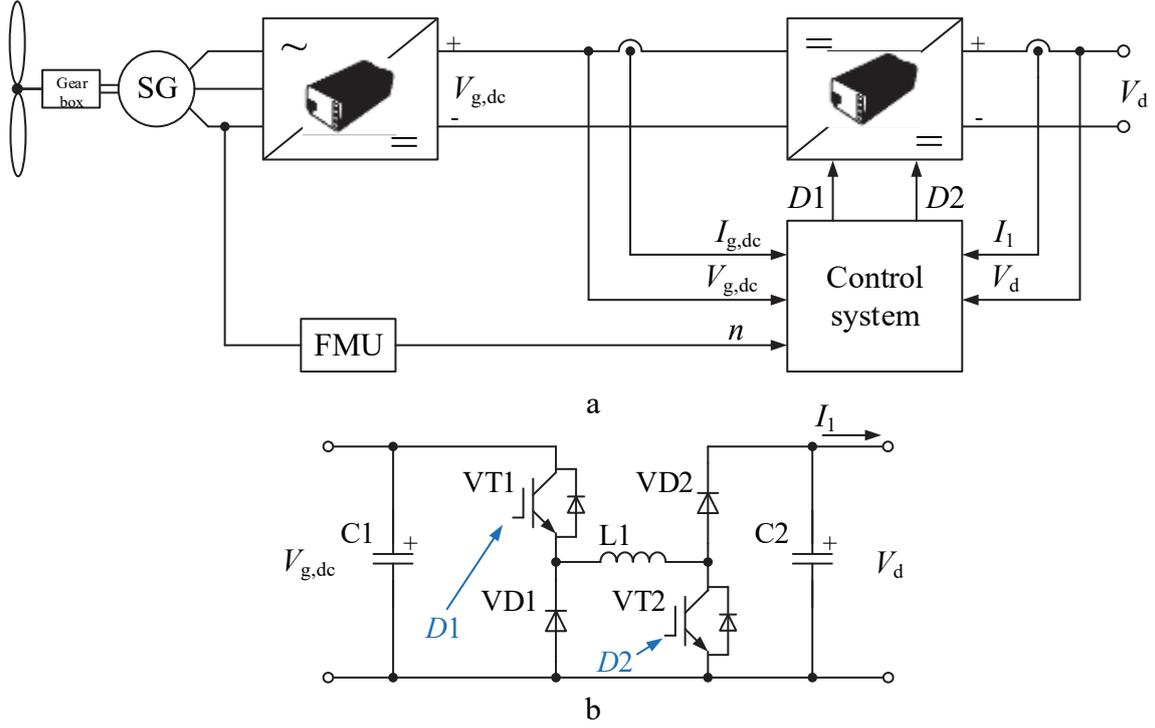
Figure 3.1. The block diagram of the proposed system (a) and the principal scheme of the DC/DC converter (b)
