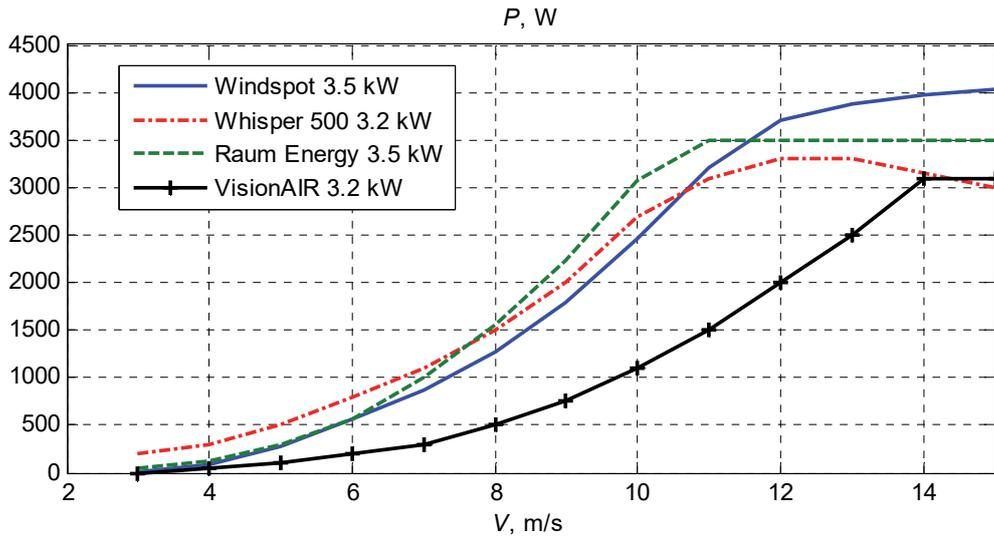
Figure 5.2. Power curves of some 3.2 kW and 3.5 kW wind turbines
