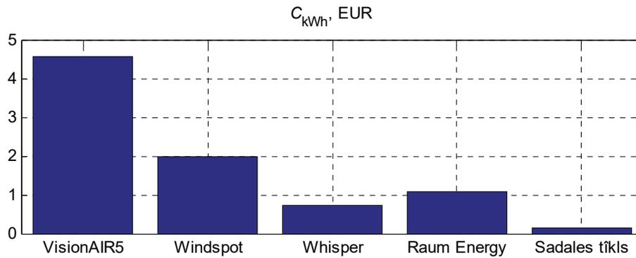
Figure 5.5. The difference between wind turbine produced energy price and price of the conventional grid (Sadales tīkls) energy
