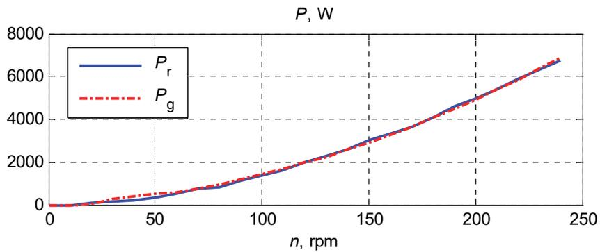
Figure 3.3. Wind generator GL-PMG-5000 rated ( $P_r$ ) and theoretically received ( $P_g$ ) power curves
