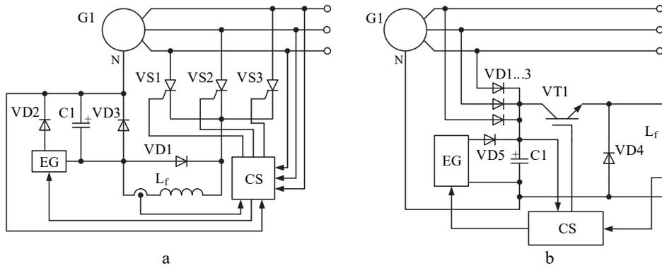
Figure 3.6. SG self-excitation system with the controlled half-bridge rectifier (a) and uncontrolled half-bridge rectifier with the step-down DC/DC converter (b): EG – electronic generator; CS – control system of the self-excitation device;  $L_f$  – excitation winding
