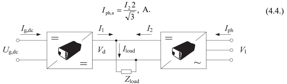
Figure 4.1. DC bus operation with the AC grid:  $U_{g,dc}$  – wind generator output DC voltage;  $V_d$  – DC bus voltage;  $V_1$  – AC grid line voltage;  $Z_{load}$  – load impedance;  $I_{g,dc}$  – wind generator output DC current;  $I_1$  – wind generator converter output current;  $I_{ph}$  – AC grid phase current;  $I_2$  – active rectifier output current;  $I_{load}$  – load current
