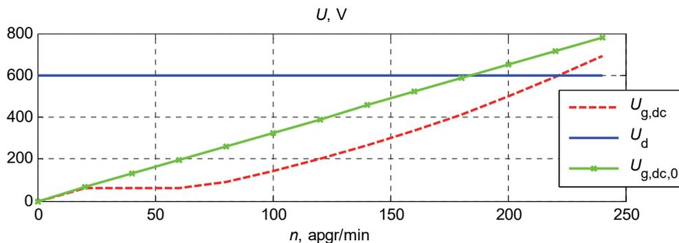
Figure 4.4. Simulation diagrams of the wind energy based DC microgrid connected to the conventional AC power grid:  $U_{g,dc}$  – wind generator output direct voltage;  $U_d$  – DC bus voltage;  $U_{g,dc,0}$  – wind generator output voltage in the idle
