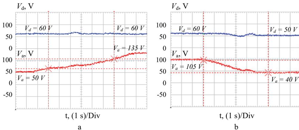
Figure 3.4. Operation of the DC/DC converter with DC load in case of increasing (a) and decreasing (b) of the converter input voltage:  $V_a$  – converter input voltage;  $V_d$  – DC bus voltage
