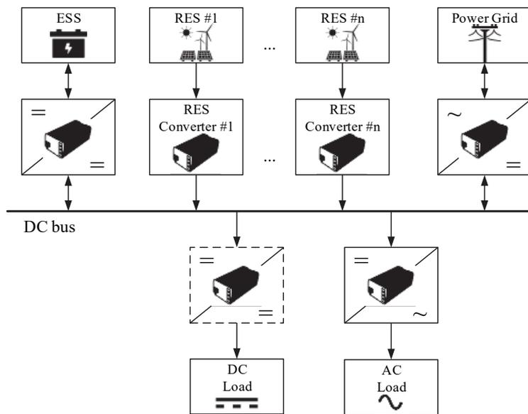
Figure 2.1. The block diagram of the DC based microgrid with the renewable energy sources [38]: ESS – energy storage system; RES – renewable energy source
