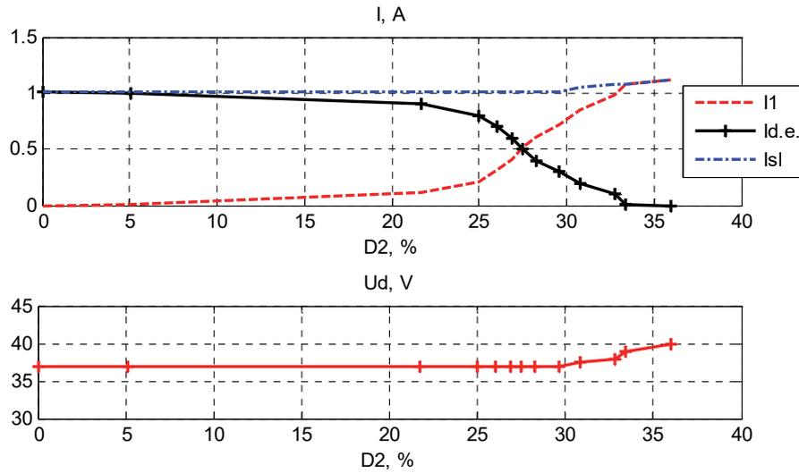
Figure 4.8. Currents and DC bus voltage  $U_d$  depending on the DC-DC converter duty ratio  $D_2$
