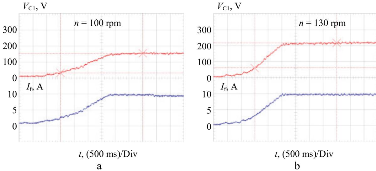
Figure 3.7. Experimental diagrams of the self-excitation process:  $V_{C1}$  – capacitor voltage;  $I_f$  – excitation current.
