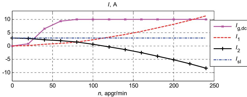
Figure 4.3. Simulation diagrams of the wind energy based DC microgrid connected to the conventional AC power grid:  $I_{g,dc}$  – wind generator output direct current;  $I_1$  – wind generator converter output current;  $I_2$  – active rectifier current;  $I_{sl}$  – load current
