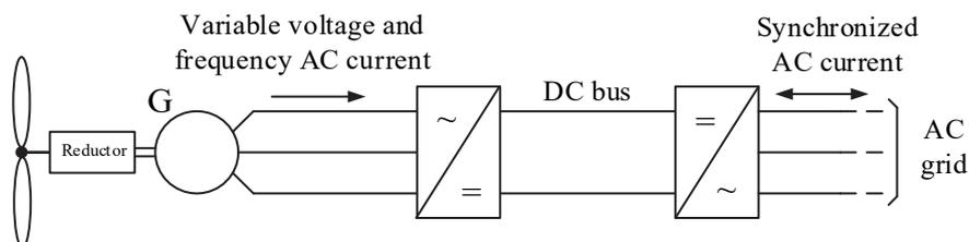
Figure 2.2. Wind turbine with permanent magnet synchronous generator
