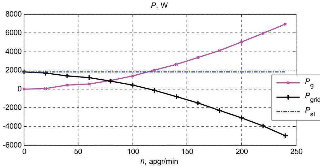
Figure 4.5. Simulation diagrams of the wind energy based DC microgrid connected to the conventional AC power grid:  $P_g$  – wind generator power;  $P_{s.t.}$  – conventional grid power;  $P_{sl}$  – load power
