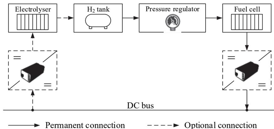
Figure 4.6. Connection of the hydrogen energy storage to the DC bus
