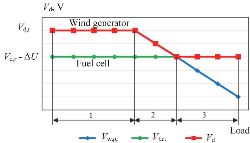
Figure 4.7. The voltage/load characteristics:  $V_{w.t.}$  – wind generator voltage;
