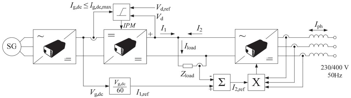
Figure 4.2. The calculation of the reference current of the active rectifier
