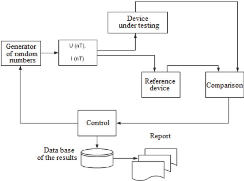
Fig. 1.5. Terminal testing supplying signals directly to the device under testing.
