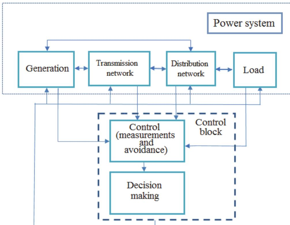
Fig. 1.4. Simplified structure of power system and its control.
