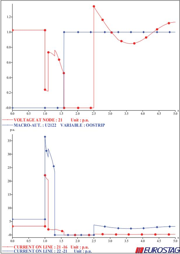
Fig. 4.4. Voltage of the power system in the unit <21> and currents of PEL 21-16 and 22-21.
