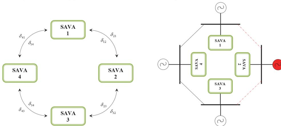
Fig. 3.11. and Fig. 3.12. SAVA round type principle scheme; electric station 2 operates in island regime.
