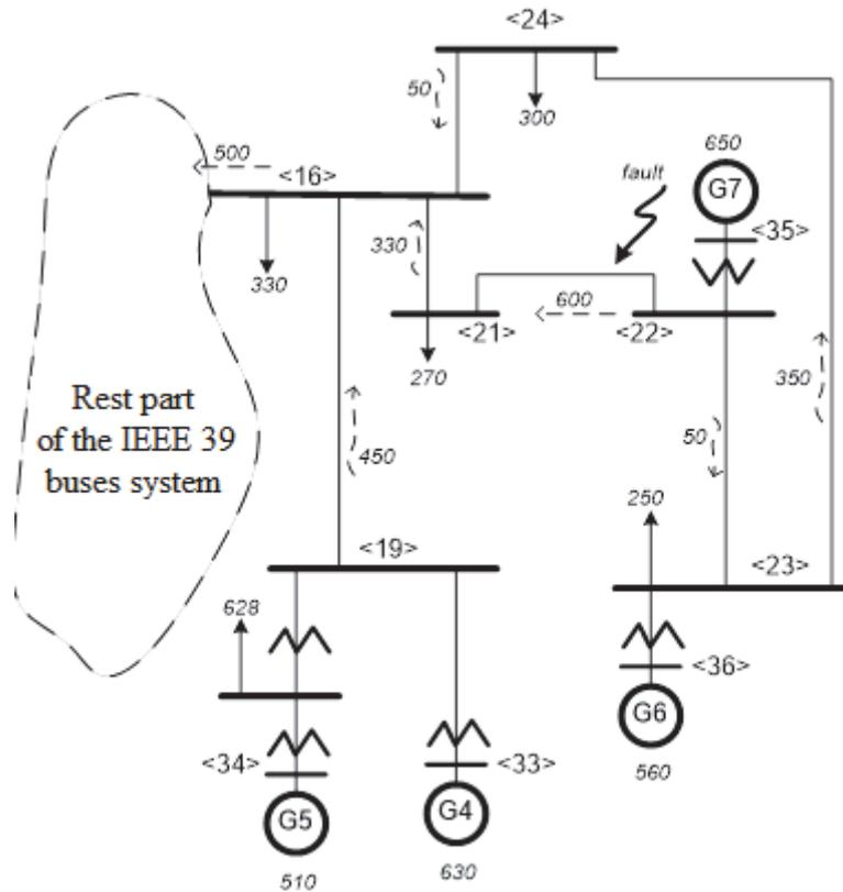
Fig. 4.1. Rest part of the IEEE 39 bus system for the testing scenario
