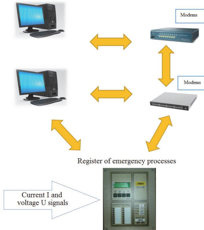
Fig. 2.2. Structure of the information exchange of the emergency processes register (EPR).
