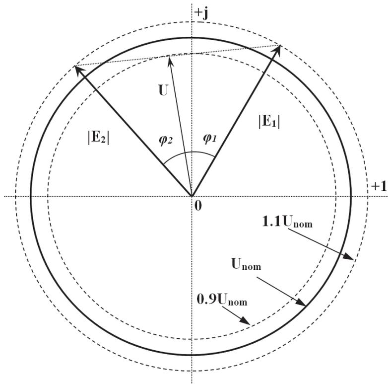
Fig. 3.6. Vector diagram of voltage and generator EMF in the complex plane.
