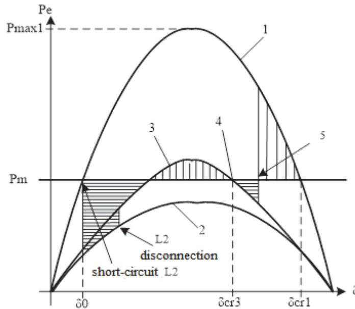
Fig. 3.7. Power-angle characteristics of generators:
