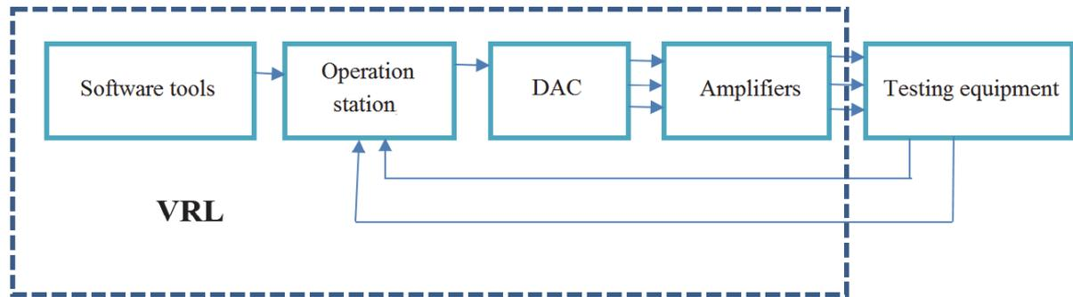
Fig. 1.2. Structure of virtual-real laboratory.
