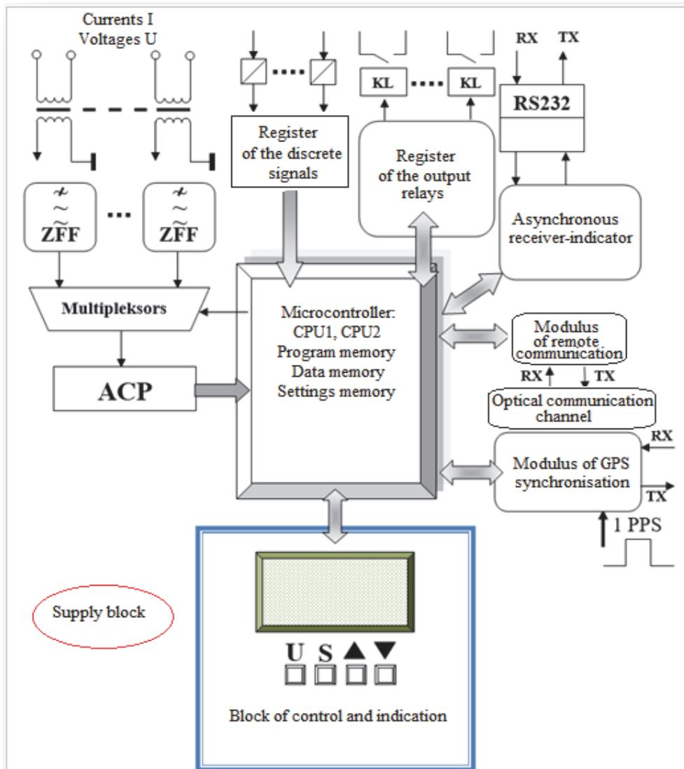
Fig. 2.4. Simplified structure of the device realisation.
