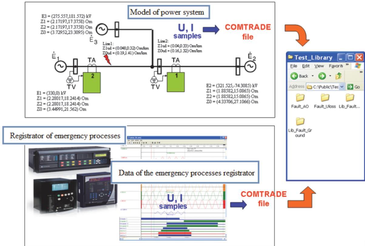
Fig. 4.6. Forming of the testing signal library.
