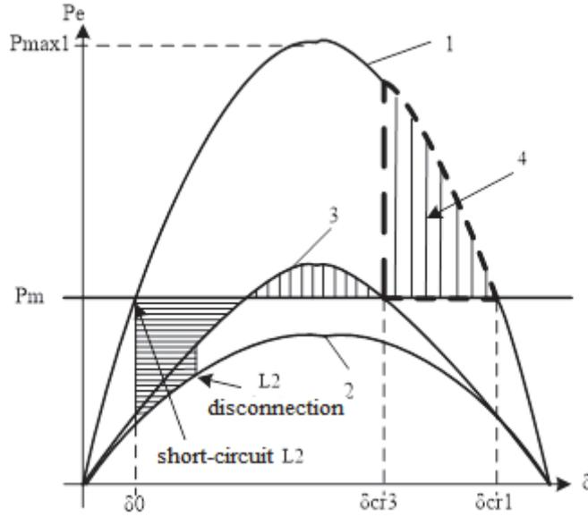
Fig. 3.8. Calculation example of proposed approach for theoretically possible braking square at time instant  $\delta_{cr3}$ :
