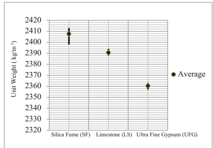
Fig. 3. Effect of mineral admixtures on unit weight.
