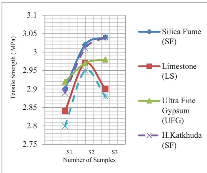
Fig. 9. Mineral admixture effect on concrete tensile strength.
