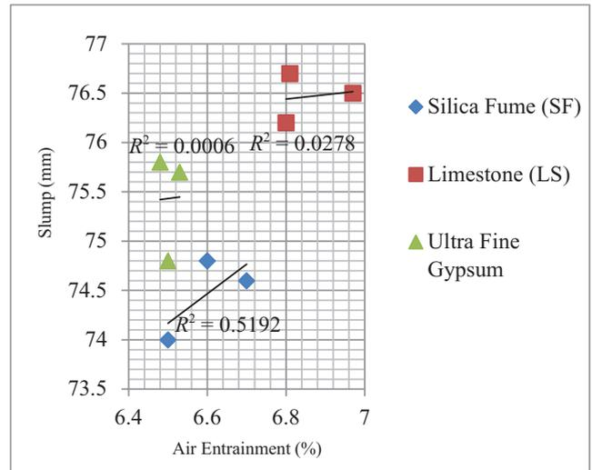
Fig. 6. Correlation between air entrainment and workability.
