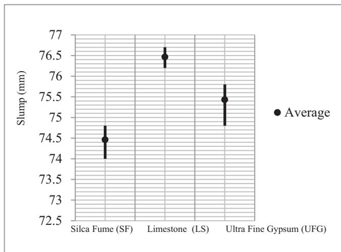
Fig. 2. Effect of mineral admixtures on workability.
