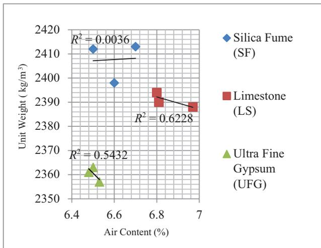
Fig. 5. Correlation between air entrainment and unit weight.
