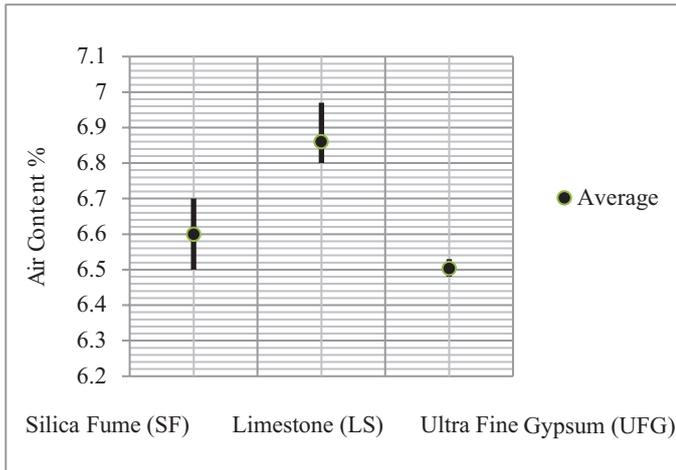
Fig. 4. Effect of mineral admixtures on air entrainment.
