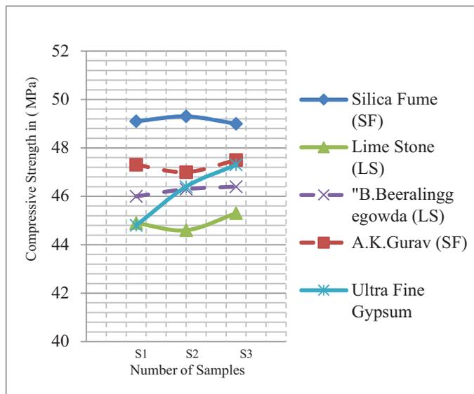
Fig. 8. Mineral admixture effect on concrete compressive strength.
