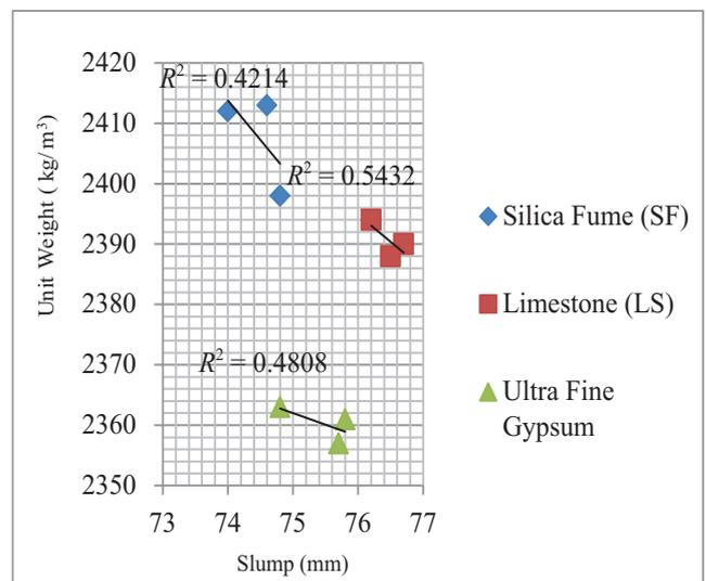
Fig. 7. Correlation between workability and unit weight.
