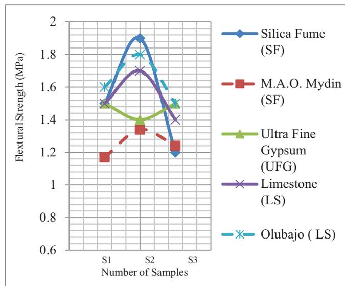
Fig. 10. Mineral admixture effect on concrete flexural strength.
