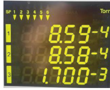
Fig. 2.4. Ionization vacuum gauge HPG 400 pressure measurement without argon correction.
