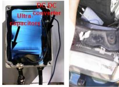
Fig. 4.3. Prototype of modernization device for starting ICE.
