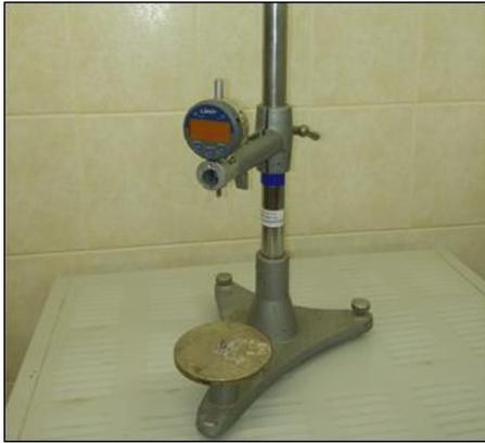
Fig. 1. Digital dial indicator and frame.
