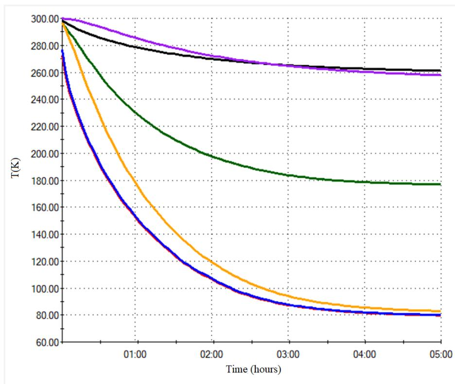
Fig. 4.9. Cooling curves for cryostat (Fig. 4.8.) components.
