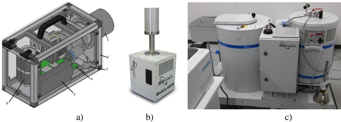
Fig. 6.1. a) portable gamma spectrometer *HandSPEC*; b) *Monolith* laboratory gamma spectrometer; c) *Nicole* gamma spectrometer with hybrid cooling.
