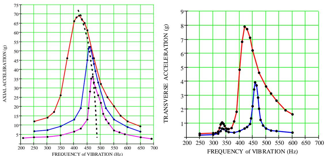
Fig. 5.3. Dependency of the vibration acceleration of the detector unit in the axial (vertical) (left) and transverse (horizontal) (right) direction of the frequency if there is a constant amplitude of the base vibration acceleration: 9g – red line; 4g – blue line; 2g – pink line.
