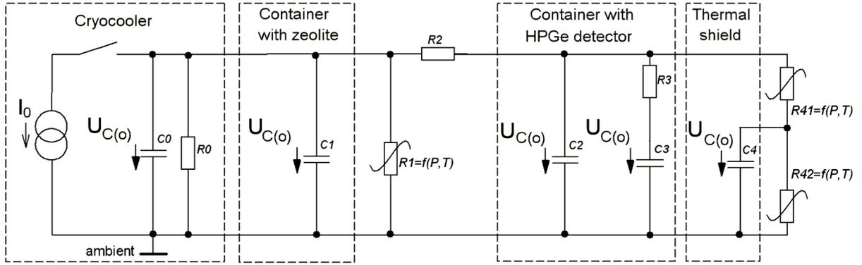
Fig. 4.2. Equivalent thermoelectric model for cryostat with EMC and thermal shield for cooling process analysis.
