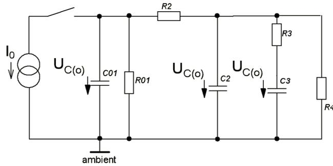
Fig. 4.3. Linearized equivalent cryostat with EMC model.
