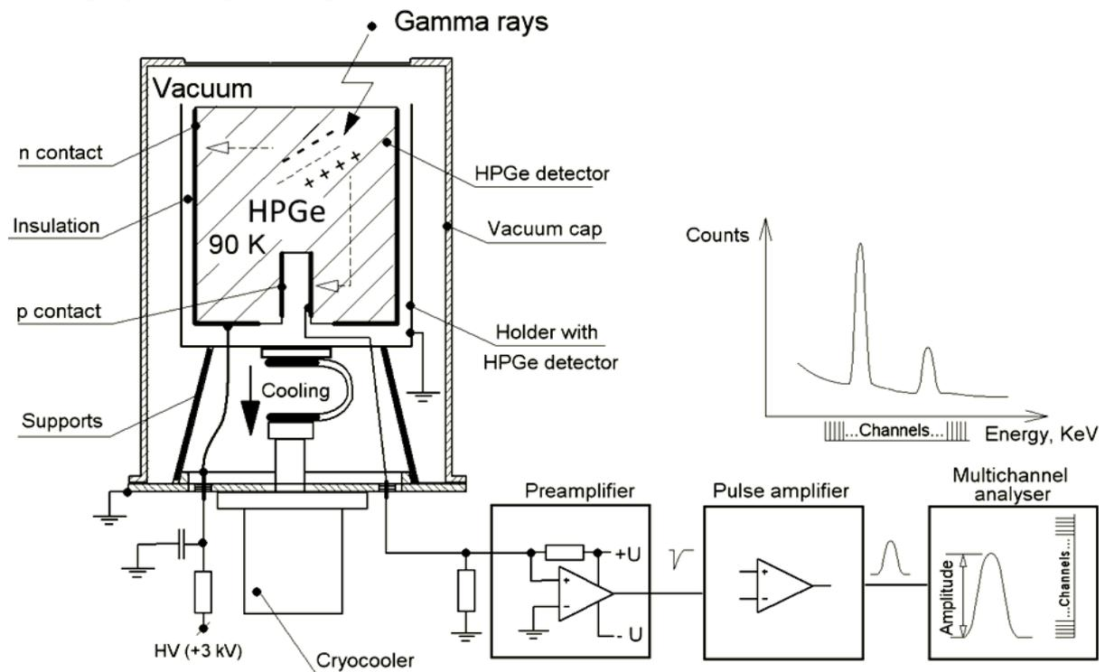
Fig. 1.1. Gamma spectrometer structure based on HPGe detectors.
